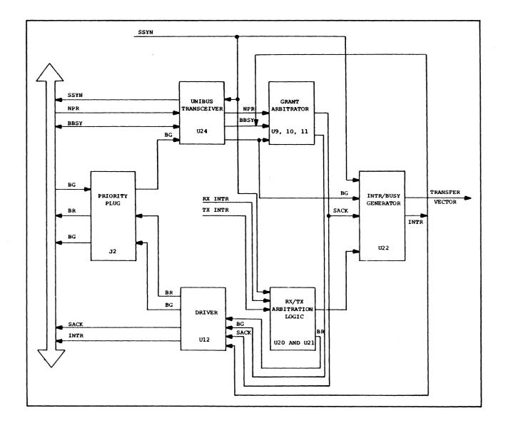
FIGURE 4-3: INTERRUPT LOGIC BLOCK DIAGRAM
