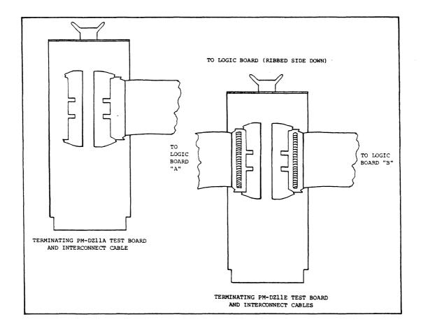
FIGURE 1-7: PM-H3271 TEST CONNECTOR (P/N 701792-100X2)
