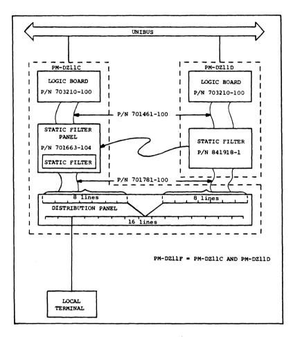
FIGURE 1-4: CURRENT LOOP MODEL HARDWARE
