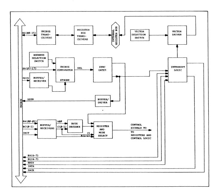
FIGURE 4-2: UNIBUS INTERFACE LOGIC BLOCK DIAGRAM
