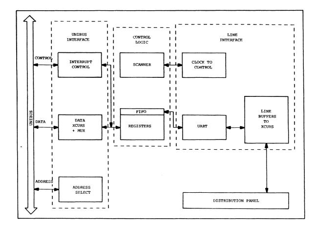
FIGURE 1-9: GENERAL FUNCTIONAL BLOCK DIAGRAM
