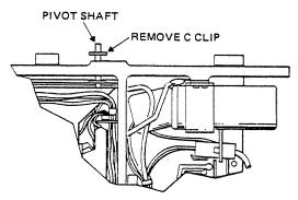
FIGURE 7 CARTRIDGE GUIDE REMOVAL
