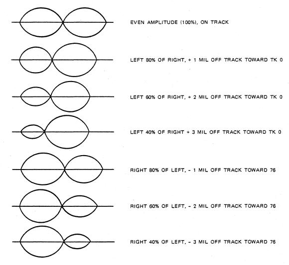
Figure 11 R/W Head Radial Alignment
