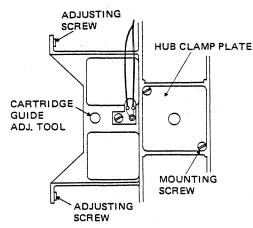
FIGURE 6 CARTRIDGE GUIDE ADJUSTMENT
