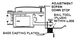
FIGURE 3 HEAD LOAD ACTUATOR DOWN STOP ADJUSTMENT
