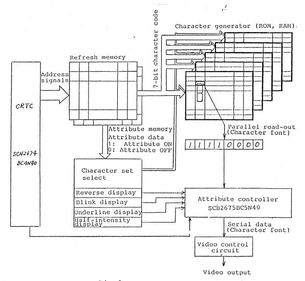
Fig. 5-4-2 Display Data Generation Processes
