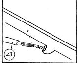
Fold back the keyboard cable toward the parts mounting surface of the board. Take care so as not to put the cable between the case and the board at assembly.
