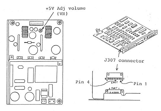
Fig. 7-1-1 +5V Power Supply Voltage Adjustment
