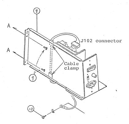
Fig. 6-1-3 Removal of Power Bracket
