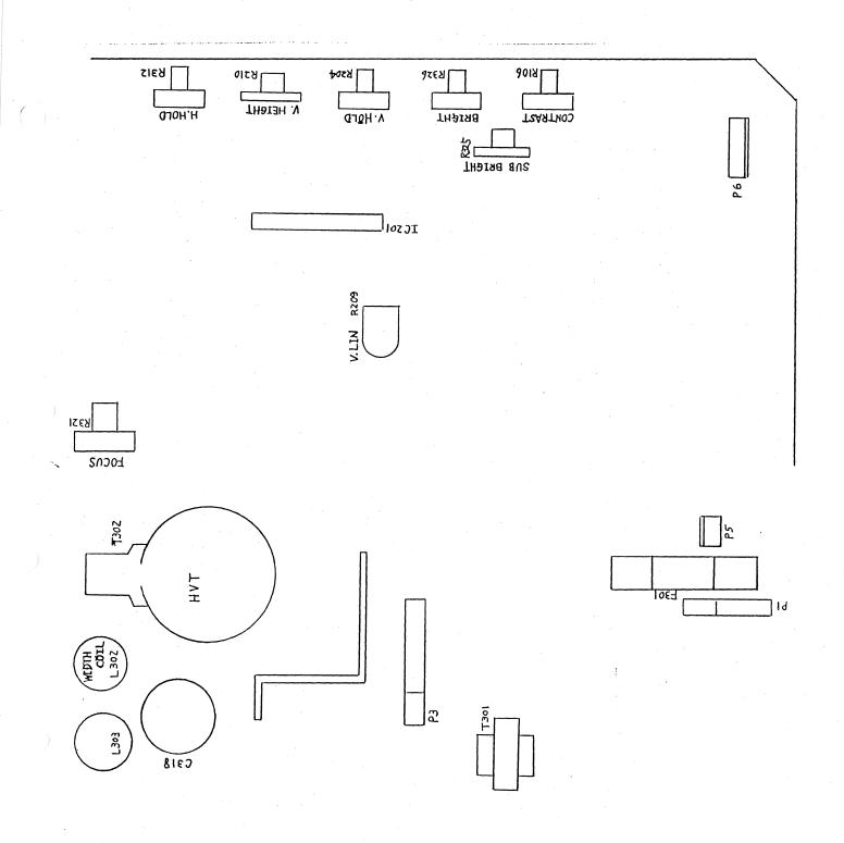
Fig. 7-1-3 Monitor Adjustment Points
