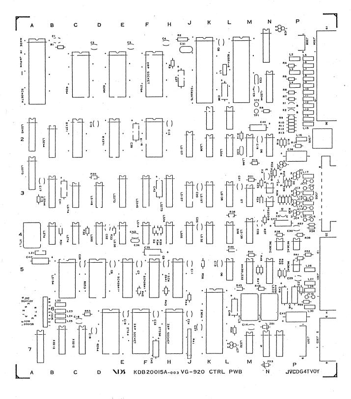
Fig. 12-1-1 Logic PWB Parts Mounting Diagram
