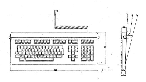
Fig. 4-2-2 Keyboard Unit Dimensions Diagram
