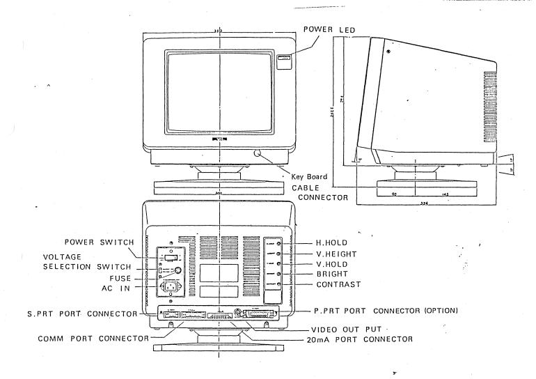
Fig. 4-2-1 Display Unit Dimensions Diagram
