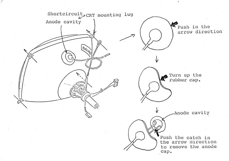
Fig. 6-1-4 Removal of Anode Cap
