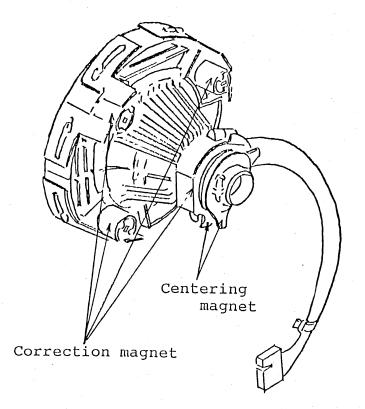
Fig. 7-1-2 Monitor Adjustment Points
