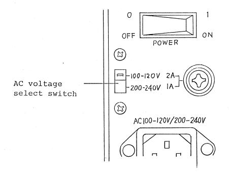
Be sure to check that the AC voltage Select switch is set as shown below when the power supply voltage is 100 to 120 V:
