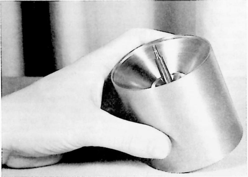
Fig. 4-7. Magnetic drum memory—capable of holding 100,000 bits of information on its surface.
