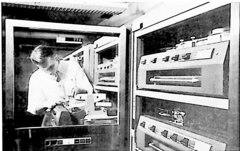
Fig. 4-2. Paper tape, an input method still being used, is being headed through a reader punch unit.
