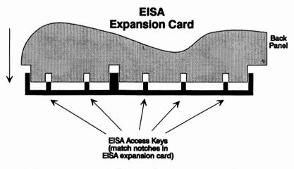
FIGURE 2-9 EISA Board Connector Notching
