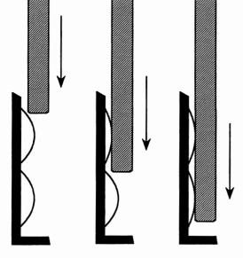
FIGURE 2-7 EISA Connector Finger Contacts
