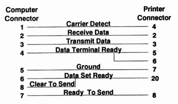
FIGURE 8-4 Wiring of a Typical Printer 9- to 25-pin RS232 Cable
