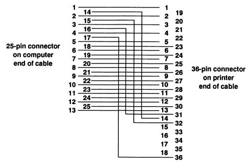
FIGURE 9-3 Typical Parallel Printer Cable Wiring
