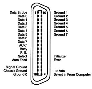
FIGURE 9-2 Typical Centronics Connector Pin Numbering
