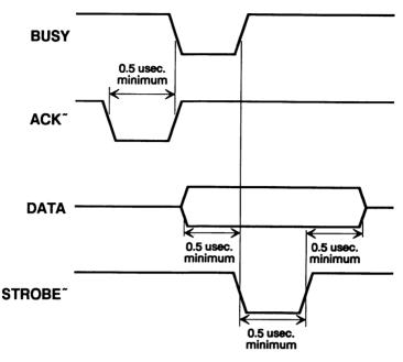
FIGURE 9-4 Typical Parallel Connector Timing
