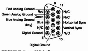
FIGURE 7-1 VGA Connector Pinout
