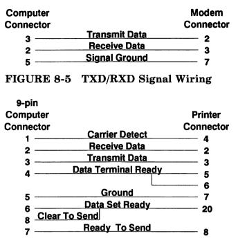
FIGURE 8-6 Null Modem Cable Wiring
