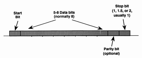
FIGURE 8-9 Serial Data Stream Format
