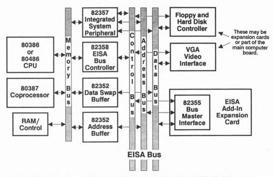
FIGURE 2-13 Typical EISA Computer Simplified Block Diagram
