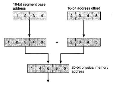
Figure 2-1. Intel 8086 address calculation.
