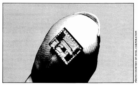
FIGURE 1-2. A microprocessor chip
