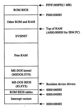
Figure 2-6. SYSINIT and MSDOS.SYS relocated.
