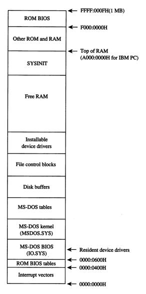
Figure 2-7. Tables allocated and installable device drivers loaded.
