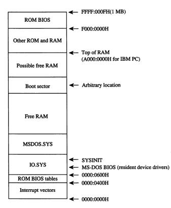
Figure 2-5. IO.SYS and MSDOS.SYS loaded.
