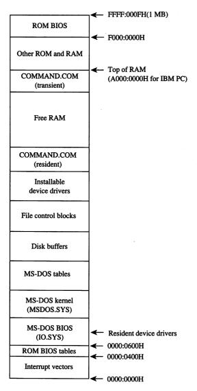
Figure 2-9. COMMAND.COM after relocation.
