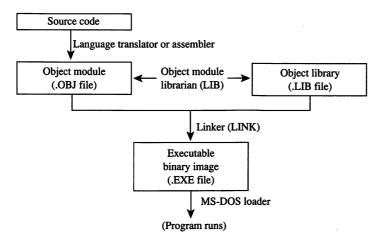
Figure 19-1. Generation of an executable (.EXE) file.
