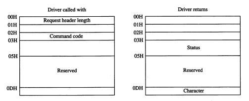
Figure 15-8. The Nondestructive Read request header.
