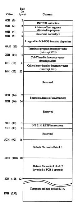
Figure H-1 (memory block diagram) illustrates the structure of the program segment prefix (PSP).
