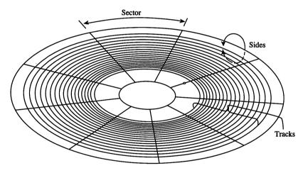
Figure 3-1. The physical layout of a CAV 9-sector, 5.25-inch floppy disk.
