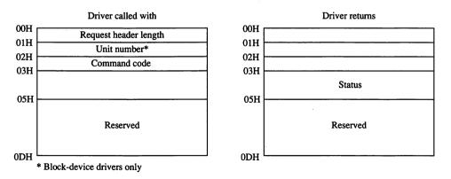
Figure 15-10. The request header for Device Open (command code 13), Device Close (command code 14), and Removable Media (command code 15).
