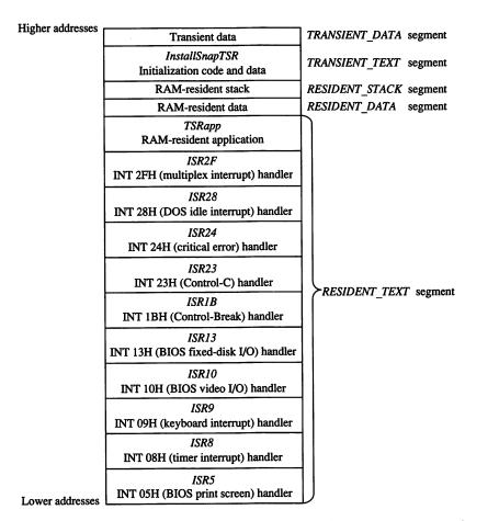
Figure 11-5. Block structure of the TSR program SNAP.EXE when loaded into memory. (Compare with Figure 11-1.)
