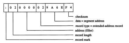
Figure L-1. The extended-address record.
