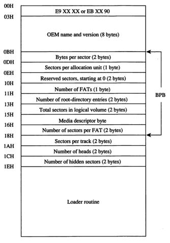
Figure 3-6. Map of the boot sector of an MS-DOS disk. Bytes OBH through 17H are the BIOS parameter block (BPB).
