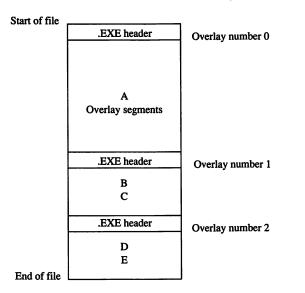
Figure 20-14. .EXE file structure produced by LINK A + (B+C) + (D+E).
