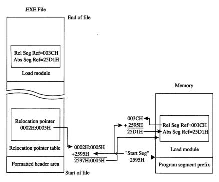
Figure 4-6. The .EXE file relocation procedure.
