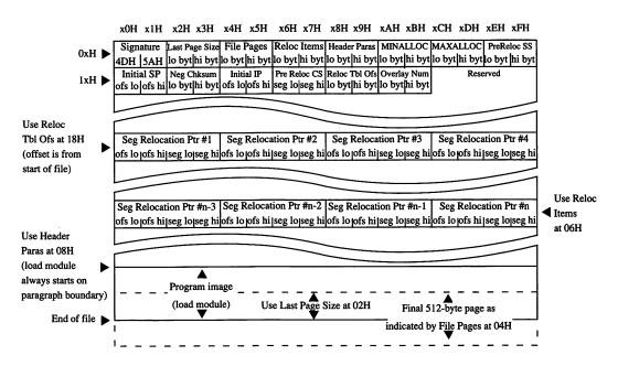
Figure 4-5. Structure of a .EXE file.
