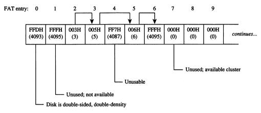
Figure 3-8. Space allocation in the FAT for a typical MS-DOS disk.
