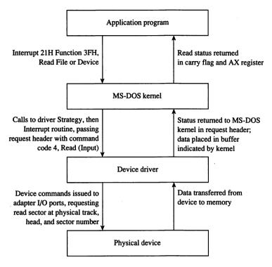
Figure 15-13. The processing of a typical I/O request from an application program.
