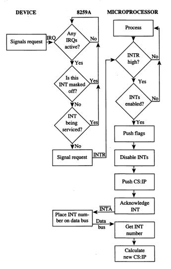
Figure 13-2. Maskable interrupt service.
