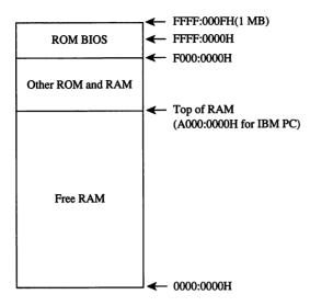
Figure 2-1. Memory layout at startup.
