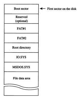
Figure 2-4. Boot-disk configuration.
