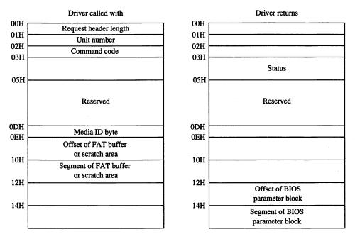
Figure 15-6. Build BPB request header (command code 2).
