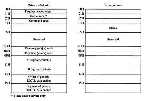
Figure 15-11. Generic IOCTL request header.
