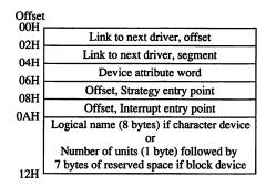
Figure 15-2. Device header. The offsets to the Strat and Intr routines are offsets from the same segment used to point to the device header.
