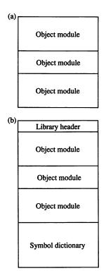
Figure 20-2. Structures of an object file and an object library. (a) An object file contains one or more object modules. (Microsoft discourages using more than one object module per object file.) (b) An object library contains one or more object modules plus a hashed symbol dictionary indicating the object modules in which each public symbol is defined.
