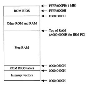
Figure 2-2. The interrupt vector table and the ROM BIOS table.
