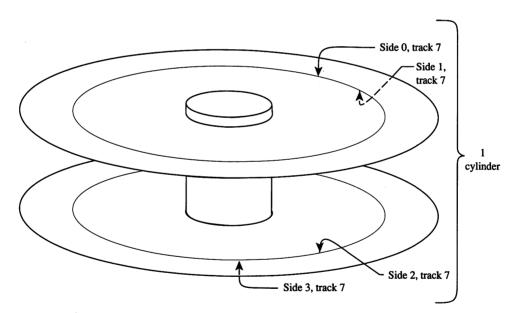
Figure 3-2. Tracks and cylinders on a fixed-disk system.
