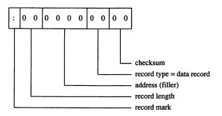
Figure L-5. The alternate end-of-file record.
