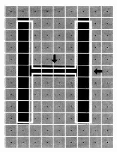
Figure 3-4: With hinting, the font rasterizer knows how to "move" the outline so the strokes are better aligned with the pixel grid; this turns on exactly one pixel for each of the three strokes in the letter.
