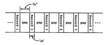
(a) Magnetic tape with 1600-character/inch storage density, showing storage of unblocked 200-character records. Each input operation reads one physical record and thus one logical record
