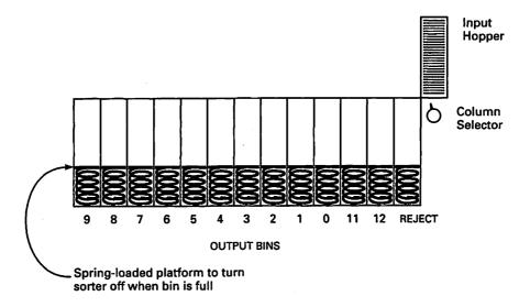
Figure 14.14 Electromechanical Punched-Card Sorter
