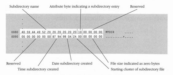
**Figure 10-7.** Extract from the root directory of an MS-DOS disk, showing the entry for a subdirectory named MYDIR. Bit 4 in the attribute byte is set, the cluster field points to the first cluster of the subdirectory file, the date and time stamps are valid, but the file length is zero.
