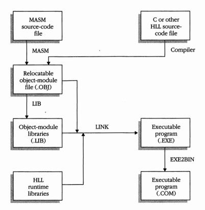
Figure 4-8. Creation of an MS-DOS application program, from source code to executable file.
