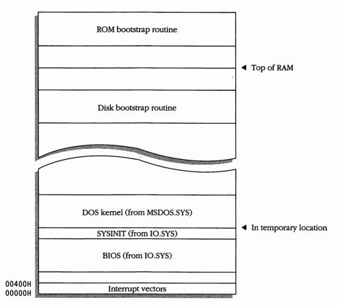
**Figure 2-3.** The disk bootstrap reads the file IO.SYS into memory. This file contains the MS-DOS BIOS (resident device drivers) and the SYSINIT module. Either the disk bootstrap or the BIOS (depending upon the manufacturer's implementation) then reads the DOS kernel into memory from the MSDOS.SYS file.
