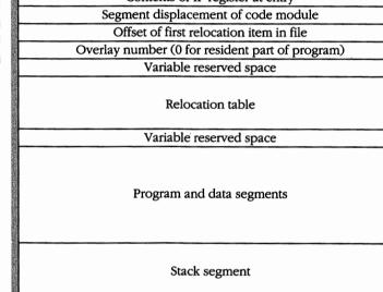
Figure 3-5. The format of a .EXE load module.
