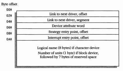
Figure 14-2. Device-driver header. The offsets to the strat and intr routines are offsets from the same segment used to point to the device header.
