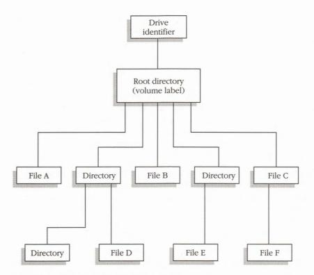
Figure 9-1. An MS-DOS file-system structure.
