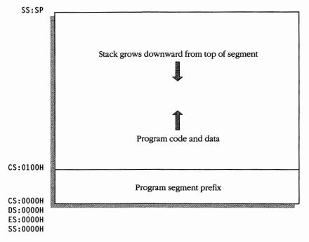
**Figure 3-2.** A memory image of a typical .COM-type program after loading. The contents of the .COM file are brought into memory just above the program segment prefix. Program, code, and data are mixed together in the same segment, and all segment registers contain the same value.
