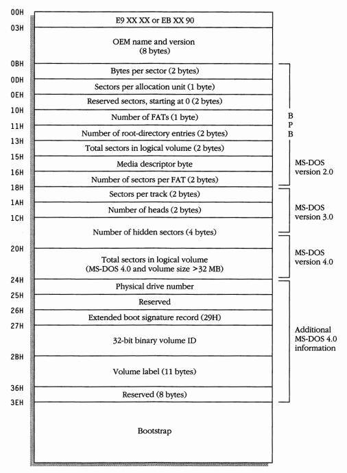
**Figure 10-2.** Map of the boot sector of an MS-DOS disk. Note the JMP at offset 0, the OEM identification field, the MS-DOS version 2 compatible BIOS parameter block (bytes OBH–17H), the three additional WORD fields for MS-DOS version 3, the double-word number-of-sectors field and 32-bit binary volume ID for MS-DOS version 4.0, and the bootstrap code.
