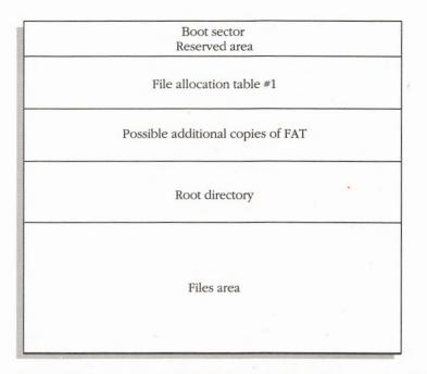
**Figure 10-1.** Map of a typical MS-DOS logical volume. The boot sector (logical sector 0) contains the OEM identification, BIOS parameter block (BPB), and disk bootstrap. The remaining sectors are divided among an optional reserved area, one or more copies of the file allocation table, the root directory, and the files area.
