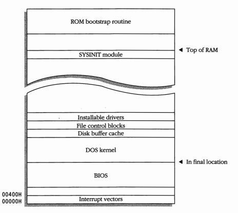
**Figure 2-4.** SYSINIT moves itself to high memory and relocates the DOS kernel, MSDOS.SYS, downward to its final address. The MS-DOS disk buffer cache and file control block areas are allocated, and then the installable device drivers specified in the CONFIG.SYS file are loaded and linked into the system.
