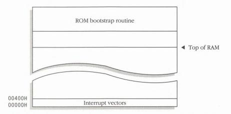
**Figure 2-1.** A typical 8086/8088-based computer system immediately after system startup or reset. Execution begins at location OFFFOH, which contains a jump instruction that directs program control to the ROM bootstrap routine.
