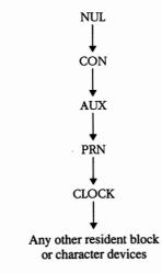
**Figure 14-10.** *MS-DOS device-driver chain before any installable device drivers have been loaded.*
