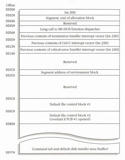
Figure 3-1. The structure of the program segment prefix.
