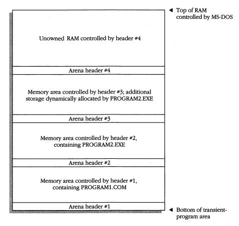
**Figure 11-3.** An example diagram of MS-DOS arena headers and the transientprogram area. The environment blocks and their associated headers have been omitted from this figure to increase its clarity.
