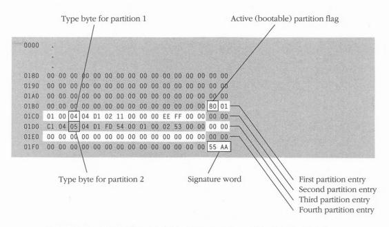
**Figure 10-11.** A partial hex dump of a master block from a fixed disk formatted under PC-DOS version 3.3. This disk contains two partitions. The first partition has a 16-bit FAT and is marked "active" to indicate that it contains a bootable copy of PC-DOS. The second partition is an "extended" partition. The third and fourth partition entries are not used in this example. **Chapter 11**
