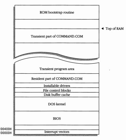
**Figure 2-5.** The final result of the MS-DOS startup process for a typical system. The resident portion of COMMAND.COM lies in low memory, above the DOS kernel. The transient portion containing the batch-file interpreter and intrinsic commands is placed in high memory, where it can be overlaid by extrinsic commands and application programs running in the transient program area.
