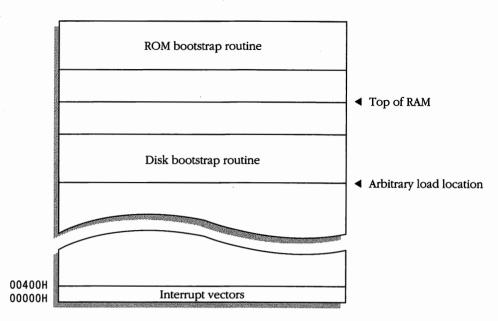
**Figure 2-2.** The ROM bootstrap routine loads the disk bootstrap routine into memory from the first sector of the system startup disk and then transfers control to it.
