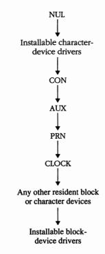
Figure 14-11. MS-DOS device-driver chain after installable device drivers have been loaded.
