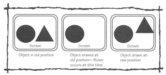
Figure 30.1 Drawing Directly to the Screen
