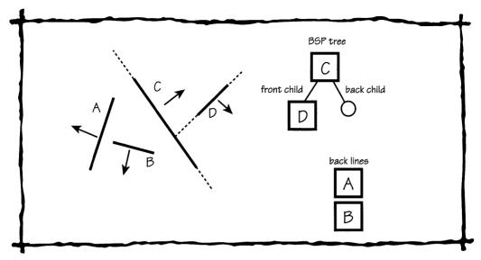
Figure 44.4 Split of wall C's front subspace along the line of wall D.
