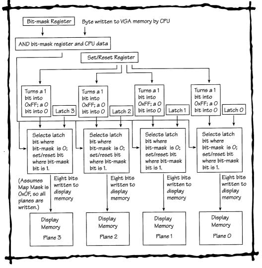
Figure 40.3 The Data Path in Write Mode 3
