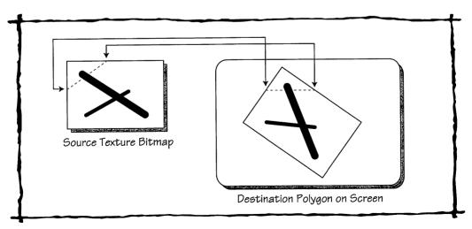
Figure 43.1 Texture Mapping a Single Horizontal Scanline
