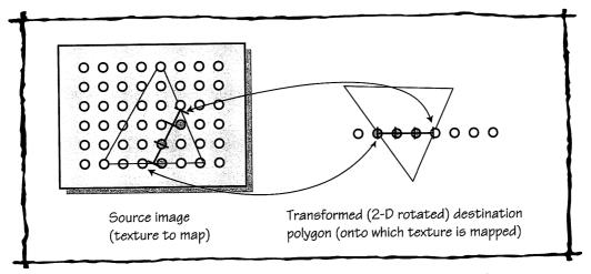
Figure 41.4 Mapping a Horizontal Destination Scan Line Back to the Source Image
