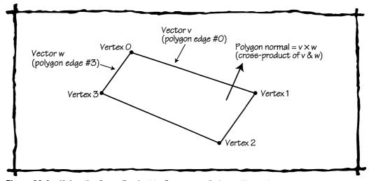
Figure 36.2 Using the Cross Product to Generate a Polygon Normal
