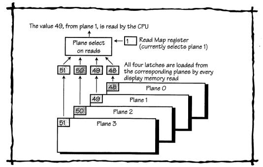
Figure 33.1 How the VGA Latches Are Loaded
