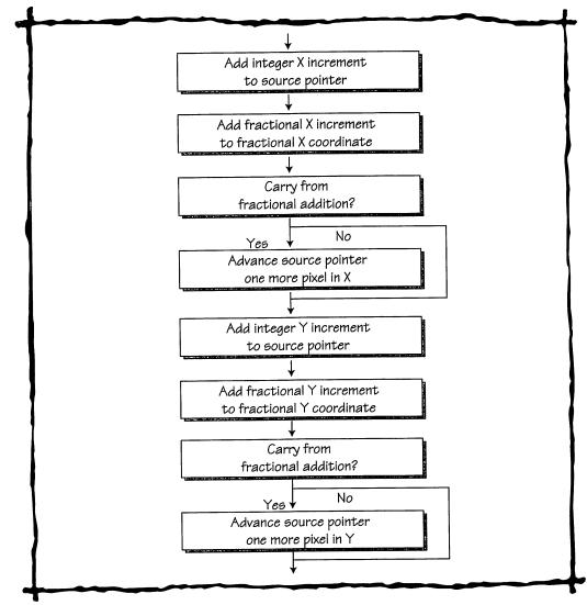
Figure 43.4 Original Method for Advancing the Source Texture Pointer
