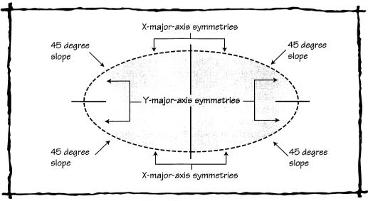
Figure 19.2 The Symmetry of Non-Tilted Ellipses
