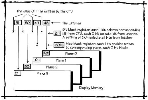
Figure 33.2 Writing 4 Bytes to Display Memory in a Single Operation
