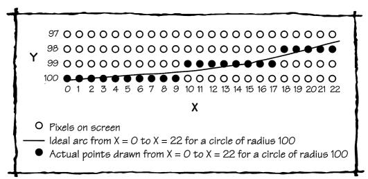
Figure 17.2 Incremental Arc Drawing
