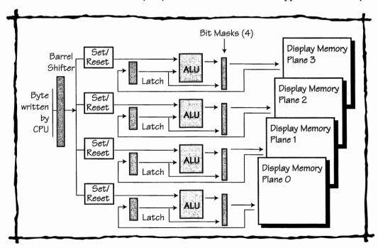
Figure 3.3 Data Flow During a Write Mode 0 Write Operation
