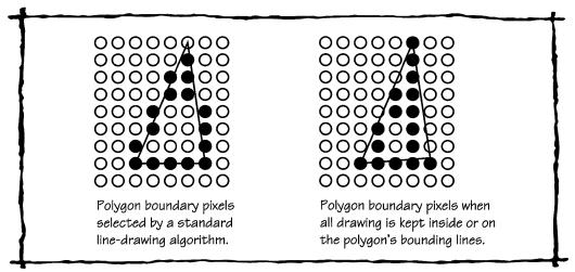
Figure 21.2 Drawing Polygons with Standard Line-Drawing Algorithms
