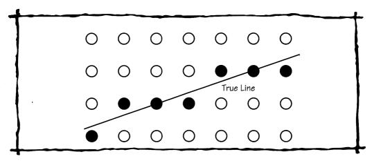
Figure 14.1 Approximating a True Line from a Pixel Array
