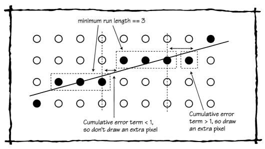
Figure 15.4 How the Error Term Determines Run Length
