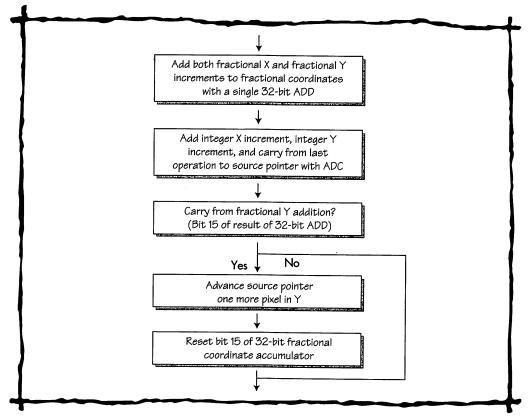
Figure 43.7 Final Method for Advancing Source Texture Pointer
