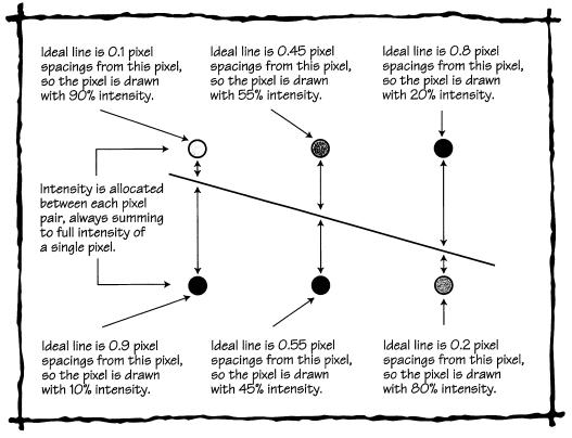
Figure 27.1 The Basic Concept of Wu Antialiasing
