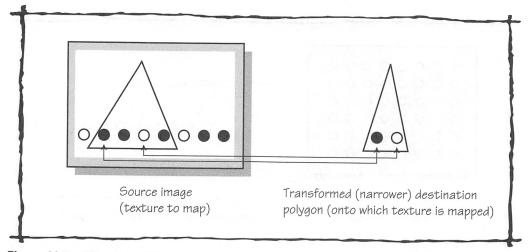
Figure 41.5 Mapping a Texture onto a Narrower Polygon
