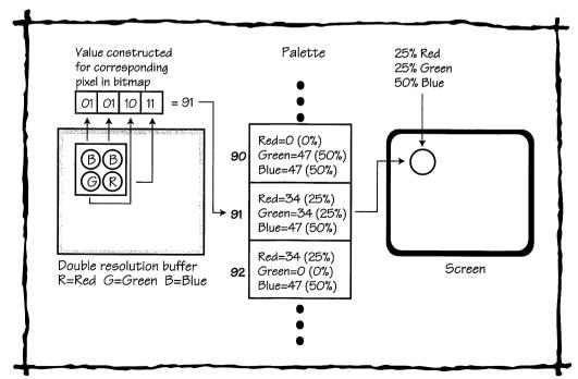
Figure 25.2 From the Double-Resolution Buffer to the Screen
