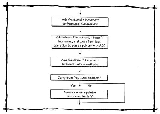
Figure 43.5 Efficient Method for Advancing Source Texture Pointer
