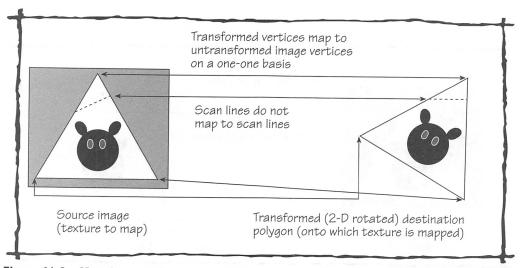
Figure 41.3 Mapping a Texture onto a 2-D Rotated Polygon
