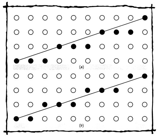
Figure 15.5 Balancing Run-Length Slice Lines: a) Unbalanced; b) Balanced
