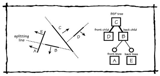
Figure 44.5 Split of wall C's back subspace along the line of wall B.
