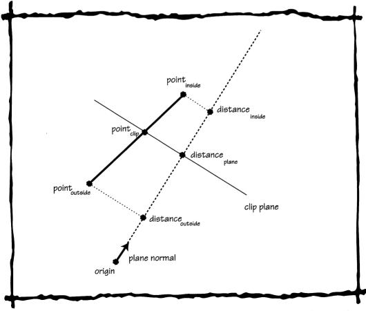
Figure 49.1 The distance from the plane to the inside endpoint, measured along the normal.
