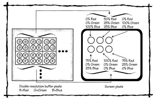
Figure 25.1 Mapping Double-Resolution Pixels to Single Screen Pixels
