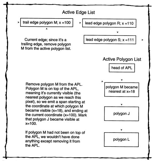
Figure 50.4 Deactivating a polygon when a trailing edge is encountered in the AEL.
