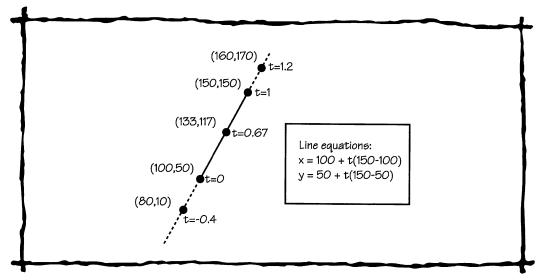
Figure 45.1 A sample parametric line.
