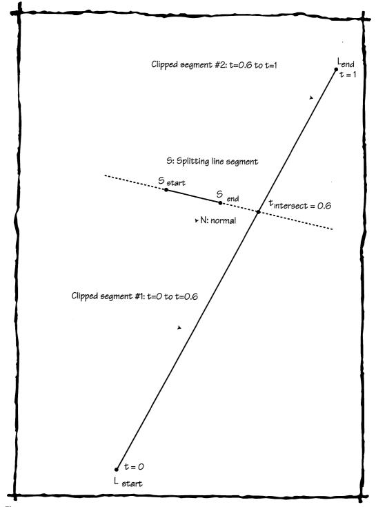
Figure 45.3 How line intersection is calculated.
