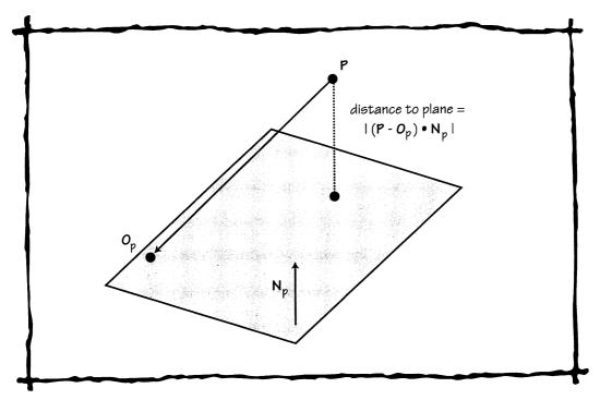
Figure 46.7 Using the dot product to get the distance from a point to a plane.
