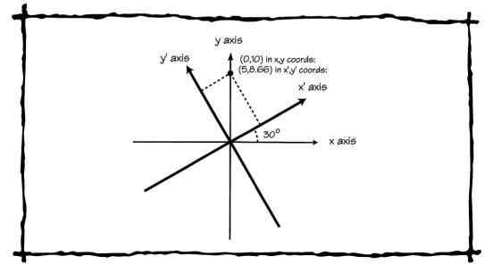
Figure 46.8 Rotation to a new coordinate space by projection onto new axes.
