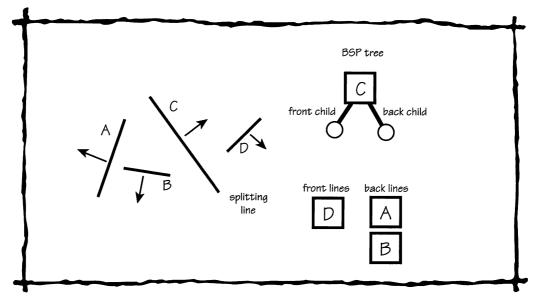
Figure 44.3 Initial split along the line of wall C.
