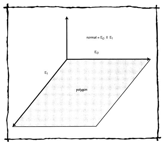
Figure 46.4 How the cross product of polygon edge vectors generates a polygon normal.
