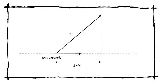
Figure 46.6 How the dot product with a unit vector performs a projection.
