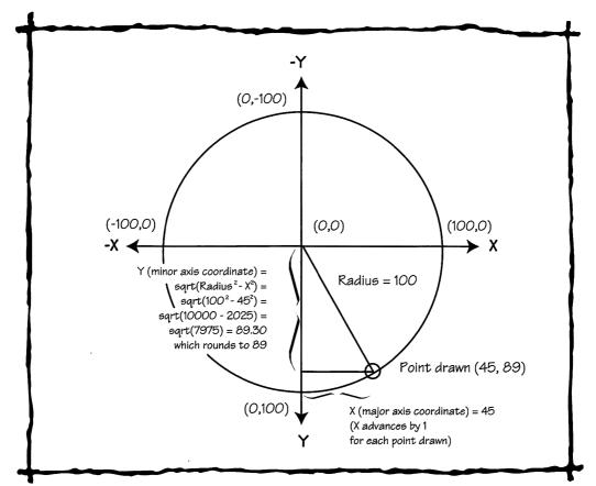
Figure 17.1 Calculating the Arc
