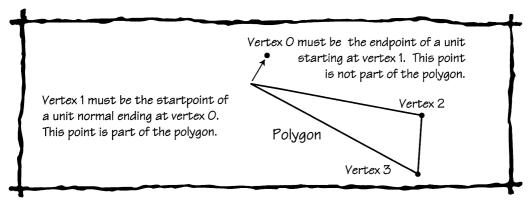
Figure 39.3 The Unit Normal in the Polygon Data Structure
