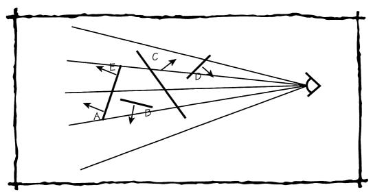
Figure 44.7 Viewing the BSP tree from an arbitrary angle.
