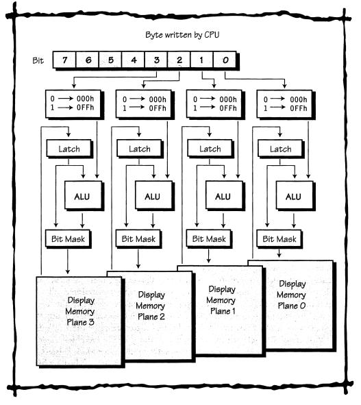
Figure 5.1 VGA Data Flow in Write Mode 2
