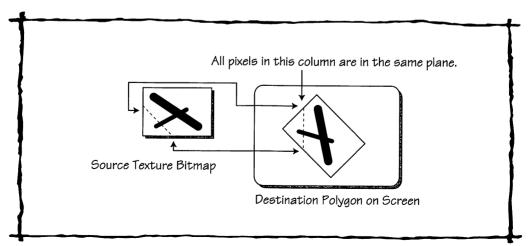
Figure 43.3 Texture Mapping a Single Vertical Column
