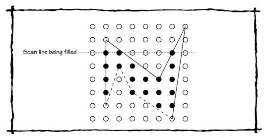
Figure 23.2 Checking Currently Active Edges (Solid Lines)
