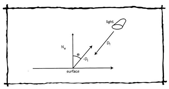
Figure 46.2 The dot product as used in calculating lighting intensity.
