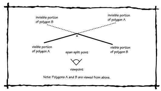
Figure 51.1 Intersecting span sorting.
