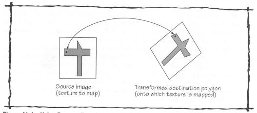
Figure 41.1 Using Reverse Transformation to Find the Source Pixel Color
