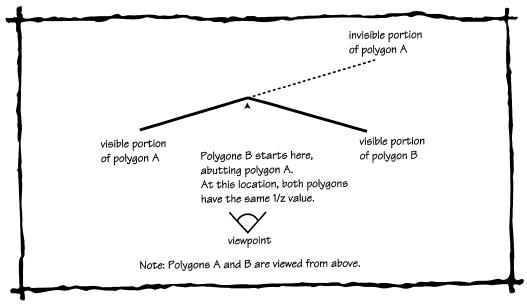
Figure 51.2 Abutting span sorting.
