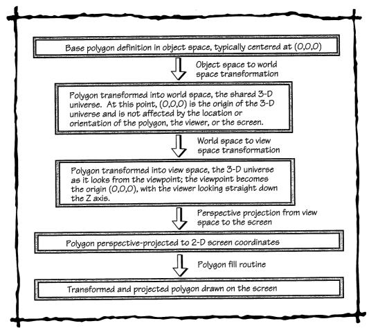
Figure 35.1 The 3-D Drawing Pipeline
