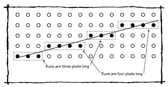
Figure 15.3 Runs in a Slope 1/3.5 Line
