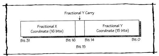
Figure 43.6 Storing Both X and Y Fractional Coordinates in One Register
