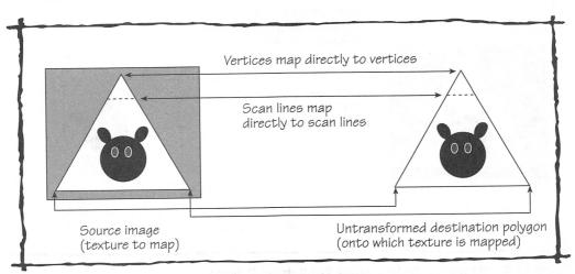
Figure 41.2 Mapping a Texture onto an Untransformed Polygon
