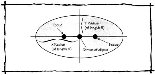
Figure 19.1 The Geometry of an Ellipse
