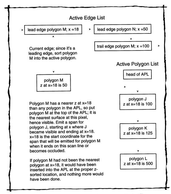
Figure 50.3 Activating a polygon when a leading edge is encountered in the AEL.
