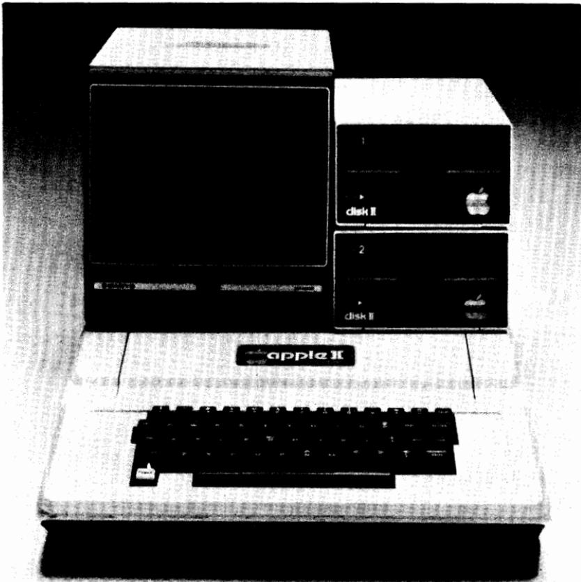
The Apple II computer. Here is a personal computer system with keyboard and CRT. The computer is in the foreground cabinet with the keyboard. The display screen is a standard TV set. The top of the computer cabinet lifts off, giving access to the plug-in components. *Photo courtesy of Apple Computers*
