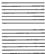
(B) Interrupted Scan equals one horizontal line—slight vertical "bump."
