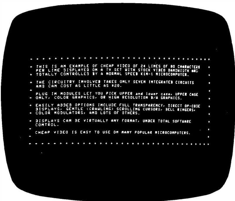
Fig. 1-4. Typical alphanumeric cheap video display.
