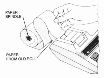
3. Use this step to install paper when a piece of paper is NOT remaining in the printer.
