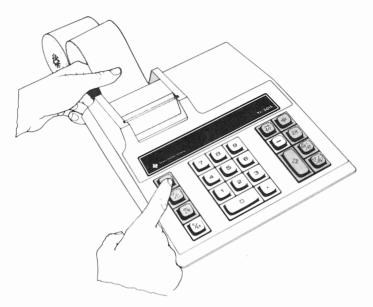
4. Place the new roll of paper back into the paper cradle to complete paper installation.
