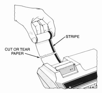
Place the new roll of paper behind the calculator so that the paper unrolls from the bottom of the spindle. If there is paper remaining in the printer, use this step to install paper and skip step 3. Otherwise, proceed with step 3.
