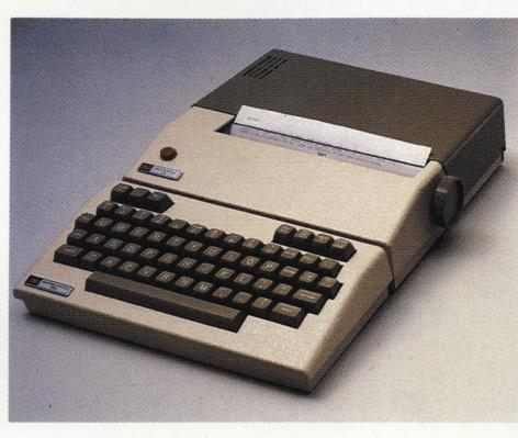
Package 83 is designed to communicate with destinations on either Telex I or International Telex networks using F1/F2 analog lines. The optional, field-installable IRC Telex kit allows connection to IRC Telex lines. It consists of a Model 1483 teleprinter and a Model 1446 Intelligent Keyboard.
