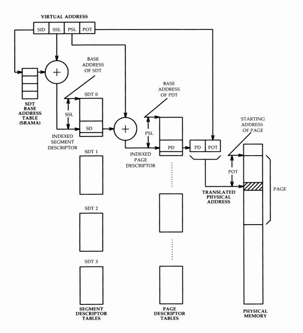
Figure 3-31: Virtual Address to Physical Address Translation for Paged Segments
