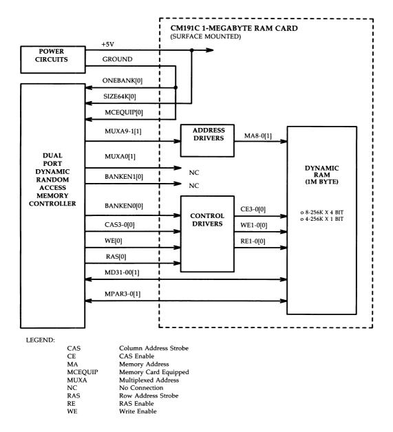
Figure 3-41: CM191C 1-Megabyte, Surface Mounted, RAM Card — Functional Block Diagram
