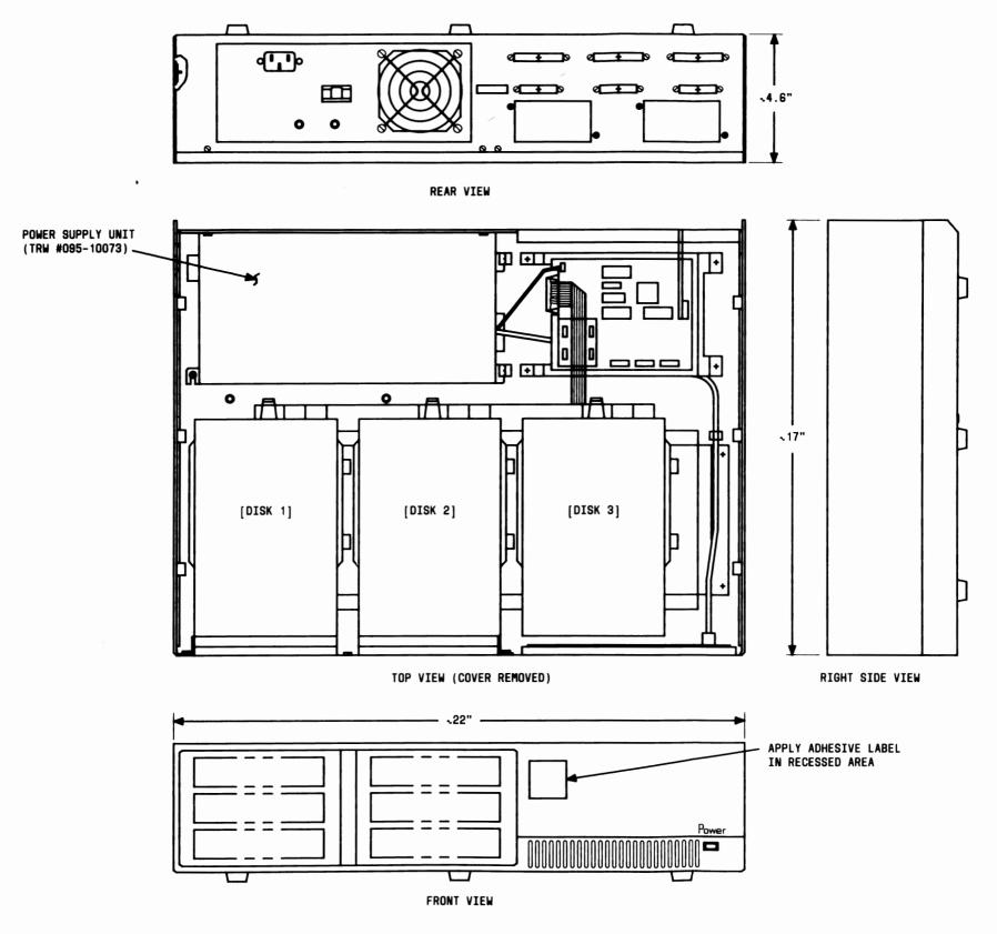
Figure 2-14: International AT&T XM/405S/900S Cabinet Assembly Drawing (ED-3T027-30)
