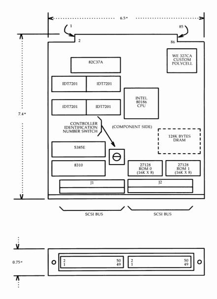
Figure 2-56: CM195W SCSI Host Adapter Card Layout
