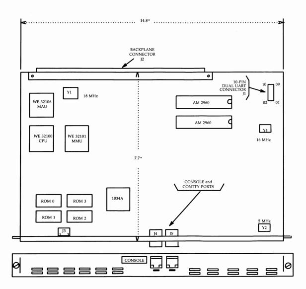
Figure 2-25: CM518A System Board Layout
