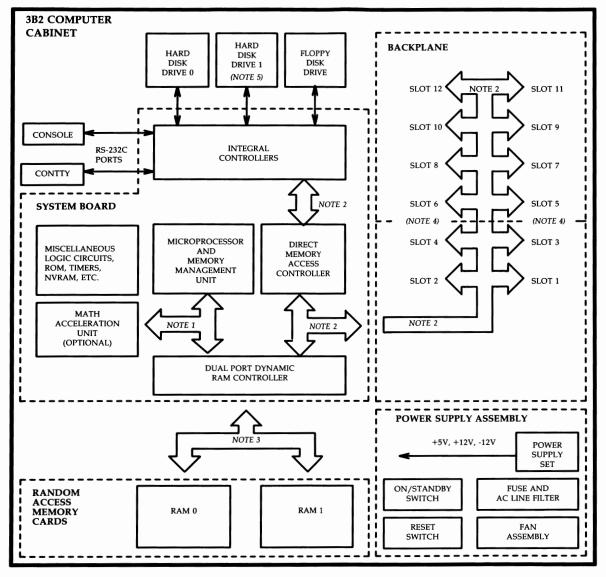
1. 32-BIT ADDRESS BUS AND 32-BIT DATA BUS.
