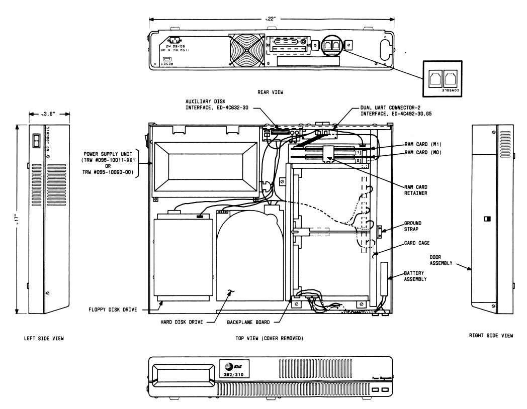
Figure 2-3: Domestic 3B2/310 Computer Cabinet Assembly Drawing (ED-4C645-30)
