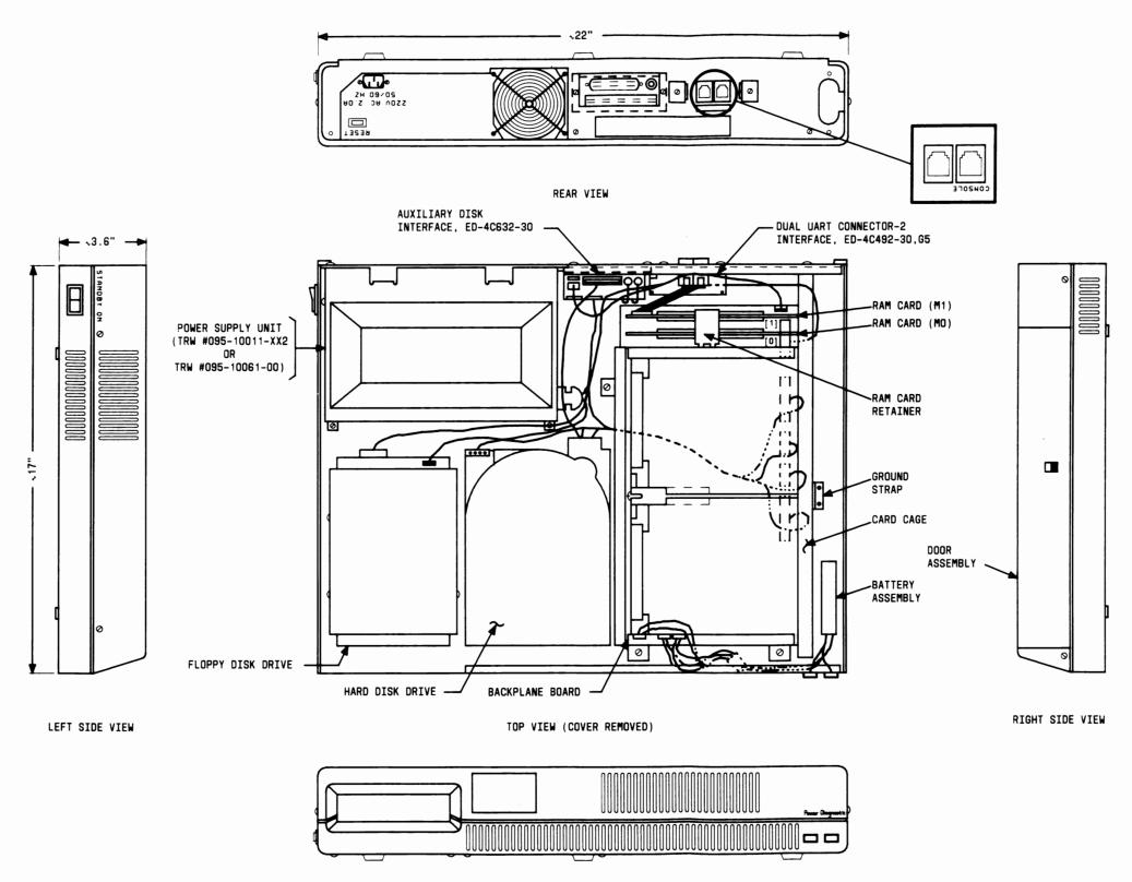
Figure 2-2: International 3B2/300 Computer Cabinet Assembly Drawing (ED-4C560-30)
