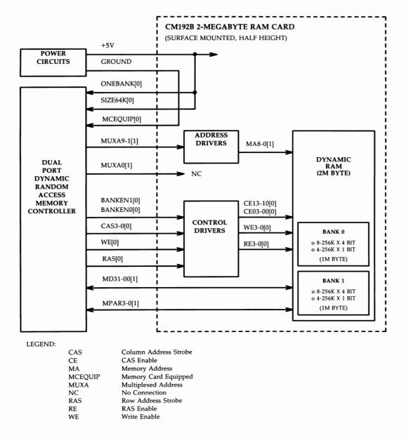
Figure 3-43: CM192B 2-Megabyte, Surface Mounted, Half Height, RAM Card — Functional Block Diagram
