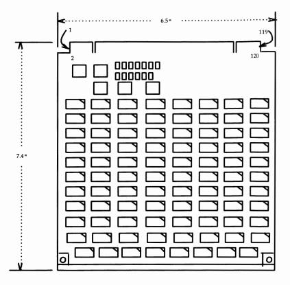
Conventional Component Side (Top) (Bottom Side also has Memory Chips)
