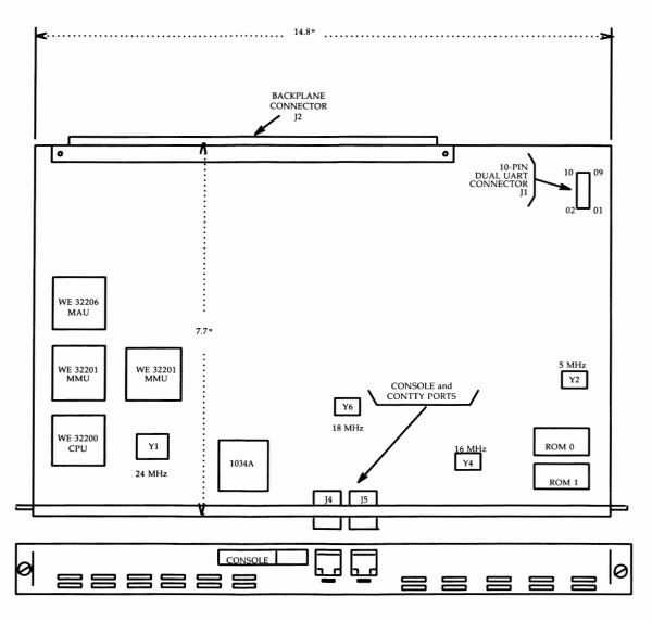
Figure 2-27: CM518C System Board Layout
