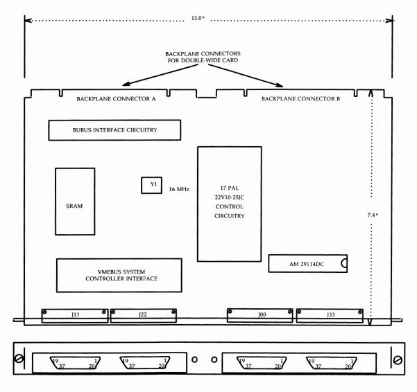
Figure B-34: CM525B VMEbus Card Layout
