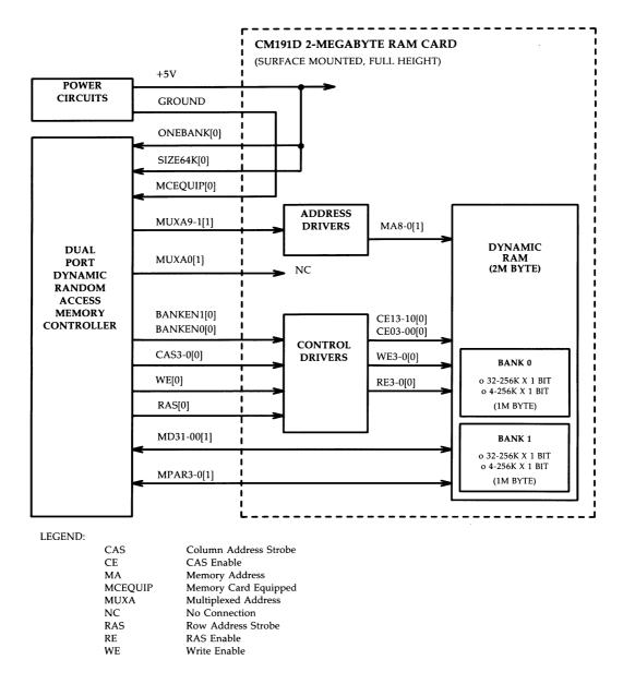
Figure 3-42: CM191D 2-Megabyte, Surface Mounted, Full Height, RAM Card — Functional Block Diagram
