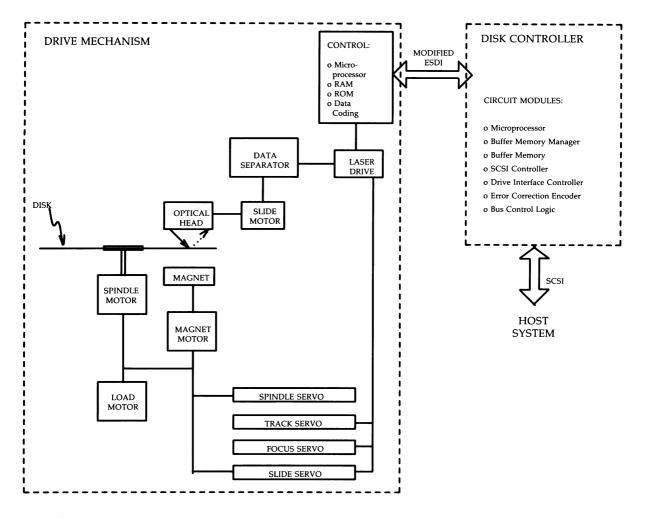
Figure 3-95: SCSI Rewritable Optical Disk Drive — Functional Block Diagram
