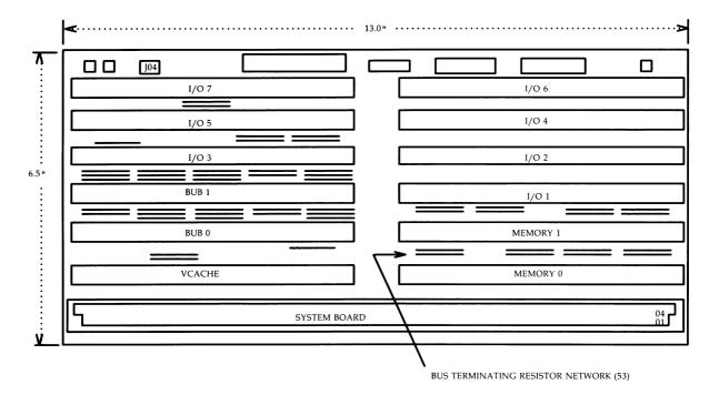
Figure 2-41: CM520A Backplane Board Layout
