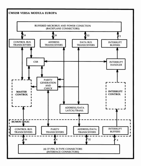
Figure 3-83: CM525B VMEbus Card — Functional Block Diagram
