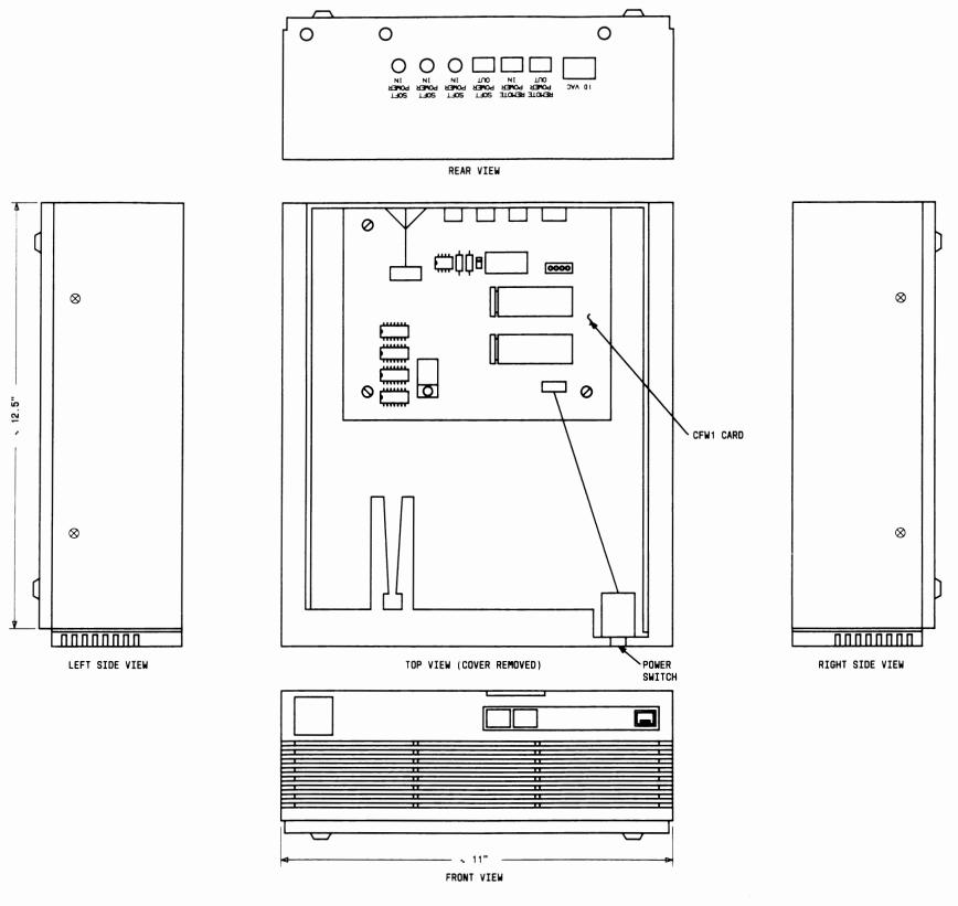
Figure 2-22: AT&T PPCU Cabinet Assembly Drawing (ED-3T011-30,G10)
