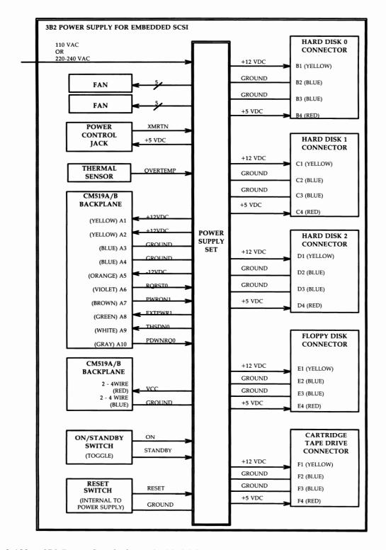
Figure 3-102: 3B2 Power Supply for Embedded SCSI— Functional Block Diagram
