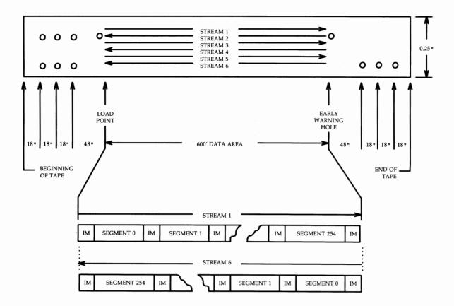
Figure 3-89: Cartridge Tape Physical Layout
