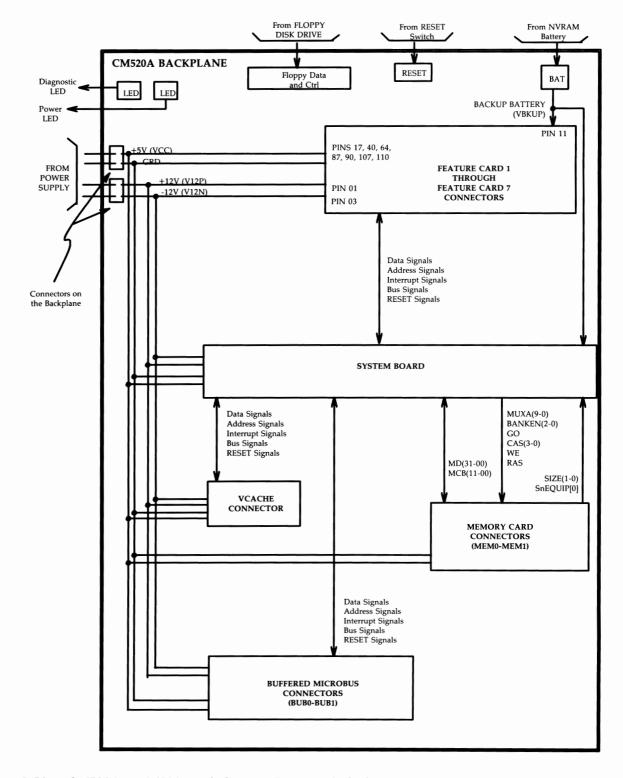
Figure 3-52: CM520A (3B2/500) Backplane — Functional Block Diagram
