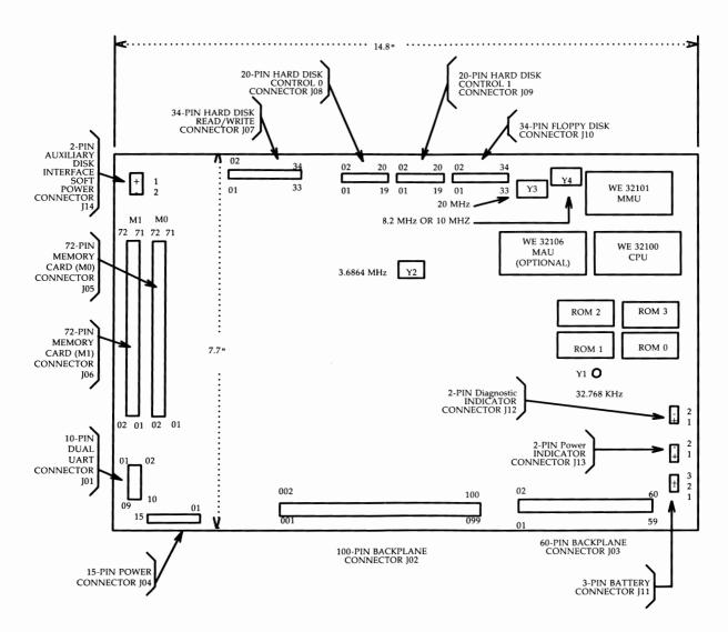
Figure 2-24: System Board, ED-4C637-30 Layout
