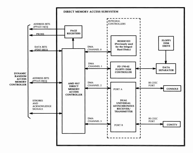
Figure 3-38: Direct Memory Access Subsystem — Functional Block Diagram
