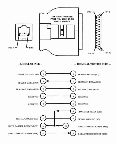
Figure B-39: Terminal/Printer Male Connector (232-21-25-010) Pin Identification
