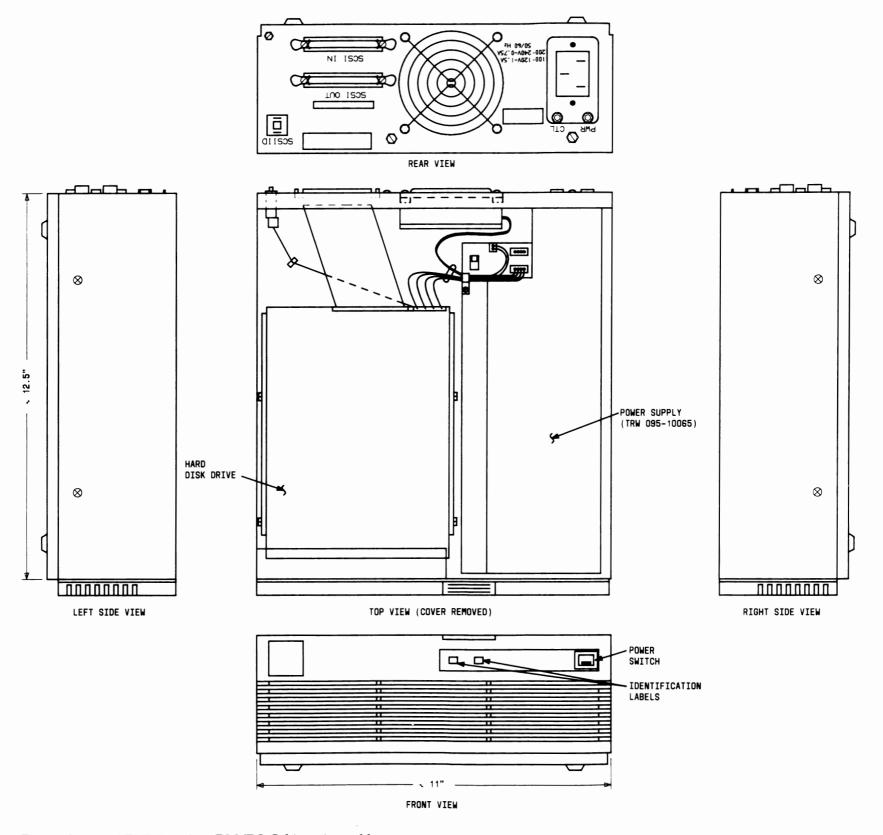
Figure 2-17: AT&T DM/S or DM/DS Cabinet Assembly Drawing (ED-3T011-30,G8,G9,G11)
