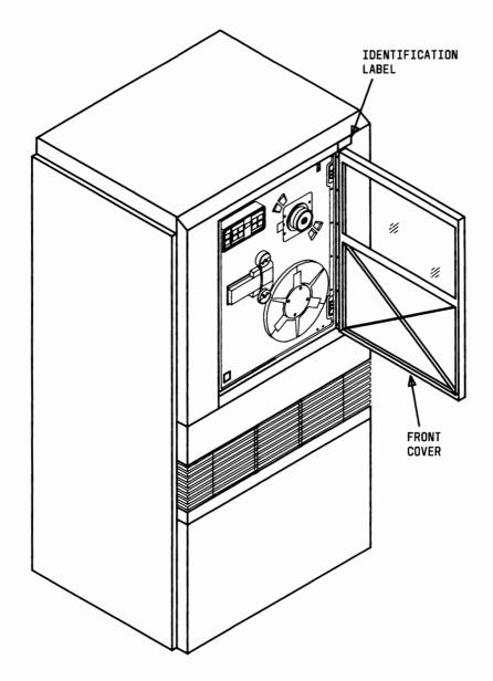
Figure 2-19: SCSI Manual Loading 9-Track Tape Cabinet
