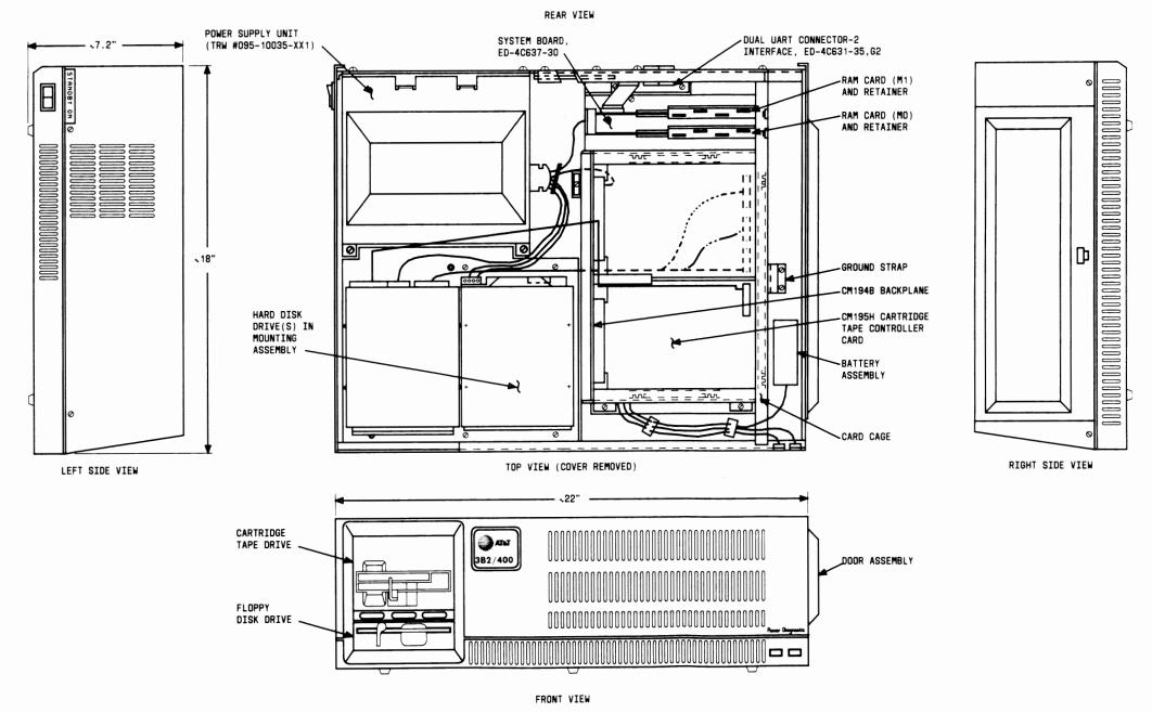
Figure 2-5: Domestic 3B2/400 Computer Cabinet Assembly Drawing (ED-4C631-30)
