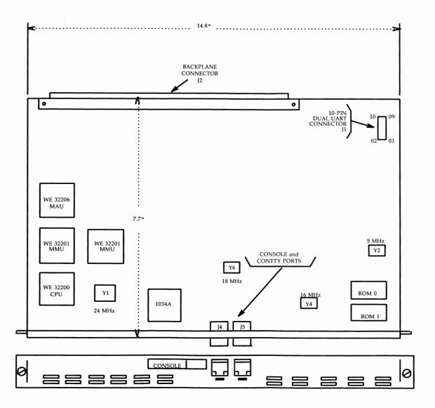
Figure 2-27: CM518C System Board Layout
