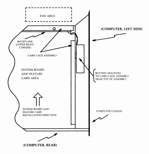
Figure 2-65: 3B2/600, 700, and 1000 Computer Backup Battery Supply Position
