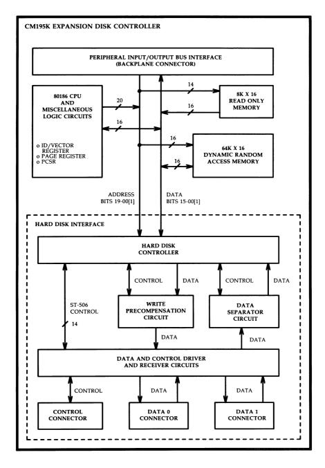
Figure 3-67: CM195K XDC Card — Functional Block Diagram
