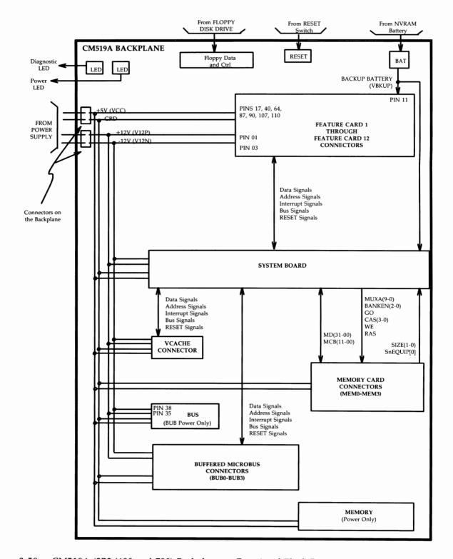
Figure 3-50: CM519A (3B2/600 and 700) Backplane — Functional Block Diagram
