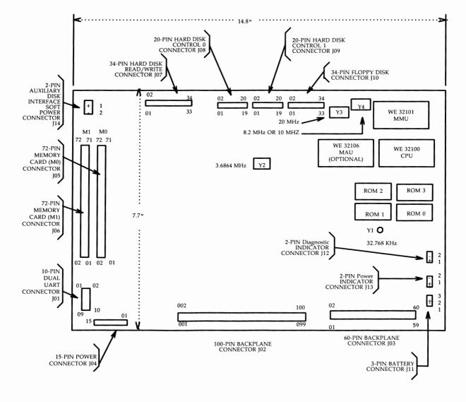
Figure 2-24: System Board, ED-4C637-30 Layout
