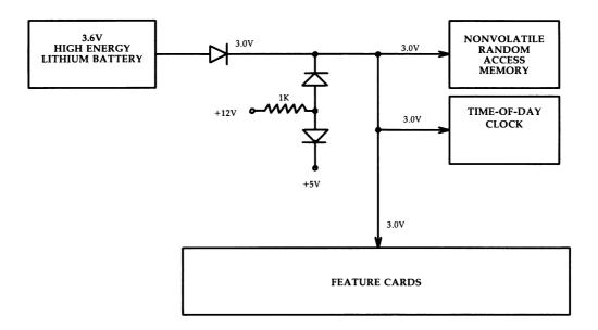
NOTE: The battery connects to the system board on Version 2 computers and to the backplane on Version 3 computers.
