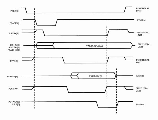
Figure 3-8: Peripheral Controller Main Memory Read Operation
