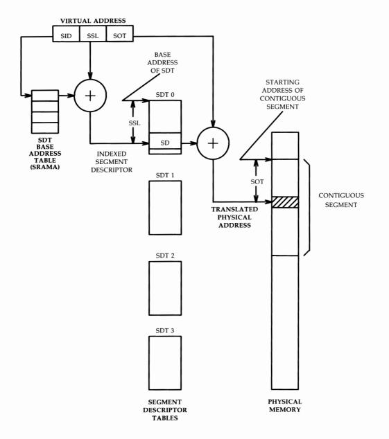
Figure 3-18: Virtual Address to Physical Address Translation for Contiguous Segments
