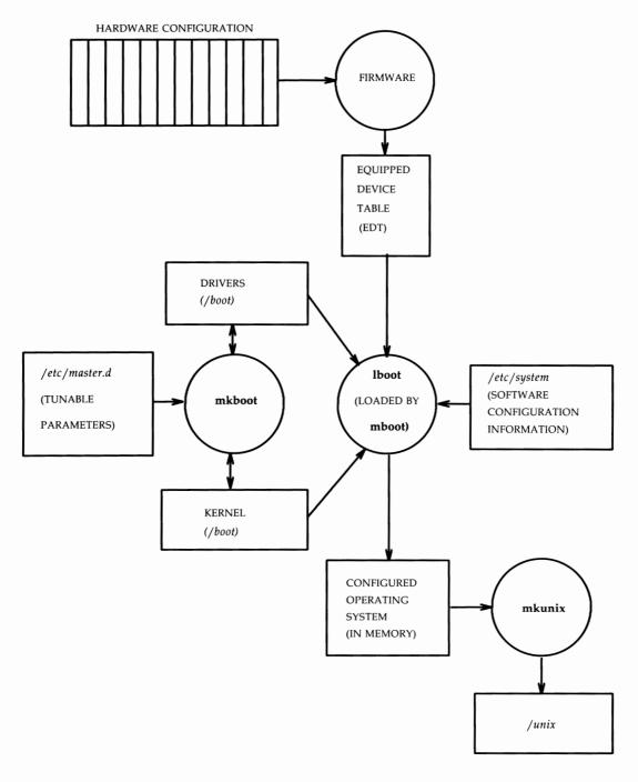
Figure 3-12: Self-Configuration Process
