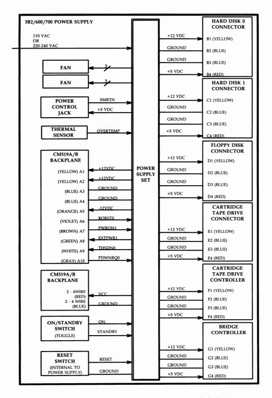
Figure 3-101: 3B2/600 and 700 Computer Power Supply — Functional Block Diagram
