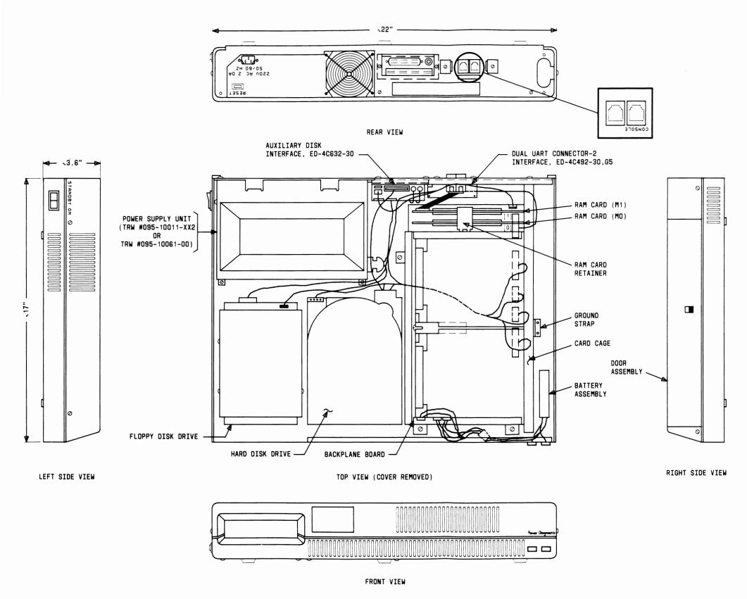
Figure 2-4: International 3B2/310 Computer Cabinet Assembly Drawing (ED-4C646-30)
