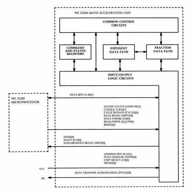
Figure 3-32: WE 32206 Math Acceleration Unit - Functional Block Diagram
