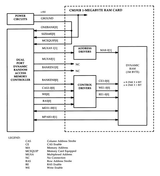
Figure 3-40: CM191B 1-Megabyte RAM Card — Functional Block Diagram
