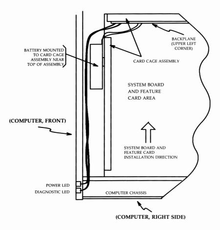
Figure 2-64: 3B2/500 Computer Backup Battery Supply Position
