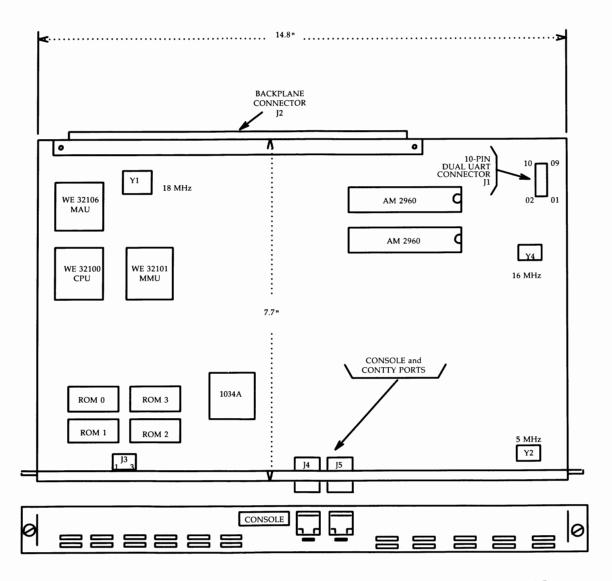
Figure 2-25: CM518A System Board Layout
