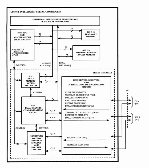
Figure 3-69: CM195T ISC Card — Functional Block Diagram
