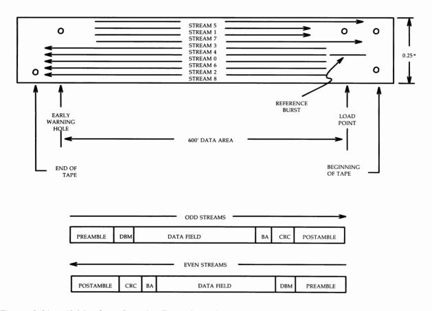
Figure 3-91: 60-Megabyte Cartridge Tape Physical Layout
