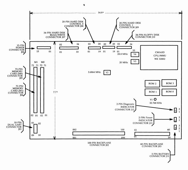
Figure B-1: CM190A System Board Layout
