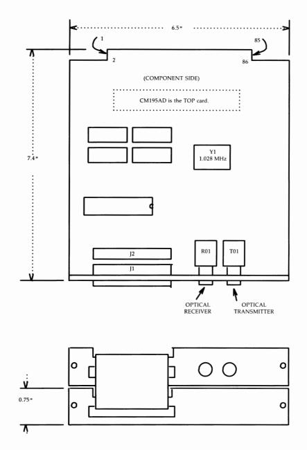
Figure 2-46: CM195AC/CM195AD Datakit VCS Interface Card Layout
