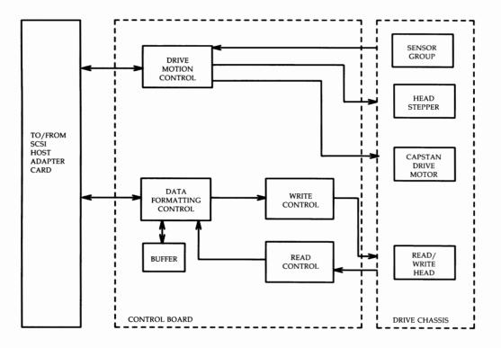
Figure 3-94: 120-Megabyte Cartridge Tape Drive — Functional Block Diagram
