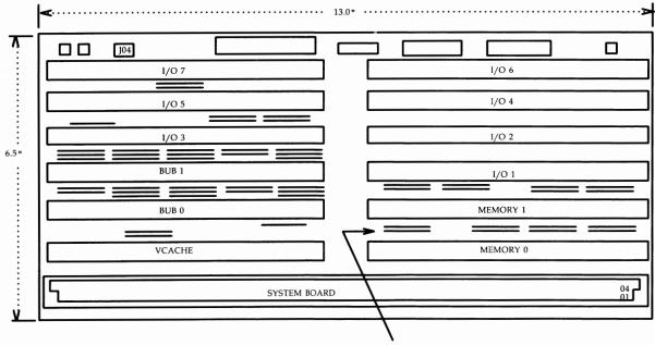
BUS TERMINATING RESISTOR NETWORK (53)
