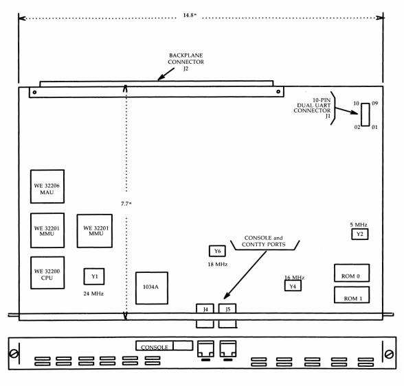
Figure B-5: CM518C System Board Layout
