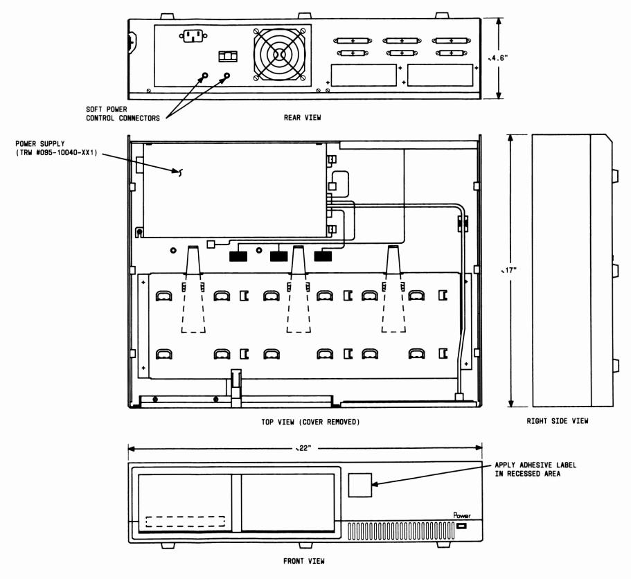
Figure 2-11: Domestic AT&T/XM Cabinet Assembly Drawing (ED-4C580-30)
