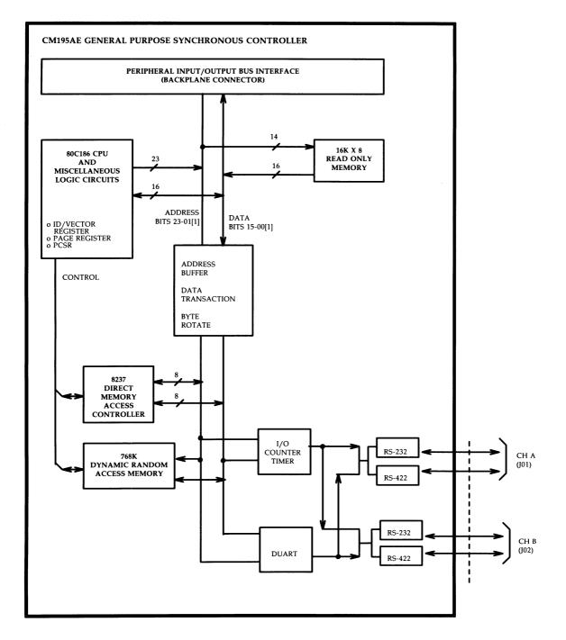
Figure 3-59: CM195AE GPSC Card—Functional Block Diagram
