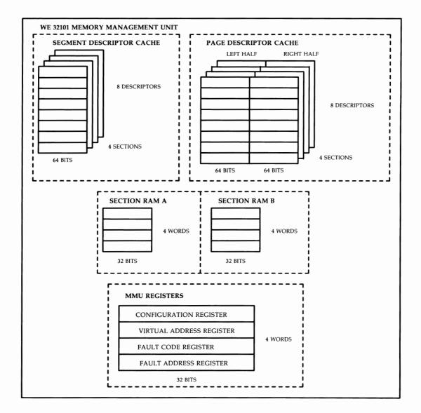
Figure 3-16: WE 32101 MMU Block Diagram
