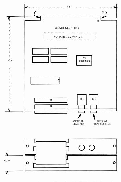
Figure B-22: CM195AC/CM195AD Datakit VCS Interface Card Layout
