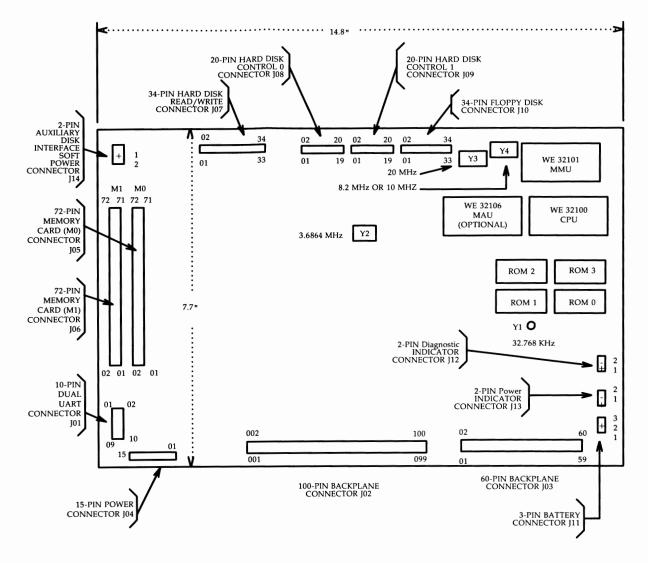
Figure B-2: System Board, ED-4C637-30 Layout
