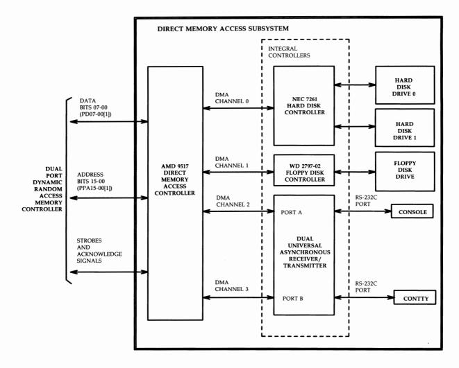
Figure 3-26: Direct Memory Access Subsystem — Functional Block Diagram
