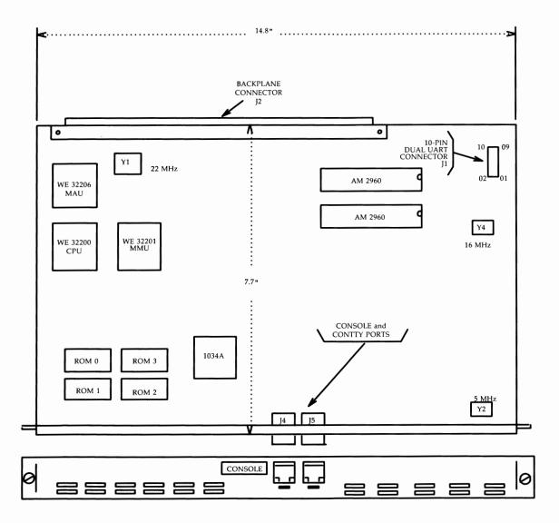
Figure B-4: CM518B System Board Layout
