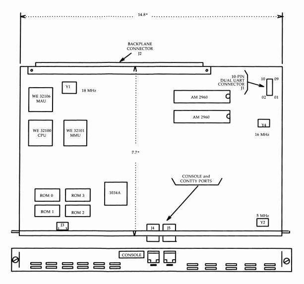
Figure B-3: CM518A System Board Layout
