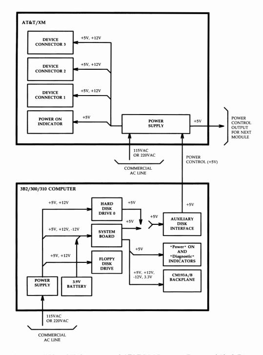
Figure 3-96: 3B2/300 or 310 Computer and AT&T/XM Power — Functional Block Diagram
