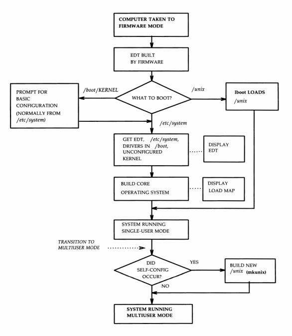
Figure 3-11: Self-Configuration - Manual Boot Sequence
