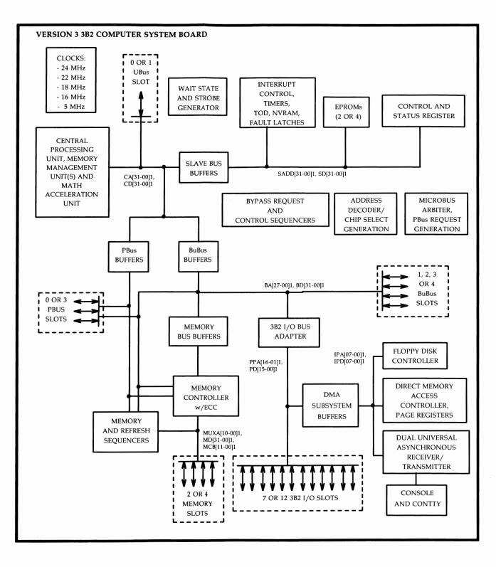
Figure 3-27: Version 3 3B2 Computer System Board — Functional Block Diagram
