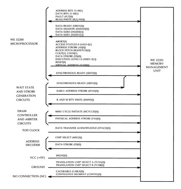
Figure 3-29: WE 32201 MMU Interconnection Diagram
