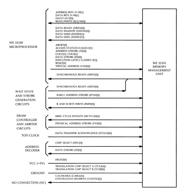
Figure 3-15: WE 32101 MMU Interconnection Diagram
