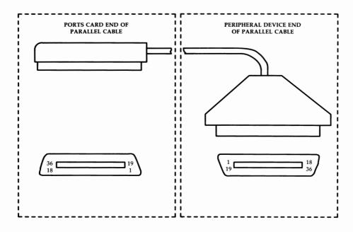
Figure B-43: CENTRONICS Connectorized Cable Pin Identification
