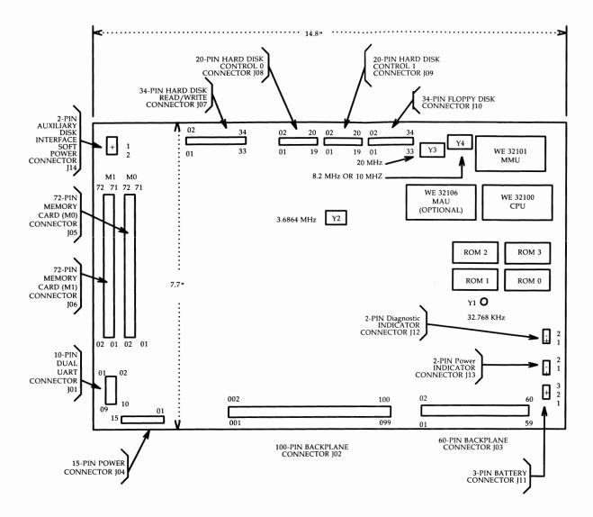
Figure B-2: System Board, ED-4C637-30 Layout
