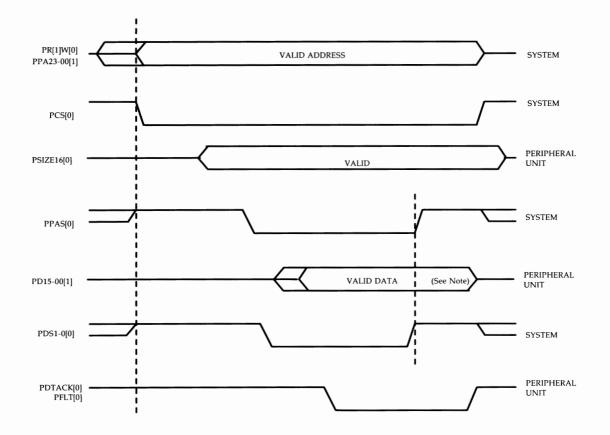
Note: Data is valid at system board for at least 20 nanoseconds before PDTACK[0].
