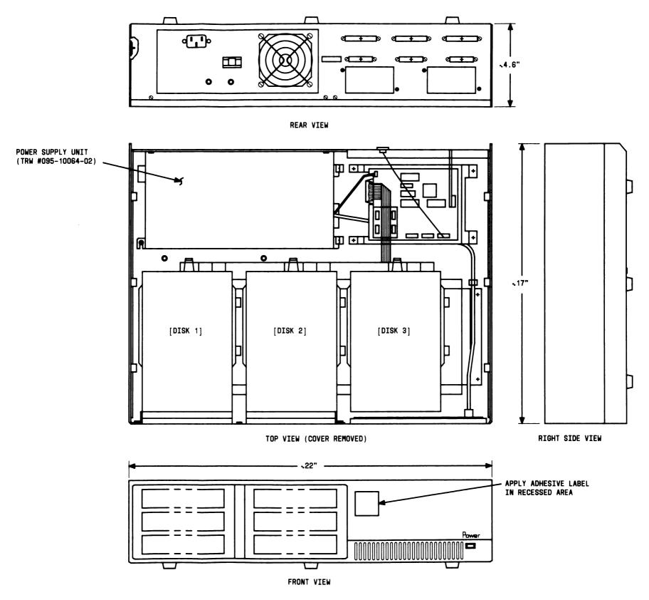
Figure 2-13: Domestic AT&T XM/405S/900S Cabinet Assembly Drawing (ED-3T010-30)
