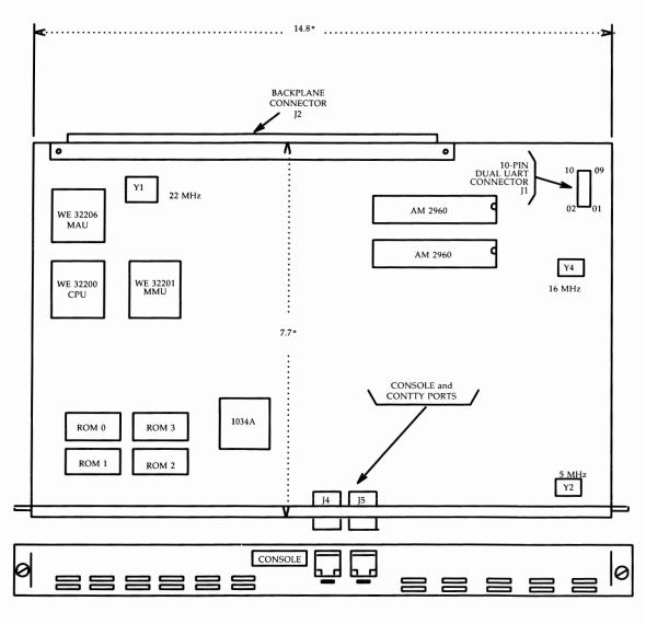
Figure B-4: CM518B System Board Layout
