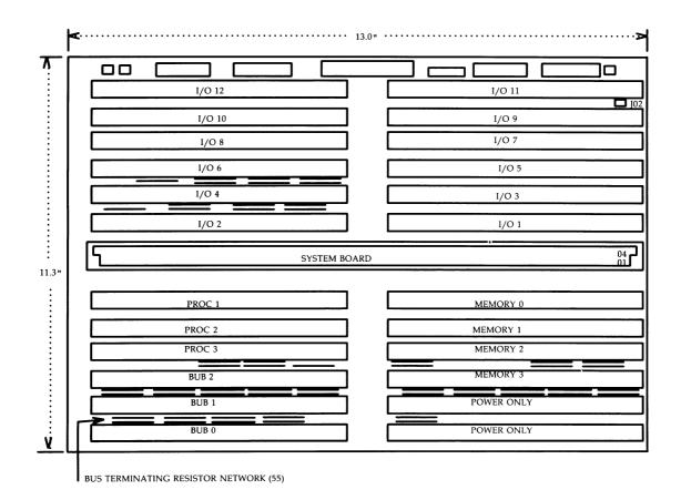
Figure 2-40: CM519B Backplane Board Layout
