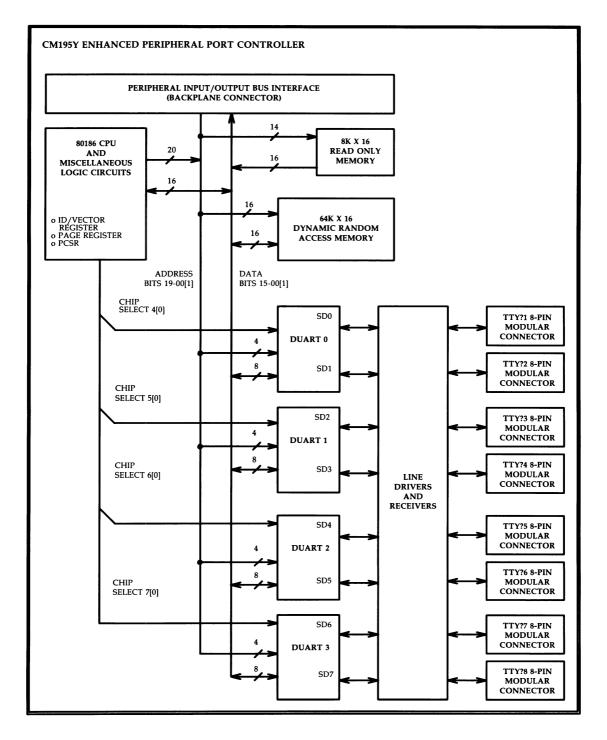
Figure 3-75: CM195Y EPORTS Card — Functional Block Diagram
