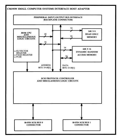
Figure 3-73: CM195W SCSI Host Adapter Card — Functional Block Diagram
