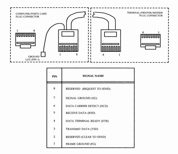
Figure B-42: 8-Conductor Modular Cable Connector Pin Identification
