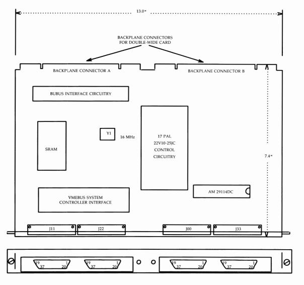
Figure 2-61: CM525B VMEbus Card Layout
