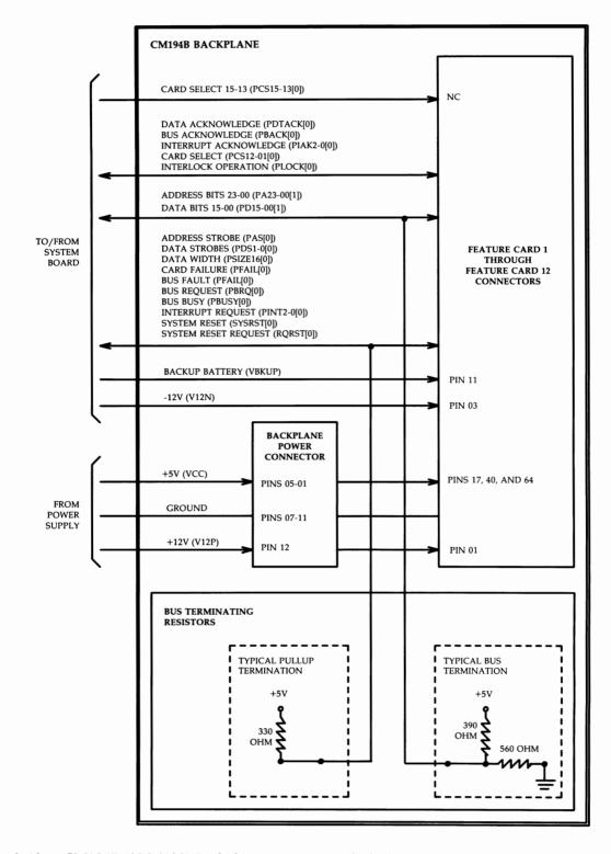
Figure 3-49: CM194B (3B2/400) Backplane — Functional Block Diagram
