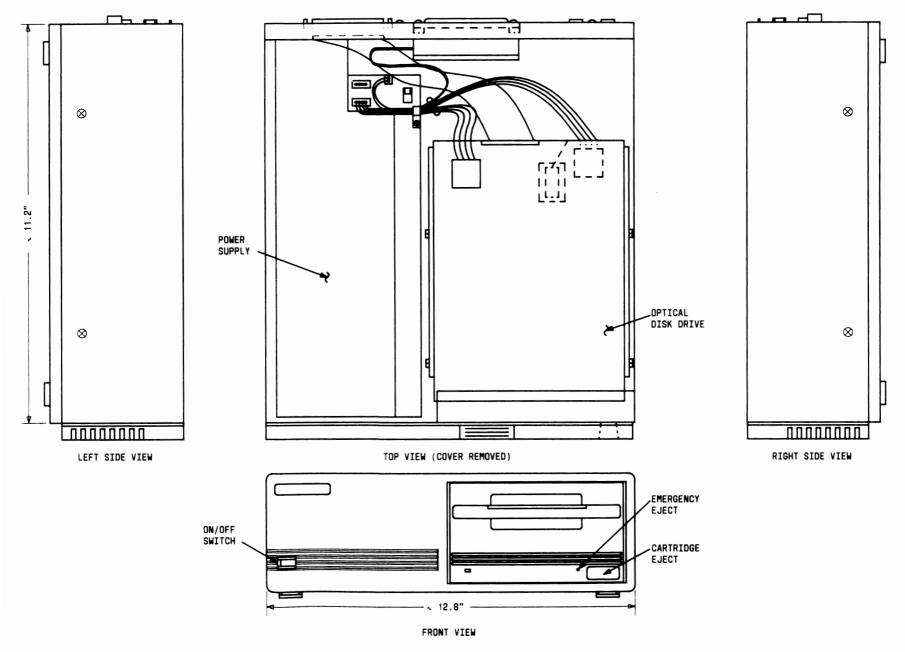
Figure 2-18: AT&T SCSI Rewritable Optical Disk Cabinet Assembly Drawing
