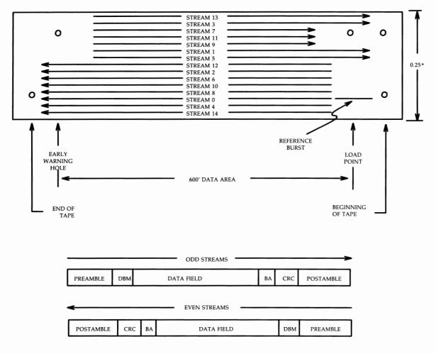
Figure 3-93: 120-Megabyte Cartridge Tape Physical Layout
