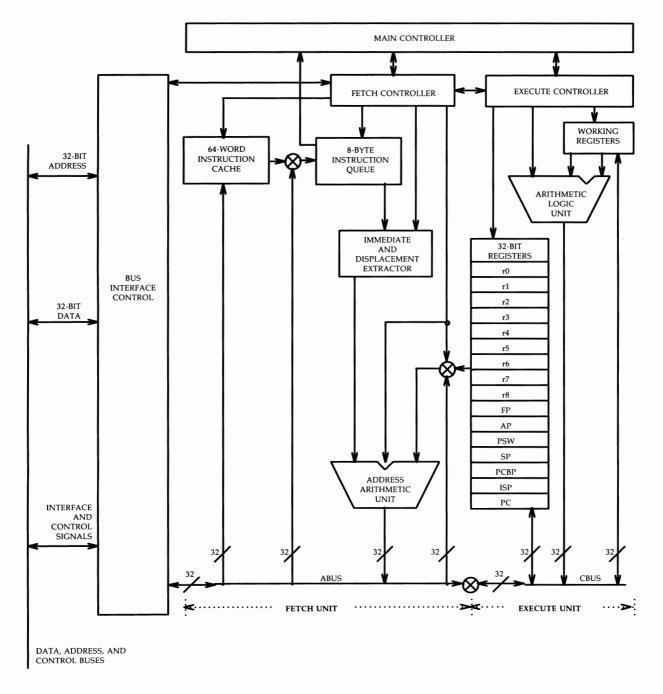
Figure 3-14: System Board CPU — Functional Block Diagram
