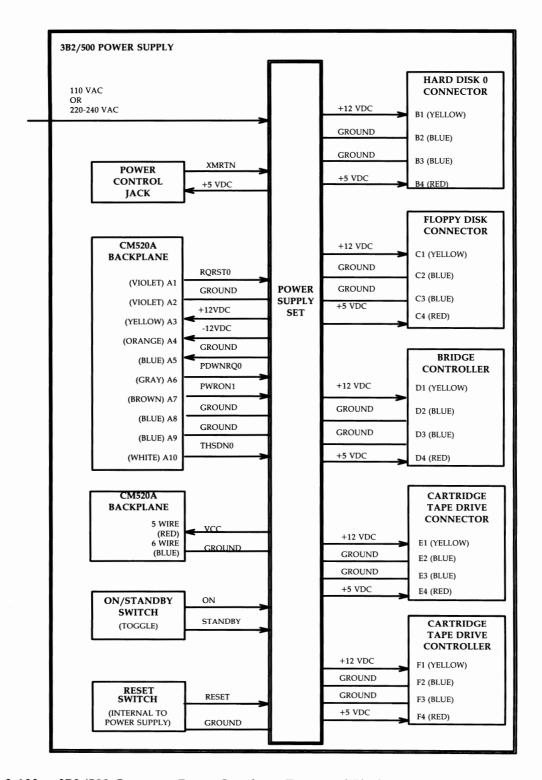
Figure 3-100: 3B2/500 Computer Power Supply — Functional Block Diagram
