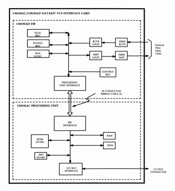
Figure 3-57: CM195AC/CM195AD Datakit VCS Interface Card — Functional Block Diagram
