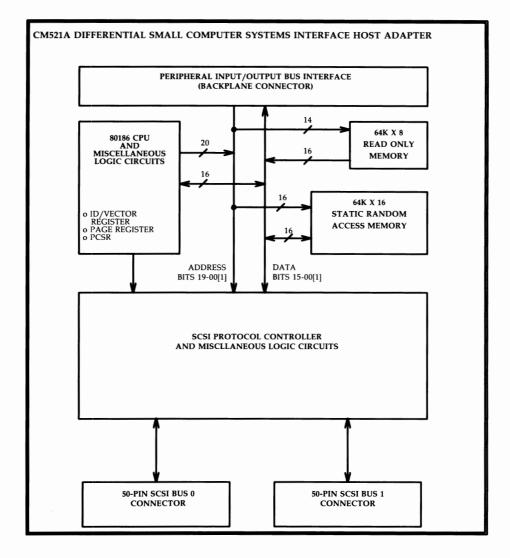
Figure 3-77: CM521A Differential SCSI Host Adapter Card — Functional Block Diagram
