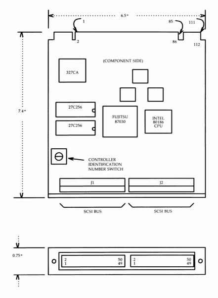
Figure 2-58: CM521A Differential SCSI Host Adapter Card Layout
