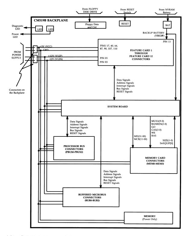
Figure 3-51: CM519B (3B2/1000) Backplane — Functional Block Diagram
