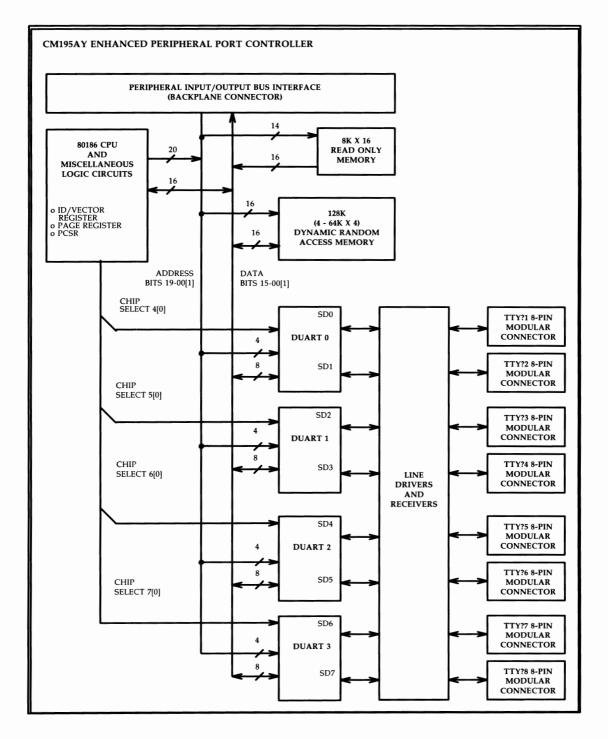
Figure 3-61: CM195AY EPORTS Card — Functional Block Diagram
