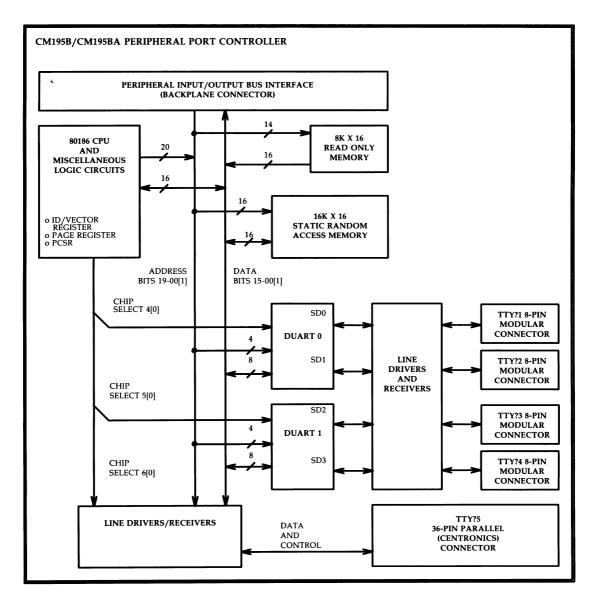
Figure 3-63: CM195B/CM195BA PORTS Card — Functional Block Diagram
