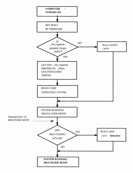
Figure 3-10: Self-Configuration — Powerup Sequence
