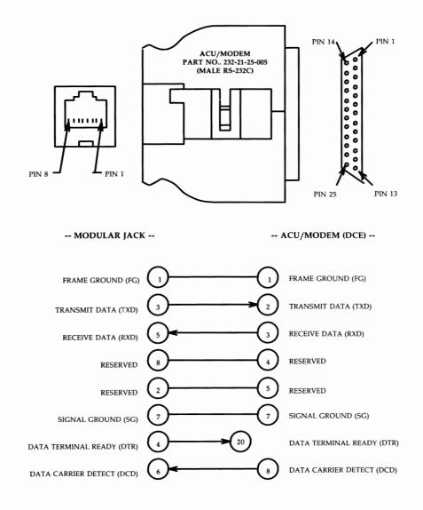
Figure B-37: ACU/MODEM Connector (232-21-25-005) Pin Identification
