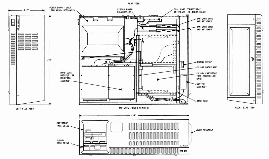
Figure 2-6: International 3B2/400 Computer Cabinet Assembly Drawing (ED-4C638-30)
