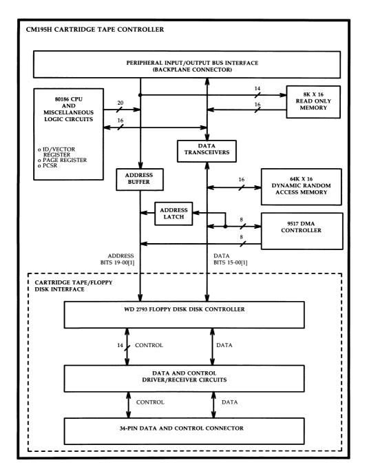
Figure 3-65: CM195H CTC Card — Functional Block Diagram
