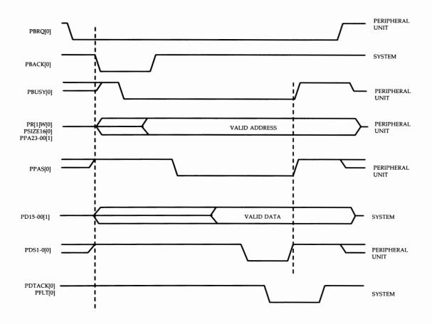
Figure 3-9: Peripheral Controller Main Memory Write Operation
