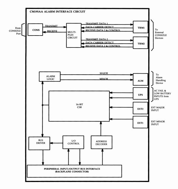
Figure 3-55: CM195AA AIC Card — Functional Block Diagram
