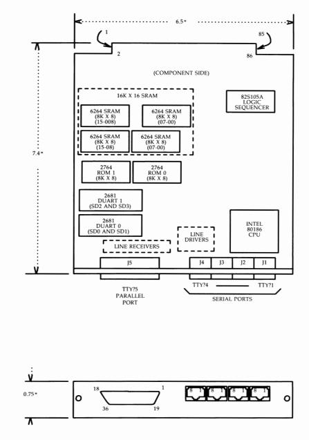
Figure 2-49: CM195B PORTS Card Layout (Early Production)
