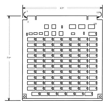
Conventional Component Side (Top) (Bottom Side also has Memory Chips)
