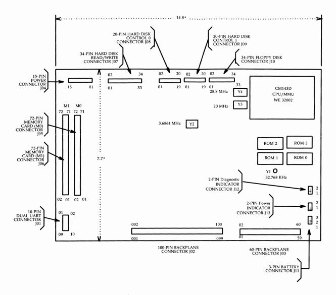
Figure B-1: CM190A System Board Layout
