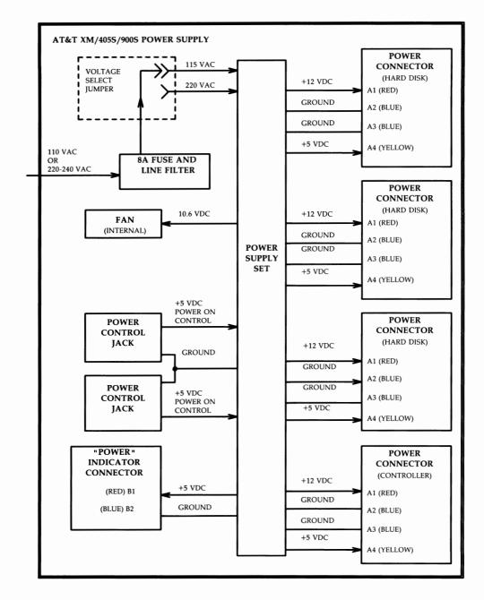
Figure 3-105: AT&T XM/405S/900S Power Supply — Functional Block Diagram
