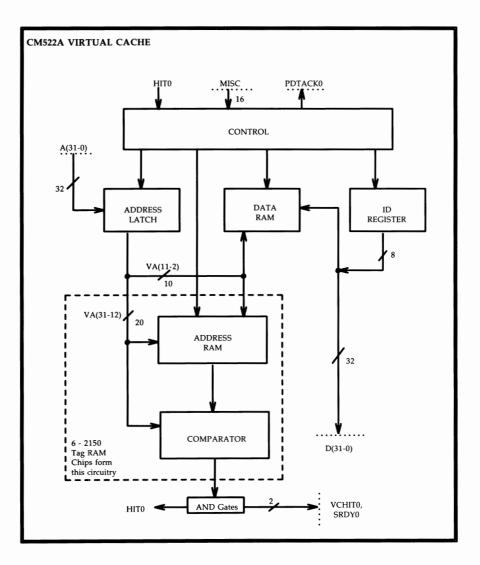
Figure 3-79: CM522A VCACHE Card — Functional Block Diagram
