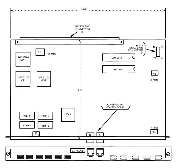
Figure B-3: CM518A System Board Layout
