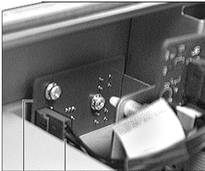
NMI/Reset Power Interconnect Board
