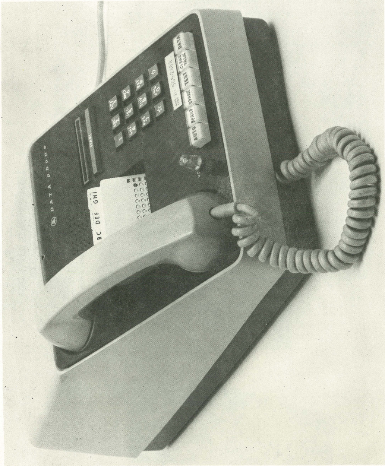
FIGURE 2 DATA SET TYPE 103G WITH TOUCH-TONE DIAL AND CARD DIALER
