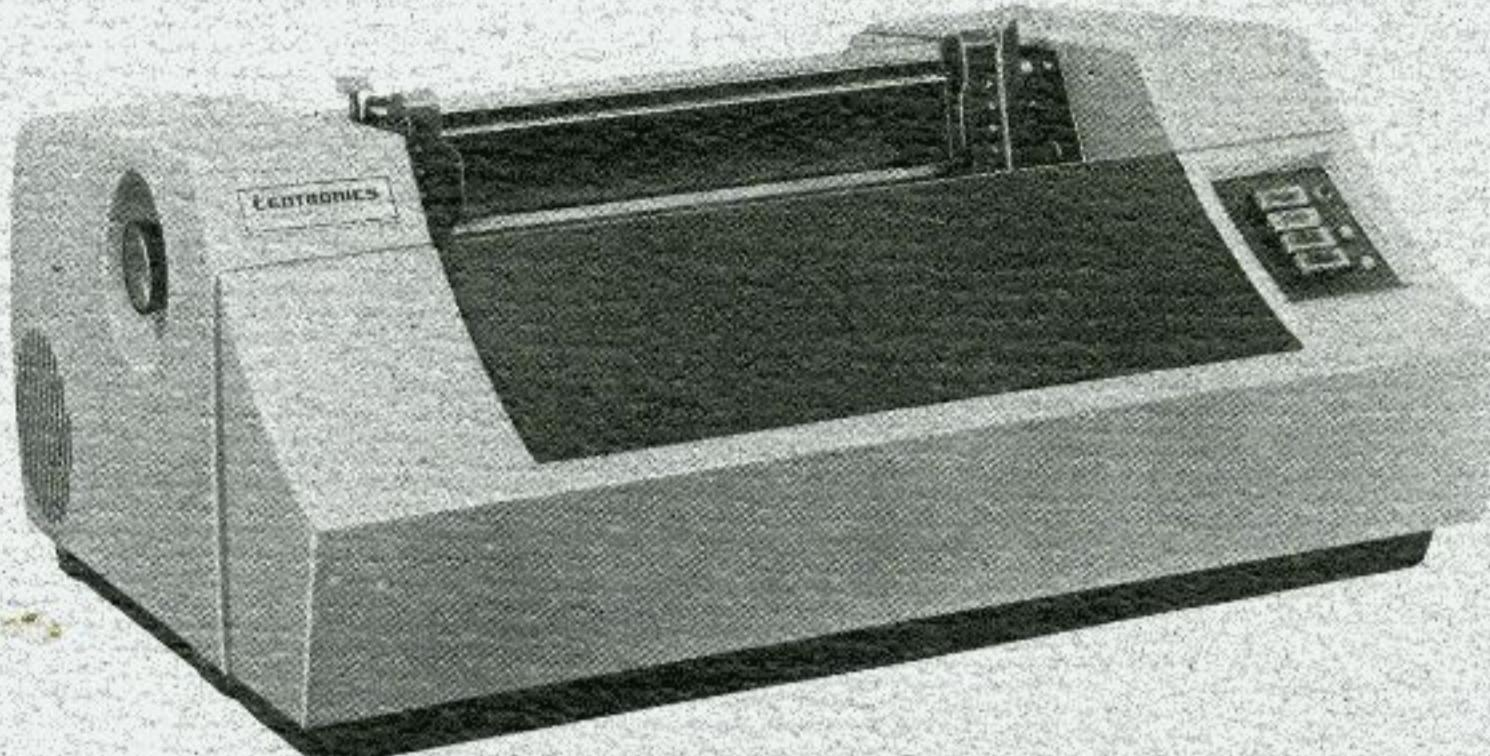
The 101AL is a medium speed, serial, impact printer which uses LSI (Large Scale Integration) electronics. The printer employs the dot matrix technique for generating characters in a 9 x 7 pattern. The 101AL will produce an original plus up to four clear carbon copies and the last printed line is visible for immediate reading.
