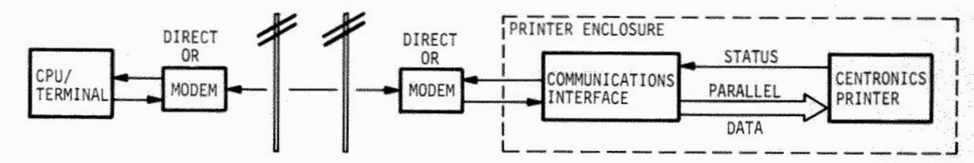
To allow direct coupling between any of its printers and a modem or data set, Centronics offers the following three communications interfaces:
