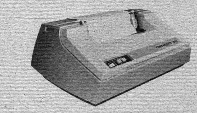
The 501 is a low cost 165 character per second 5 x 7 dot matrix, serial, impact printer that establishes a new price/performance standard. A wide range of options allows the printer to be styled for specific application requirements. Capable of producing an original plus up to four clear carbon copies, the 501 can operate with the paper supply located to the rear or below the printer.
