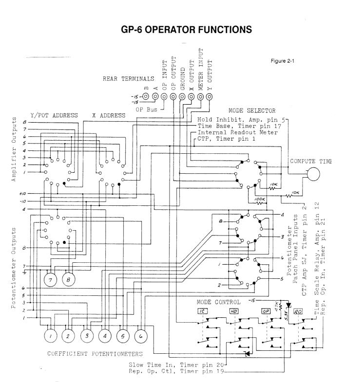
Figure 2-1 is a schematic of operator functions. Descriptions of the individual operations are described in the following:
