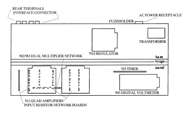
Input summing resistors for integrator and summer amplifiers are located on the **Input Resistor Network Boards**. Resistors are 5.00Kand 50.0K, metal film, 0.1%.
