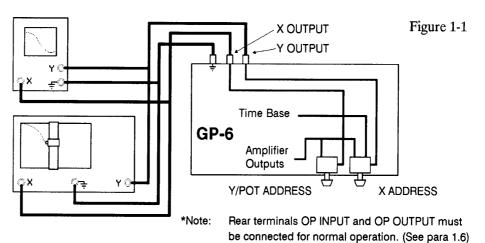
Rear binding post terminals offer convenient connections to the X and Y inputs of the plotter and/or oscilloscope. The three connections are shown in Figure 1-1 and listed below.
