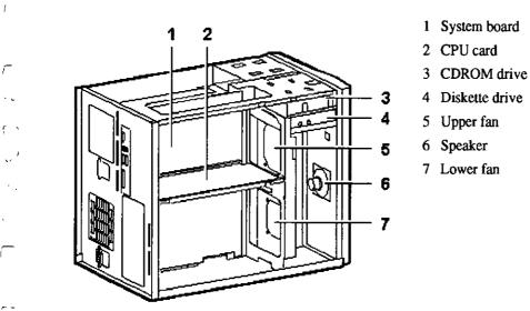
Figure 9-4 shows system components on the power supply side with the side panel removed.
