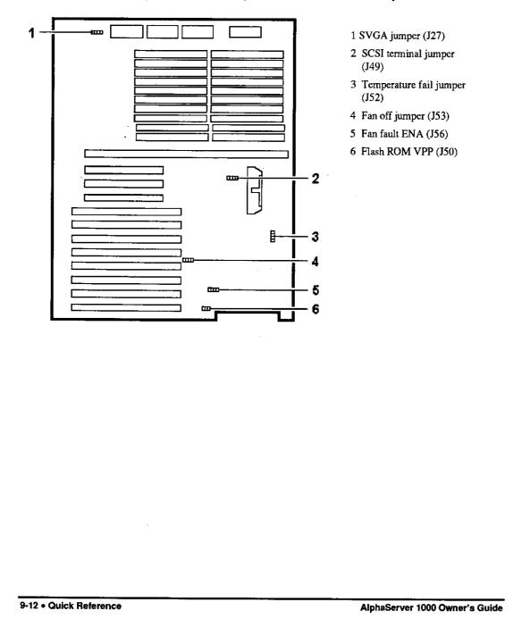
Figure 9-6 System Board Jumper Positions for Normal Operation
