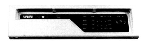
Figure A-1 Pushbutton Console
