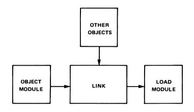
Figure 11-6 The Link Operation
