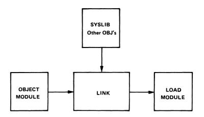
Figure 9-4 The Link Operation
