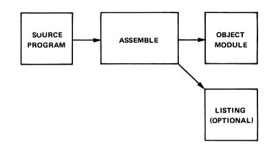
Figure 11-3 Function of a MACRO-11 Assembler
