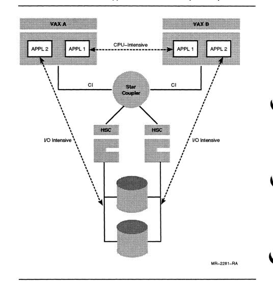
Figure 2–1 Comparing the Direction of Information Flow for an I/O-Intensive Application Distributed by Replication and a CPU-Intensive Application Distributed by Decomposition
