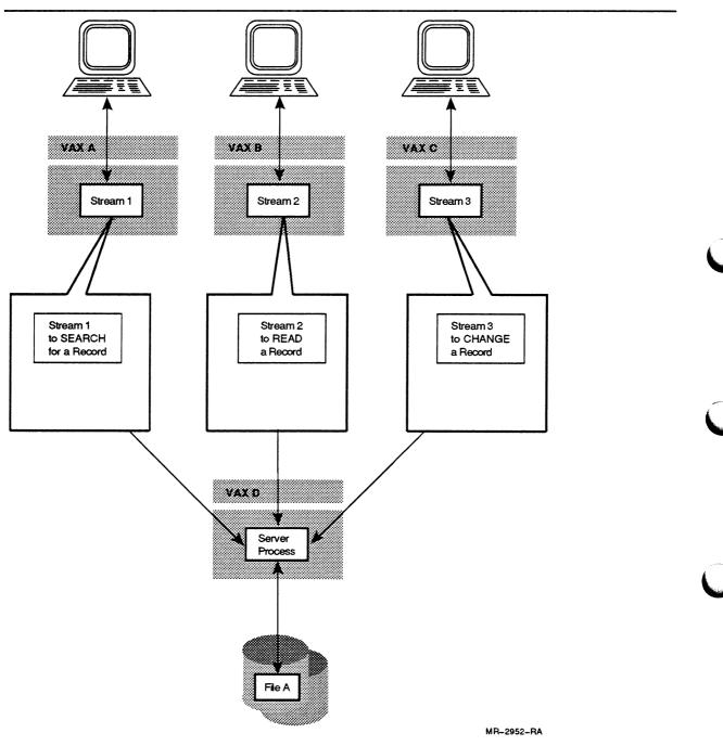
A file or database server is probably the most common implementation of the Many-to-One Client-Server Model in the VAXcluster application environment. Rather than having an application access a file directly, the application requests file access from the remote server process.
