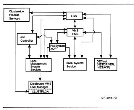
Figure 3–1 Functional Relationship of VAXcluster System Programming Tools
