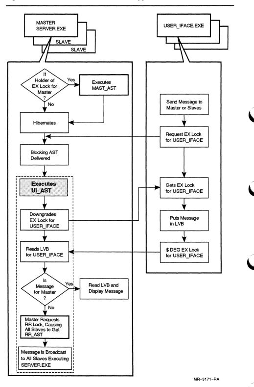
Figure 8–6 Modules for Demonstration Application
