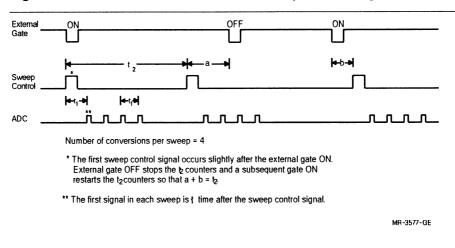
Figure A-16: Clock Mode 16, Timed Sweeps, with Edge Gate
