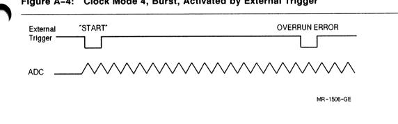
Figure A-4: Clock Mode 4, Burst, Activated by External Trigger
