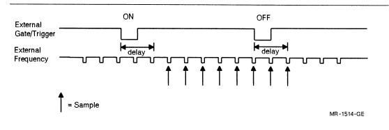
Figure A-22: Clock Mode 22, External Triggers, with Delayed Edge Gate
