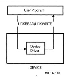
The synchronous I/O interface is recommended for applications that examine or modify the data between I/O operations, such as single-point or slow data acquisition and closed loop control. High-speed applications requiring only one buffer of data to complete I/O operations can also benefit from using synchronous I/O routine calls.
