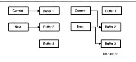
This allows the data to be transferred continuously, without having to wait for the time it takes the software to set up the next buffer. Of course, the time it takes to transfer the first buffer must be greater than the time it takes to set up for the next buffer.
