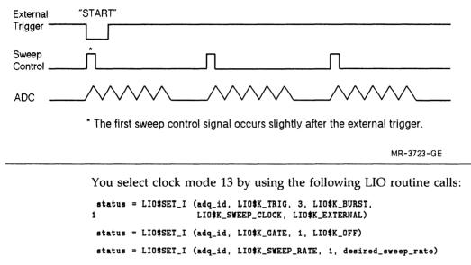
The GATE set parameter is not needed unless you previously enabled gating.
