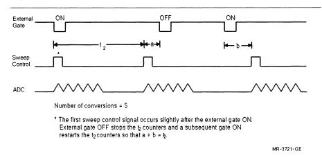
Figure A-11: Clock Mode 11, Burst Sweeps, with Edge Gate
