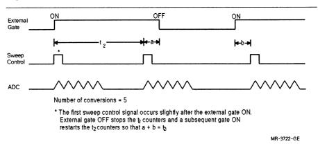
Figure A-12: Clock Mode 12, Burst Sweeps, with Level Gate
