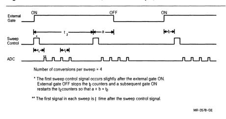
Figure A-17: Clock Mode 17, Timed Sweeps, with Level Gate
