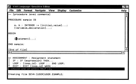
A menu of options appears at the bottom of the screen. The options ASSIGNMENT and IF are tokens that you can expand into templates. The text after each token describes what will be inserted into your buffer if you select that token.
