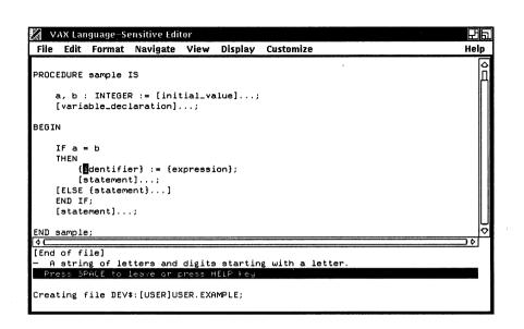
2. Press the spacebar to remove the information about {identifier} ....
