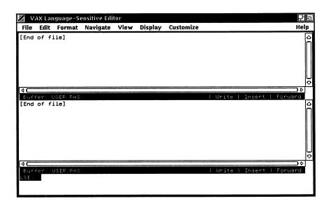
Each window in the work region has a **status line**. The status line is highlighted and provides information about the associated buffer. The status line tells you the name of the buffer, whether the buffer is a write or readonly buffer, whether you are in insert or overstrike mode, and whether the buffer is in a forward or reverse direction.
