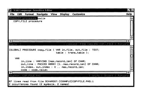
This query display works just like the previous ones. You can use the NEXT STEP and PREVIOUS STEP commands to select entries. You can expand a symbol into its corresponding set of occurrences, and you can go to a source from any of those occurrences.
