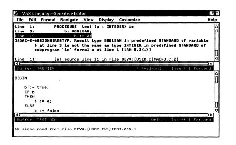
Figure 16–2 shows the screen after the GOTO SOURCE command is executed with the cursor positioned on the line number of the second diagnostic. The supplied text from the text region refers to the expanded macro "test" in the source.
