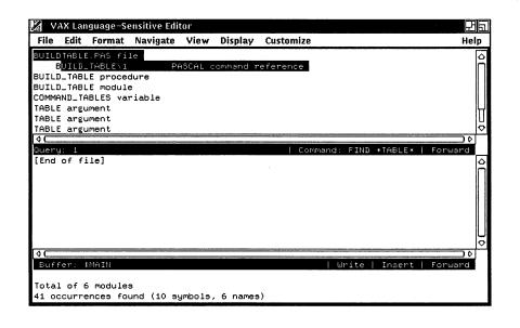
This query display shows the name and the class of all of the symbols whose name contains "table." The first symbol is a file named BUILDTABLE.PAS. The first symbol has already been expanded. The second one is a procedure named BUILD\_TABLE.
