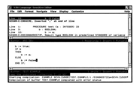
Corrections accompany some errors. For example, in Figure 2–16, the compiler supplied a correction for the missing semicolon. You can accept or reject the correction.
