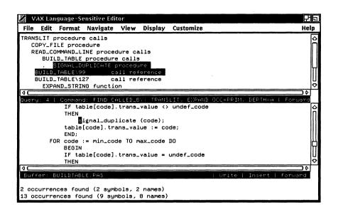
The query display shows that SIGNAL\_DUPLICATE is called in two different places within the routine BUILD\_TABLE. The declaration of SIGNAL\_ DUPLICATE does not appear in the query result because SIGNAL\_ DUPLICATE calls only RTL routines. However, this does not pose a problem, because the GOTO DECLARATION/INDICATED command works in a query buffer. You can get to the declaration of SIGNAL\_DUPLICATE by using the GOTO DECLARATION/INDICATED command (CTRL/D).
