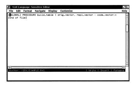
2. To expand the procedure to the next level of detail, press CTRL/E or CTRL// (the EXPAND key).
