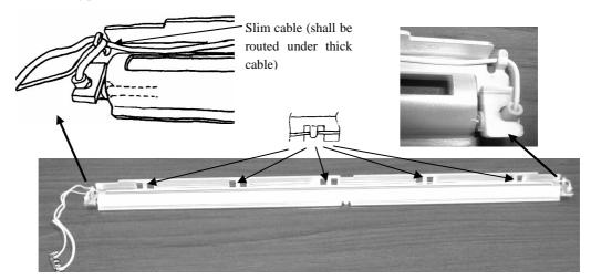
(2) After mounting the Lamp SR, perform the following adjustment:
