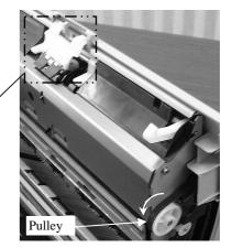
(3) Remove two screws (Self-tapping screw) from TOP cover
