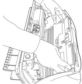
2) Rotate the Pick roller bushing in the direction of the arrow.
