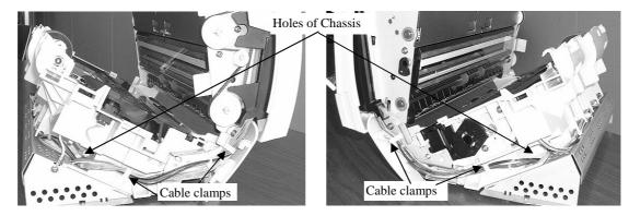
Note: Route the cables as shown in above figures when assembling.
