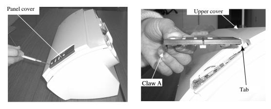
(3) Take out the Panel PCA and disconnect one connector from the Panel PCA.
