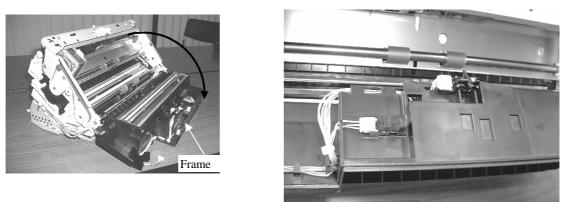
(6) Release the craws that fix the sensors and disconnect the connector of the sensor to remove.
