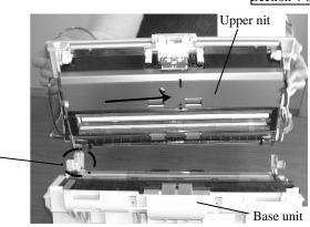
Note: When assembling the Upper unit, insert an arm of coil spring into a slot of bracket first, and insert the shaft to the hole of bracket as shown in the figure below. Then attach a plastic washer to another end of the shaft, and then insert the shaft into a hole of bracket as shown in the right figure.
