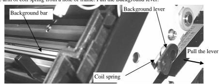
Note: Mounting procedure of the Background bar and Background lever is as follows.
