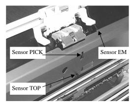
(1)How to activate Emulation mode Open the cover. Press Sensor PICK and Function button, and then press and release Power button. Keep pressing Sensor PICK and Function button until scanner shows Screen B on the panel. The interface between PC and scanner is entirely disabled in this mode. The following display appears during the scanner initialization in the emulation switching mode activation.
