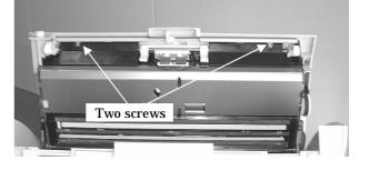
(4) Open the ADF a little, and open Upper cover by about 2 cm. Push Upper cover in E direction and press B portion down to unlock the craws inside of the cover. Then detach the Upper cover
