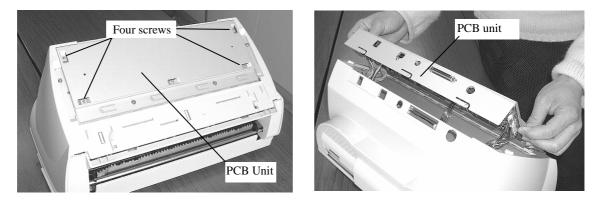
(2) Remove 4 screws from the PCB unit, and open the PCB unit a little taking care not to pull the cables inside by force.
