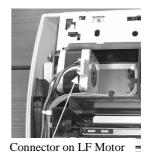
(4) Unhook the arm of coil spring from a hole of frame. Pull the Background lever.
