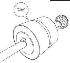
7. Attach the Pick roller shaft to the scanner.
