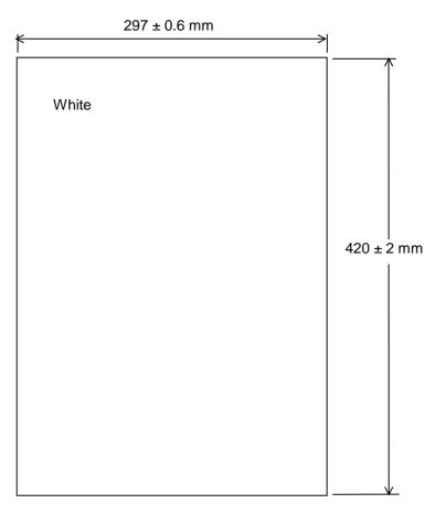
Figure 5-1-3. Test sheet for the magnification/offset adjustment
