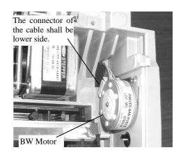
(2) When routing the motor cable on backside of the scanner, insert thinner cable first to avoid cables come out the hooks.
