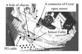
(3) Remove two screws from Base unit.
