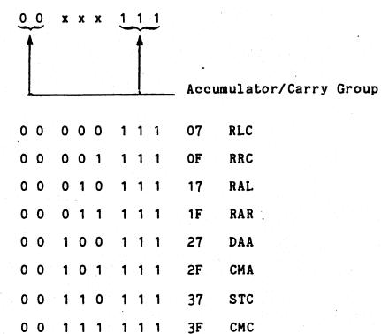
The rotate instructions shift the accumulator left or right.
