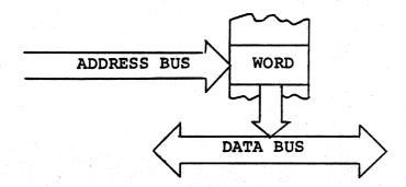
Read operations put the contents of a word onto the data bus.
