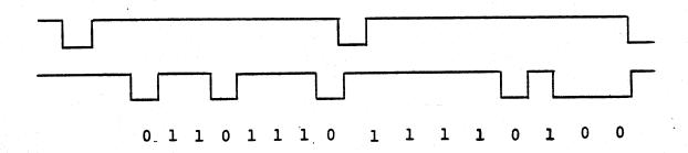
We can put time intervals between words on the data line and fit the word marks into the intervals. If they can be distinguished from the data bits (by a narrower or wider pulse, or a different frequency, for instance) they will still serve the same function.
