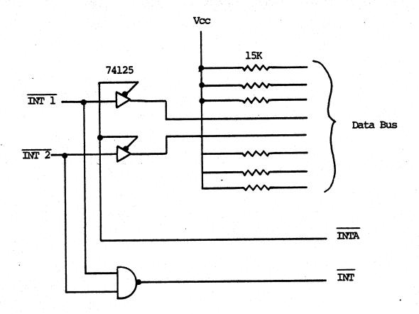
VECTORED INTERRUPT USING RESISTORS
