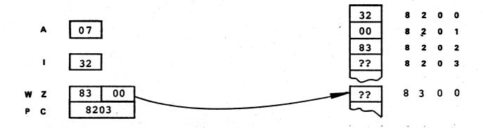
8) The processor sends the contents of the A register to address 8300 and the instruction is completed.
