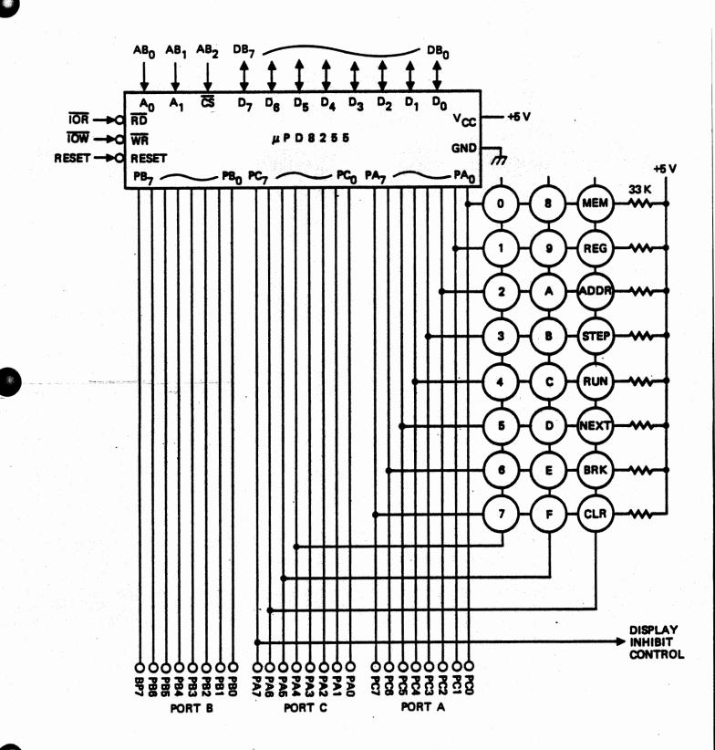
8255 and Key Input Scanning Circuit
