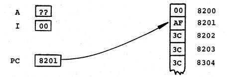
2) The memory sends the contents of address 8201 to the I register, and the (PC) is incremented.
