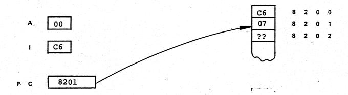
4) The memory sends the contents of address 8201, which is added to the contents of the A register, and (PC) is incremented by 1.
