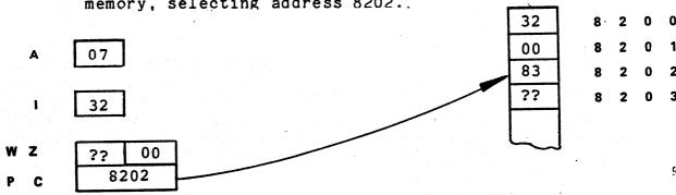
6) The memory sends the contents of 8202 to the W register, and (PC) is incremented by 1. The complete address in which the contents of A are to be stored is now available.
