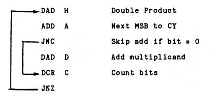
The product is developed from most significant position toward least significant, and instead of shifting the multiplicand we shift the product. The result is identical. This requires a bit counter, since the product must be shifted eight times, whereas the previous program can stop as soon as the multiplier reaches a value of zero. Figure 10-17 shows the process.
