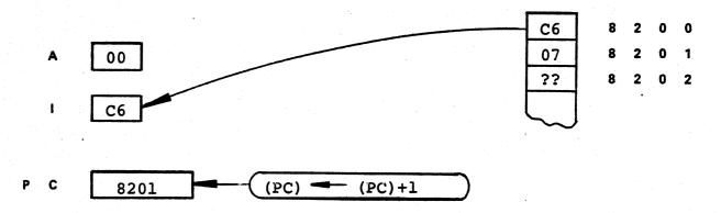
3) The logic is decoded, and the processor again sends the contents of (PC) to memory, selecting address 8201.
