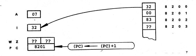
3) The instruction is decoded, and the processor sends the contents of (PC) to memory, selecting address 8201.
