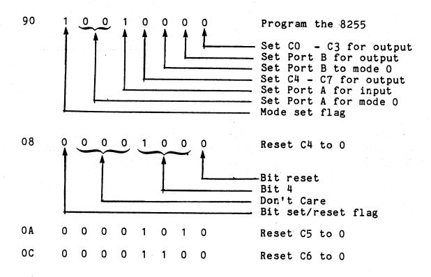
This provides a technique for altering one output bit without changing others. Another technique is to read the content of the output data latch:
