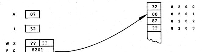
4) The memory sends the contents of 8201 to the Z register and (PC) is incremented by 1. Now Z contains the low order part of the address in which the contents of A will be stored. The design of the processor requires that the low order part of the address be stored immediately after the instruction code, followed by the high order portion.
