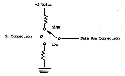
Clearly we could connect many such switches to a data bus line and if exactly one switch is high or low the line will be in a well defined state. The circuit used in the memory uses MOS transistors. If the high transistor is turned on, the circuit delivers current to the line from the 5 volt supply. If the low transistor is turned on, the circuit sinks current to ground. If both are off, the circuit exhibits a high impedance to the line.
