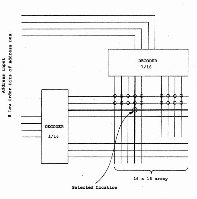
INTERNAL ADDRESS DECODING
