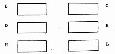
Their arrangement is like that of the W and Z registers, and for the same reason: a pair of eight bit registers is able to store a 16-bit memory address.
