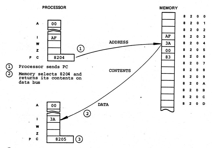
Processor loads data to I register and increments PC
