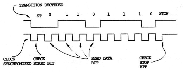
One half bit-time later the receiver checks the start bit. If it is not zero, an error has been made. Thereafter the receiver accepts eight bits, reading them at one bit-time intervals, then tests the stop bit to
