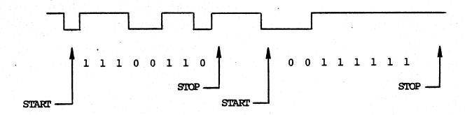
After some period of time with no data, (i.e. constant 'one' signals) the receiver will see a transition to zero. This signals the start of a character, and the receiver synchronizes its clock.
