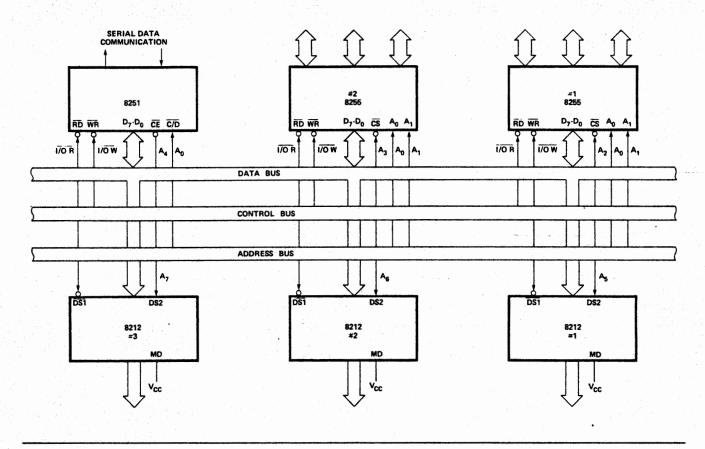
Figure 3-16. Typical I/O Interface.
