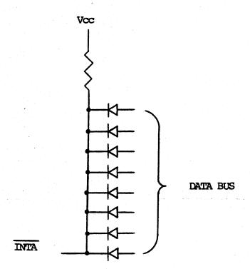
This scheme places all the capacitance of the diodes on the data bus at all times, so it must be used with care.
