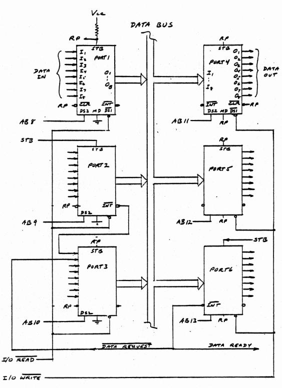
ARRAY OF INPUT /OUTPUT PORTS
