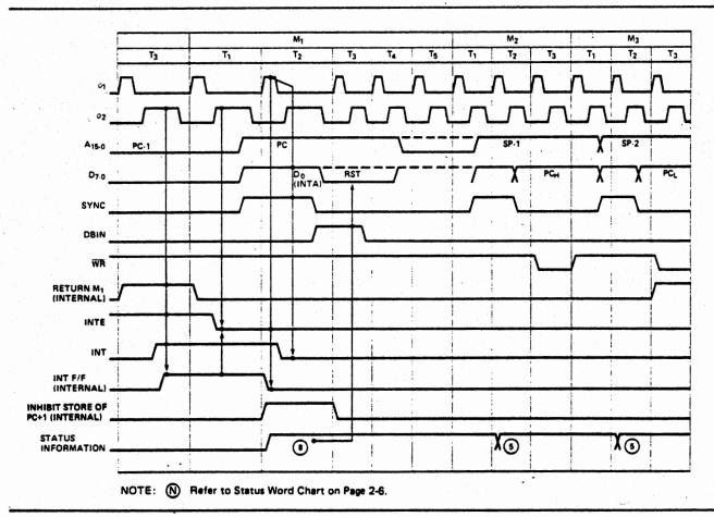
Figure 2-8. Interrupt Timing
