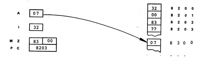
The execution of STA has required four machine cycles: an instruction fetch, two memory reads, and one memory write. Do not be confused by the fact that the high and low order parts of the address in this three-byte instruction (and all similar instructions) are reversed. The arrangement was adopted by the microprocessor's designers to simplify parts of the internal circuitry.
