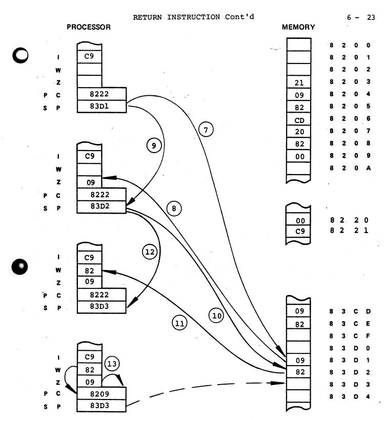
The stack pointer addresses the low byte of the return address which is loaded to Z (7,8). The stack pointer is incremented (9) and the high byte is loaded to W (10,11). The stack pointer is incremented again (12) and the program counter is loaded from W and Z.
