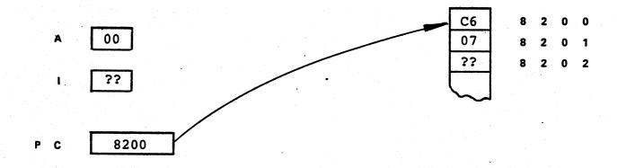
2) The memory sends the contents of address 8200 to the I register and (PC) is incremented by 1.
