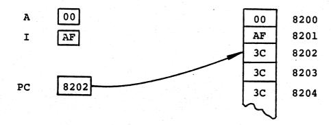
2) The memory sends the contents of address 8202 to the I register, and the (PC) is incremented.
