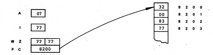
2) The memory sends the contents of 8200 to the I register and (PC) is incremented by 1.
