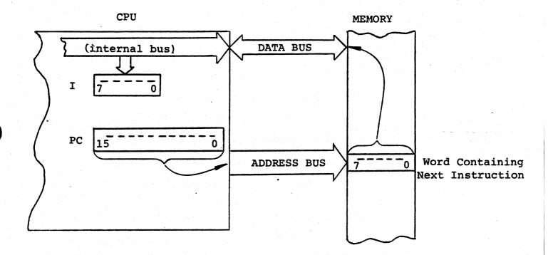
After the instruction has been loaded in I it is fed to the <u>instruction</u> decoder. The instruction decoder works much like the address decoder described earlier, looking at a pattern of input binary signals and outputing a pattern of signals which will sequence and control all of the steps required to execute the instruction.
