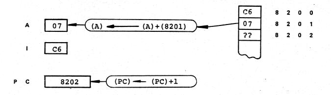
5) The instruction is completed. The memory has been accessed twice (two machine cycles), and (PC) has been incremented twice.
