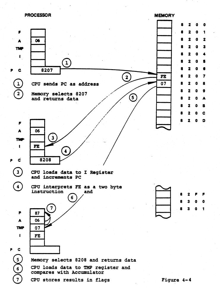
For all of the arithmetic and logical instructions that operate on data in the A register and one general purpose register, there are corresponding immediate instructions. These may be thought of as referring to a phantom register, created just to provide a desired data byte.
