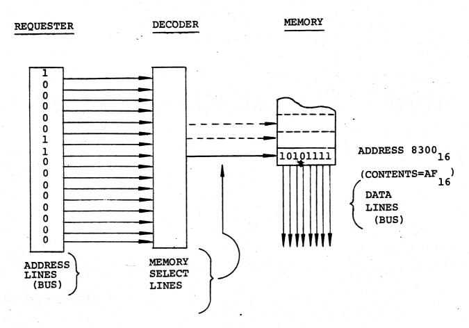
The memory select lines are essentially internal to the memory itself. The address lines and data lines serve as the communication channels between the CPU and its memories and I/O devices, and they have special names: address bus and data bus.
