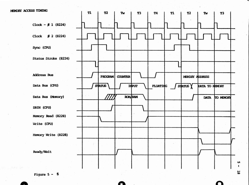
The clock generator receives the SYNC signal and generates a status strobe in response: this is a narrow pulse which the system controller uses to latch the status data.
