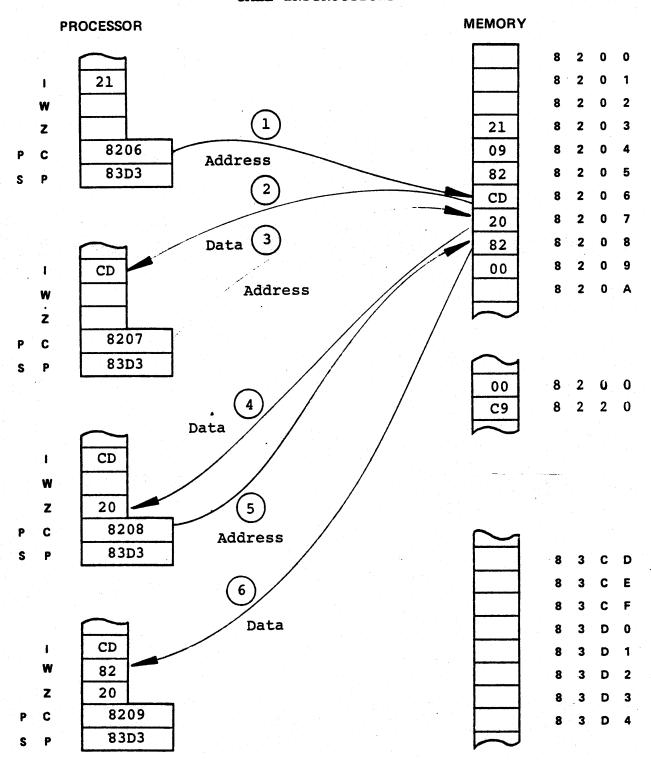
As in a jump instruction, the PC is used to address the instruction code and the two following bytes, which are loaded into I, Z and W respectively  $\Gamma$
