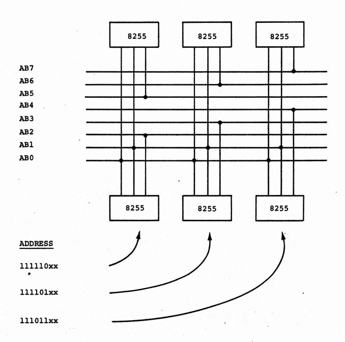
MULTIPLE I/O PORTS ON ADDRESS BUS Figure 8-4
