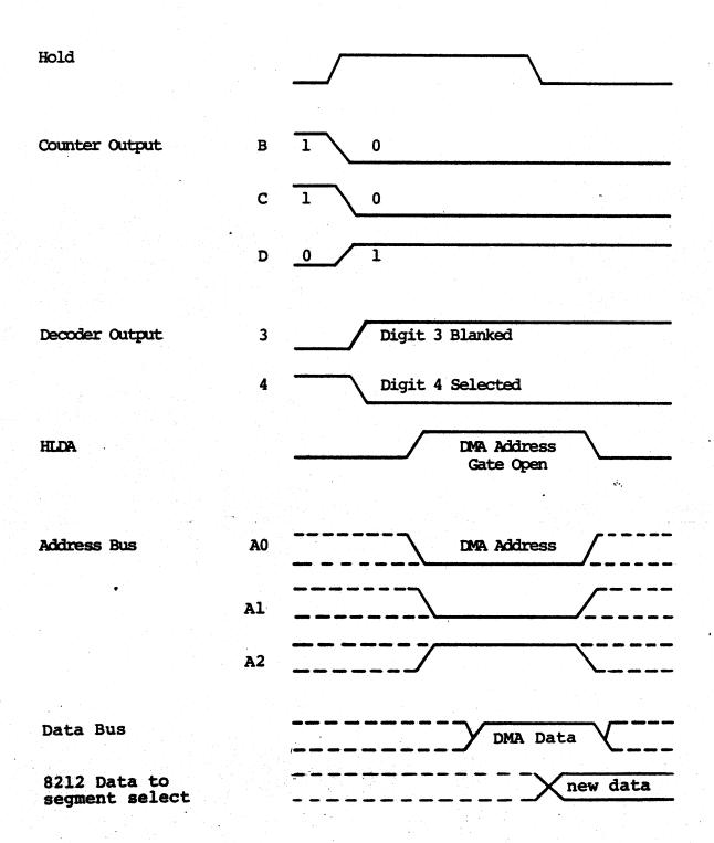
DMA TIMING IN MTS Figure 8-18
