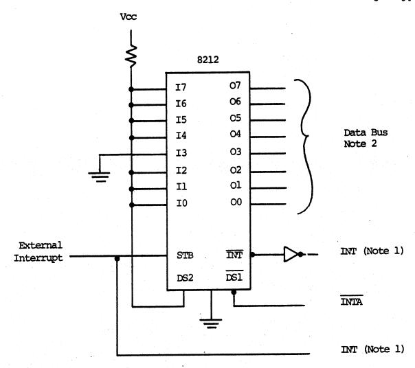
Note 1: If the external interrupt is a continuous signal it should provide the interrupt to the 8080. If it is a pulse, the 8212 can store it and provide the interrupt request.
