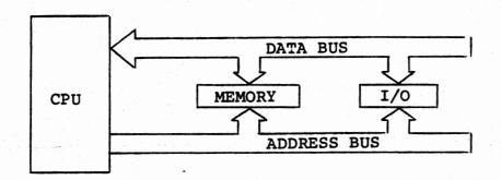
The CPU may send or receive data along the data bus (it is bidirectional), but no memory address is sent to the CPU along the address bus.
