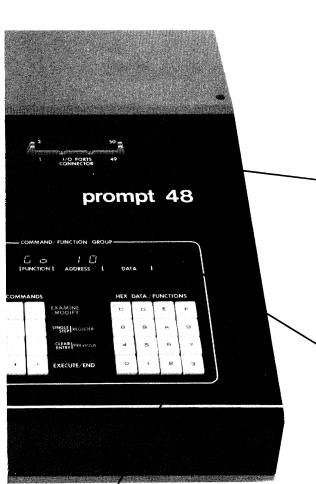
An optional cable, PROMPT-SER, directly connects the PROMPT system to virtually any terminal via a rear access slot. Another cable, PROMPT-SPP, allows programs and data to be downloaded from the Intellec Microcomputer Development System to the PROMPT system for debugging.
