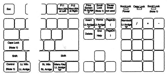
Note 1: Scroll Lock LED ON = PC Style: Caps Lock is Caps Lock and Left Control is Control Scroll Lock LED OFF = Amiga Style: Caps Lock is Control and Left Control is Caps Lock RESET: Control + Left Amiga + Right Amiga resets Amiga and flashes LED's
