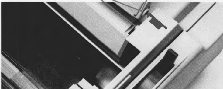
Brace holds support upright for single sheets.
