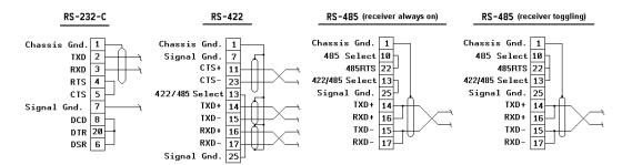
**Important** To select RS-422 communications, you MUST tie pin 13 to pin 25. To select RS-485 communications, you MUST either tie pin 13 to pin 25 and pin 10 to pin 22, or tie pins 10, 13, and 22 together. Be careful not to connect any wires to unused connector pins.
