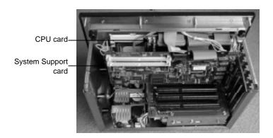
To add or replace DRAM you must remove the System Support card. Follow these steps to remove the System Support card.
