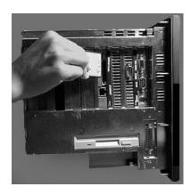
3. When you are ready, reinstall the CF card by carefully inserting the card into the slot and pushing it into the slot until the card is securely seated.
