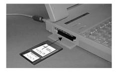
The computer should recognize and configure the card as an ATA card, assigning an additional drive letter for the card (e.g., D)
