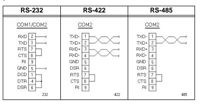
**Important** Be careful not to connect any wires to unused connector pins.
