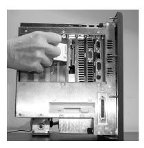
3. When you are ready, reinstall the CF card by carefully inserting the card into the slot and pushing it into the slot until the card is securely seated.
