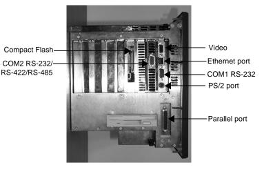
**Serial Ports** The PowerStation has two serial ports, COM1 and COM2, which you can use to communicate with external devices. These ports support baud rates of up to 115 Kbaud. The COM1 port supports the RS-232 communication standard. Use a standard DB9 connector for communicating with this port.
