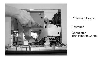
2. Disconnect the connector and move the connector and ribbon cable aside.
