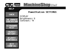
3. On the PowerStation Settings submenu, press the Calibrate Touchscrn button.
