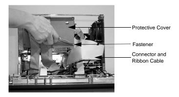
11. Remove the protective cover, carefully sliding it from beneath the remaining ribbon cables.
