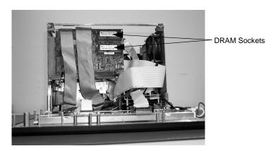
2. Push outward on the two clips holding the DRAM module in its socket as shown below. You may need to use a small screwdriver or the tip of a pen to push on the clips.
