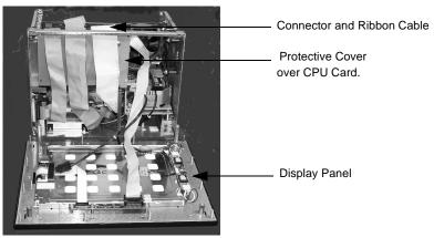
10. Use a pair of needle nose pliers to squeeze the fasteners that hold the protective cover to the CPU Board. See the illustration below.
