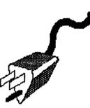
Figure 1 125V AC Attachment Plug Cap
