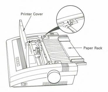
With the paper rack in a horizontal position, you can slide it forward or backward about 1/4 inch. Slide it forward to lock the printer cover and tear off the paper. Slide it backward to open the cover.
