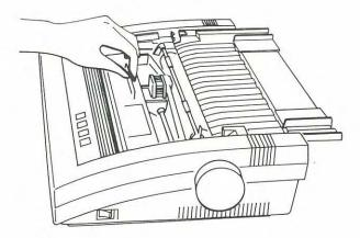
4. Unwrap the new ribbon cassette (Cat. No. 26-1236A) and tighten the ribbon by turning the ribbon feed knob in the direction shown by the arrow.
