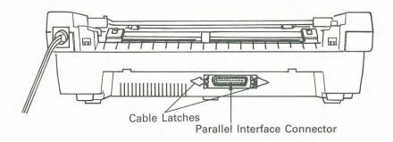
Be sure that you have the correct cable for connecting the computer to your printer. The following table lists the printer cables that Radio Shack carries. See your computer manual for connection locations on the computer.
