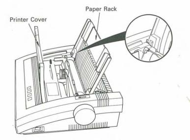
For fanfold paper: Install the paper rack as described for single-sheet paper. Then, pull the rack up along the slanted grooves and place the paper rack in its horizontal position, as shown below.
