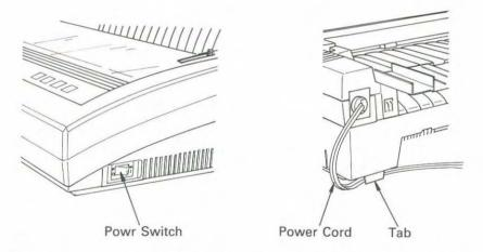
The power switch is on the right side of the printer. To turn on the printer, set the power switch to ON/1. To turn off the printer, set the power switch to OFF/0. If the printer is on, the POWER indicator on the control panel lights. Note that turning the printer off during operation causes the loss of print data.
