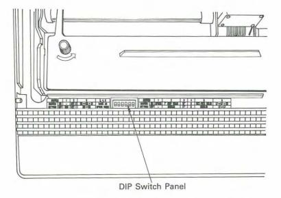
Furn off the printer and remove the printer cover. Set the DIP switches with the tip of a ball-point pen. To select IBM codes, set Switch 1 to OFF pefore turning on the printer. To select Epson codes, set Switch 1 to ON. For specific switch functions in each of these modes, refer to the two ables on the next page.
