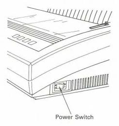
Set the power switch to OFF/0 to turn off the printer.
