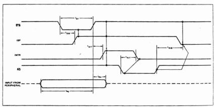
Figure 9. MODE 1 (Strobed Input)
