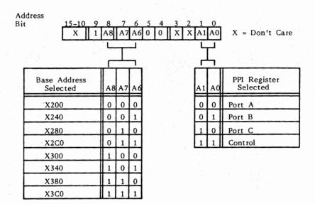
Fig. 2-2 DG24 I/O Port Address Decode
