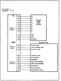
Figure 25. Machine Tool Controller Interface
