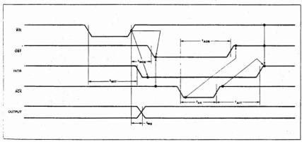
Figure 11. Mode 1 (Strobed Output)
