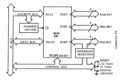
Fig. 3-1 DG24 Block Diagram
