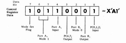
Note that PC 3,4, and 5 are used for the Port A handshaking and interrupt signals and are therefore not available for I/O ("8255A Operational Description", Figure 8); however PC 0,1,2,6, and 7 can be used for digital I/O. The interrupt signal generated on PC 3 may be jumpered to one of the the PC's interrupt channels. The interrupt channel selection was described in Chapter 2.
