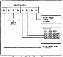
Figure 7. Bit Set/Reset Format
