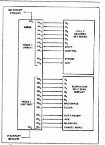
Figure 20. Keyboard and Display Interface
