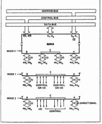
Figure 5. Basic Mode Definitions and Bus Interface
