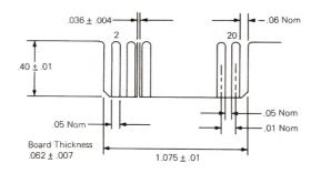
FIGURE 4 J3 Connector – Power
