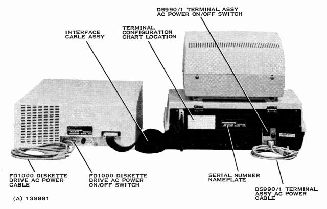
Figure 1-8. Rear View of DS990/1 System
