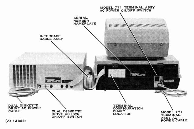
Figure 1-2. Rear View of Model 771 Intelligent Terminal System
