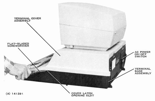
Figure 1-3. Terminal Cover Assembly Release
