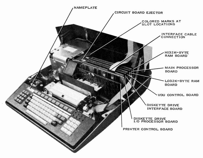
Figure 1-4. Internal View of Terminal Assembly
