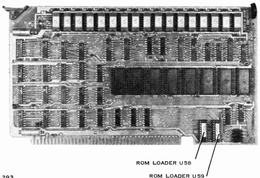
Figure 1-5. HI 32K-Byte RAM Circuit Board
