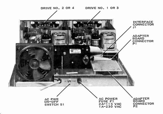
Figure 1-18. FD1000 Assembly Internal Rear View
