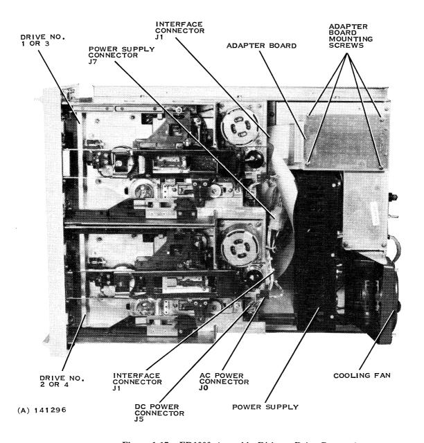
Figure 1-17. FD1000 Assembly Diskette Drive Removal
