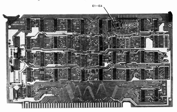
Figure 1-7. Diskette Drive Interface Circuit Board
