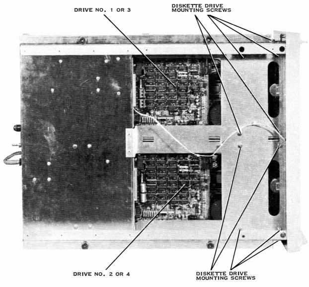
Figure 1-16. FD1000 Assembly Internal Top View
