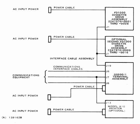
Figure 1-13. Typical Connection Diagram for the DS990/1 System With Two FD1000 Assemblies
