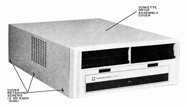
Figure 1-14. FD1000 Assembly Cover Removal
