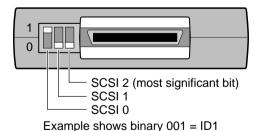
Figure 6-2 The SCSI ID Switch (Series 2 Drives only)
