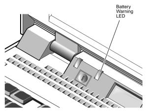
Figure 4-2 The Battery Warning LED
