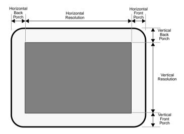
Figure 11-7 Video Timing Parameters on the Displayed Image
