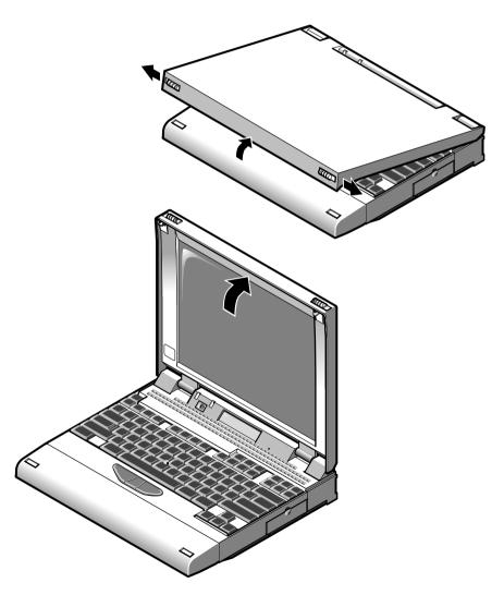
Figure 3-6 Adjusting the Display Viewing Angle
