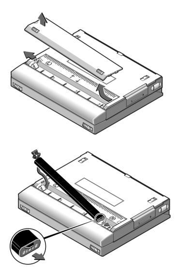
Figure 1-1 Installing the Battery (SPARCbook 3000 Shown)
