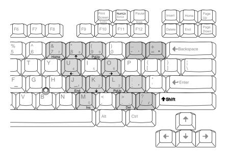
Figure 3-8 Numeric Keys with Shift Pressed
