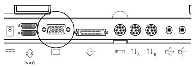
Figure 11-3 Display Interface Connector
