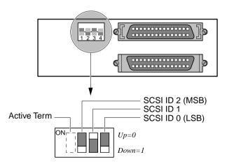
Figure 7-3 SCSI Floppy Disk Drive DIP Switches
