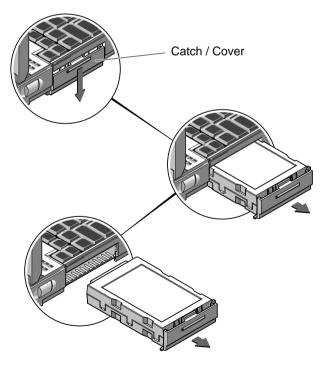
Figure 6-1 Removing the Hard Disk
