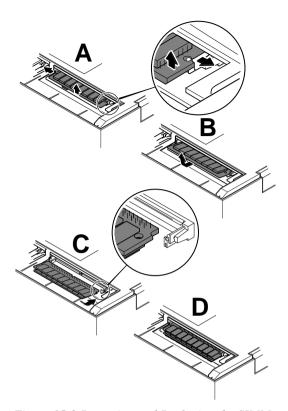
Figure 15-2 Removing and Replacing the SIMMs
