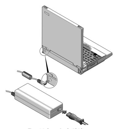
Figure 1-2 Connecting the AC Adapter
