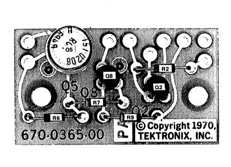
Fig. 4-2. Lampdrive Circuit Board.
