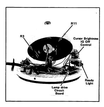
Fig. 4-1. Component location in the Joystick.
