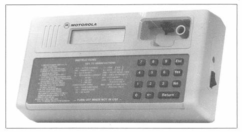
MOTOROLA'S BRAVO Numeric Display Portable Programmer lets you program and reprogram all codes, addresses and options on BRAVO Numeric Display pagers. Just remove the battery door and battery from the pager, put the pager in the Programmer, and select your options. You can program or reprogram BRAVO Numeric Display pagers anywhere in minutes!
