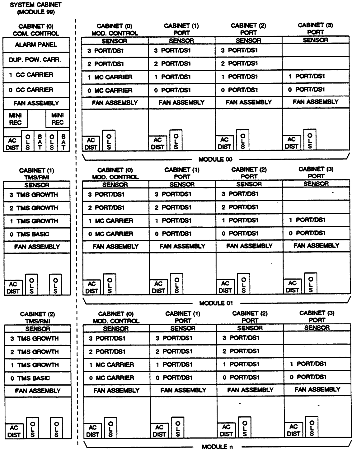
Figure 3-24. Typical Module/Cabinet/Carrier Layout for Critical Reliability Configuration
