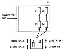
20.19.2 The following table shows the switch package associated with each port circuit. A switch section is fully depressed at the upper (U) end to provide the *RC NTWK* option and the *HI GAIN* (U) option. The switch section fully depressed to the lower (D) end provides the *600 OHM* option and the *LO GAIN* (D) option.
