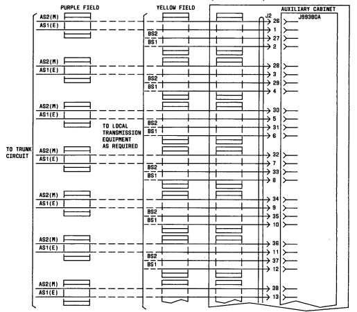
12.8.3 Connection from J2 connector to cross-connection field (Sheet 1 of 2)
