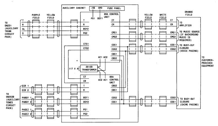
11.3.6 89A control unit connection - Loudspeaker Paging and Chime Paging features (See Part 9, paragraph 9.2.9 for circuit pack terminations and connections.)
