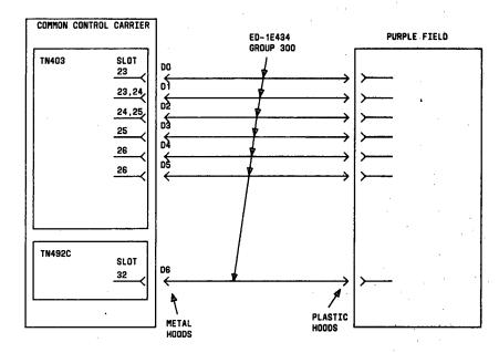
9.3.5 Connectors, slots, and cables for TN403 data channel circuit packs and TN492C alarm interface circuit pack for duplicated common control
