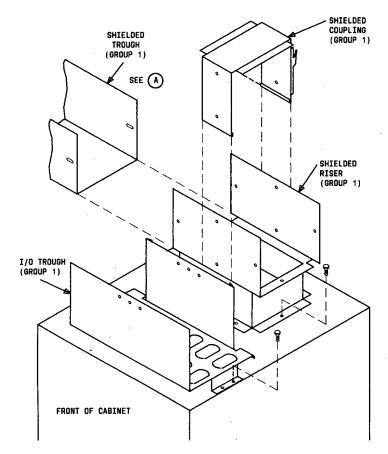
Figure 5.3 — Installation of Basic Duct Work for One Cabinet (Group 1)
