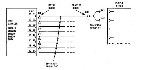
9.3.2 Connectors, slots, and cables for SN221B, SN222B, SN228, SN229, and SN241 circuit packs located in port carriers
