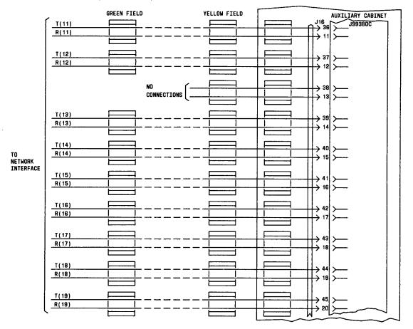
12.10.2 Connections between J16 connector and cross-connect field (Sheet 3 of 3)
