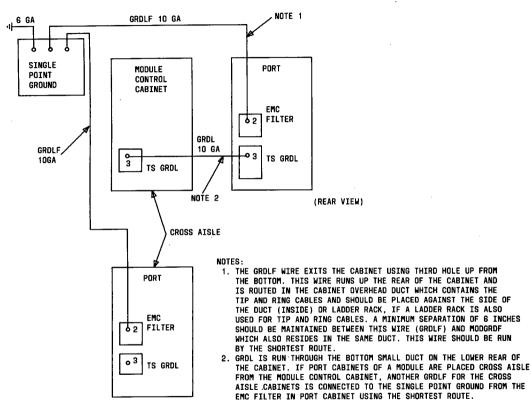
7.6.8 Lightning ground (GRDL) connections for cabinet equipped with port carriers
