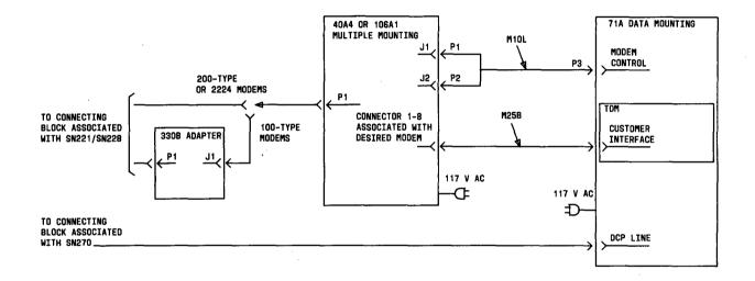
13.5.3.3.2.3 Connections using 201CR and/or 208BR modems (See Part 9, paragraph 9.2.9 for circuit pack terminations and cross-connections.)
