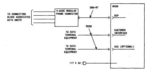
13.5.2.3.5 MPDM connections (multiple-mount application) (See Part 9, paragraph 9.2.9 for circuit pack connection and terminations.)
