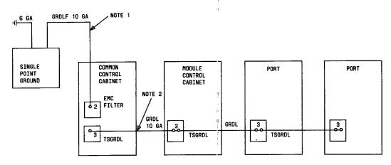
7.6.5 Typical lightning ground connections - unduplicated common control, single module, cabinets all on same aisle
