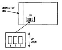
14.2.2.5.2.2 Set the option switches based on the length of the DS-1 cable between the cabinet and the DS-1
