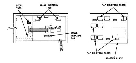
13.5.5.3.7 Connect the line cord to digital voice terminal, connect the handset if required, then attach the configuration to a wall mounting or to a stand for desk mounting.
