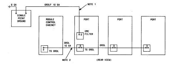
7.6.4 Typical lightning ground connections - duplicated common control, single module, all cabinets on same aisle
