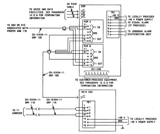
12.5.7 Attaching 15-pin or 25-pair connector to ED-1E434-11 GRP 357.
