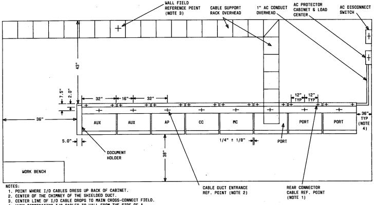
4. WHEN TERMINATING I/O CABLES TO WALL FROM THE SIDE OF A CABINET SPACE FROM CABINET TO WALL MUST BE 43 INCHES.
