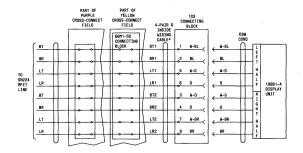
\* TYPE 286A (0.51 MM OR 24-GAUGE) CABLE IS EQUIVALENT. TYPE 285A (0.64 MM OR 22-GAUGE) Required if only one port (display unit half) is connected and run exceeds 210 m (700 FEET).
