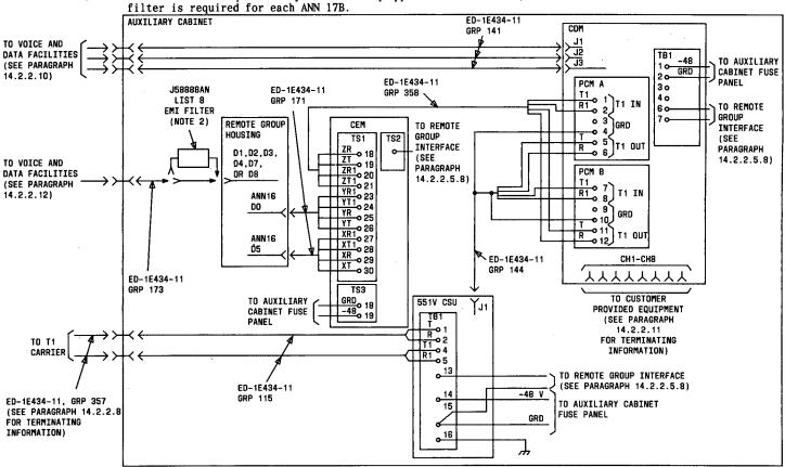
NOTE 1: The power, grounding and alarm leads are covered elsewhere in this part. NOTE 2: This filter is required only if RGH is equipped with an ANN 17B, but a filter is required for each ANN 17B.
