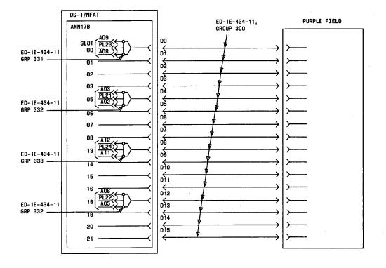
9.3.8 Connections, slots and cables for ANN 11B DS-1 trunk port located in DS-1/MFAT carrier
