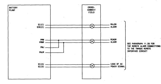
8.6.2 Alarm arrangement for battery plant circuit breaker panels with individual circuit breaker alarm contacts.
