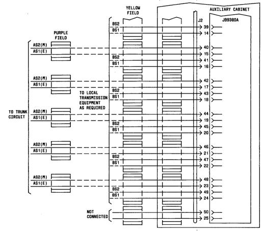
12.8.3 Connection from J2 connector to cross-connection field (Sheet 2 of 2)
