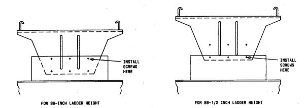
FIGURE 5.15 - Ladder Rack Supported 86 or 88-1/2 Inches From Floor (GRP 33)
