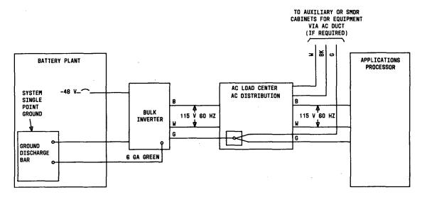
8.5.2 Extended power reserve ac distribution for auxiliary cabinet when bulk inverter does not provide required ac.
