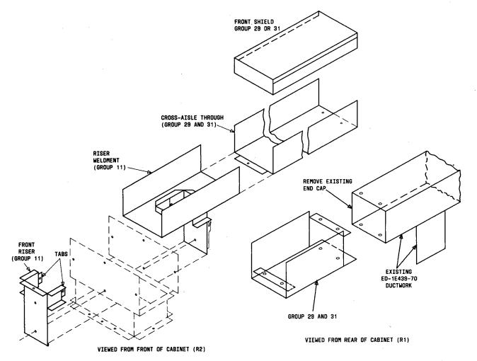
FIGURE 5.13 - Shield Transition Duct Work from System 85 (R2 or R3) to DIMENSION System 85 (R1)
