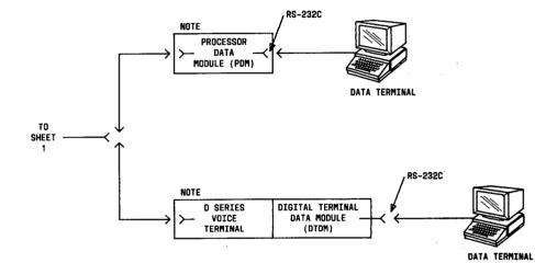
NOTE: CONNECTION INFORMATION FOR THE PDM AND DTDM IS IN PART 11.19 OF THIS MANUAL. 13.4.2 Data channel connection to switch (Sheet 1 of 2)
