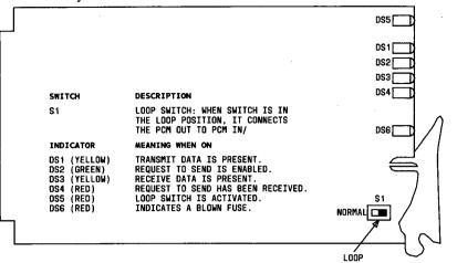
12.5.1.3.3.3 Switch locations and settings for 0 to 19.2 kbps asynchronous data channel unit
