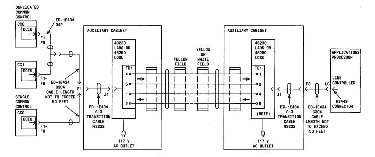
16.7 Applications Processor to System Connections Through DCIU and LADS/LDSU – Distance Greater than 100 Feet
