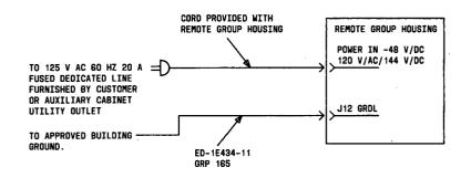
14.2.2.6.3 OLS with nominal holdover. This configuration can be used with or without an auxiliary cabinet. The remote group housing must have an OLS board (634WAAB) in slot 06.
