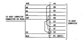
NOTE: Busy Out adapter must be used if pin 18 or 25 on the host computer is used to busy out a port.
