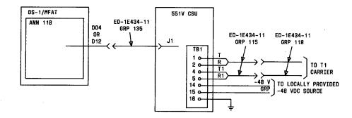
Part 12 Page 33 12.5.4 DS-1 trunk port to T1 carrier using CDM, CEM and 551V CSU
