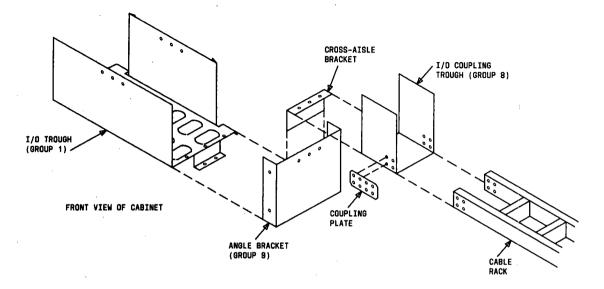
Figure 5.9 - Installing I/O Cable Rack Riser to End of Cabinet (Group 9)
