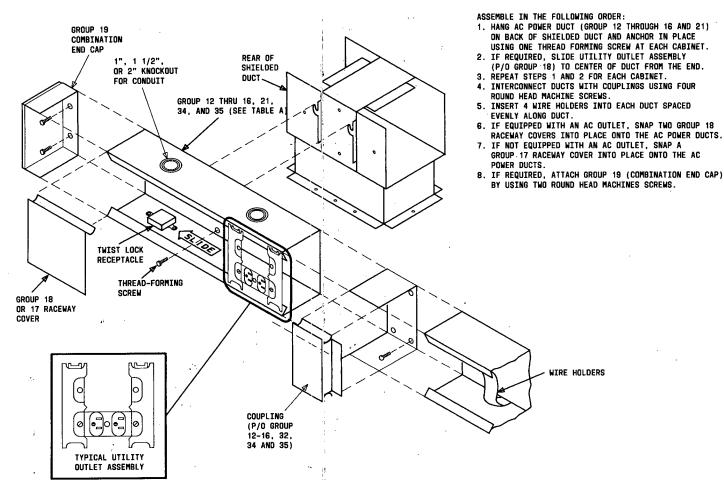
Figure 5.10 - Installing AC Power Duct
