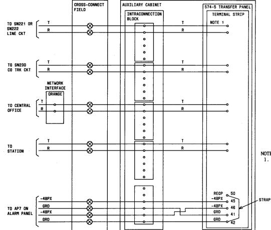
11.12.2.2 Power failure transfer connections showing one transfer voice terminal (station) and power connections mounted in auxiliary cabinet. (See Part 9, paragraph 9.2.9 for circuit pack terminations and connections.)
