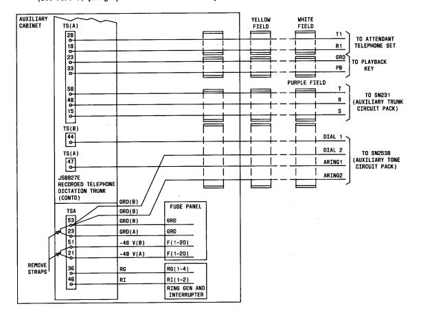
11.14.4 Dictation trunk - telset, playback key, ringing generator, and fuse panel connections (See Part 9, paragraph 9.2.9 for the circuit pack terminations and connections.)
