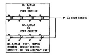
22.1.4 Lightning Ground (GRDL) Carrier Connections
