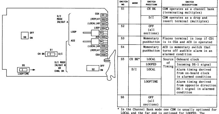
In the Channel Bank mode one CDM is usually optioned for LOCAL and the far end is optioned for LOOPED. The exception is when the DS-1 facility provides timing. In that case, both CDMs are optioned for LOOPED.
