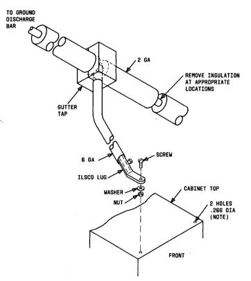
NOTE: EITHER HOLE ON CABINET TOP MAY BE USED TO CONNECT 1LSCO LUG.
