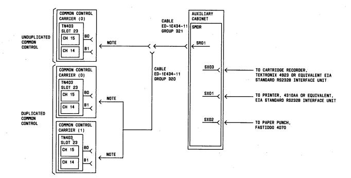
NOTE: Connect to appropriate connector (B0 or B1). Appropriate connector can be determined from CSD. 11.17.3 Interface to NCOSS, CMDR, and CSMDR using LSUs
