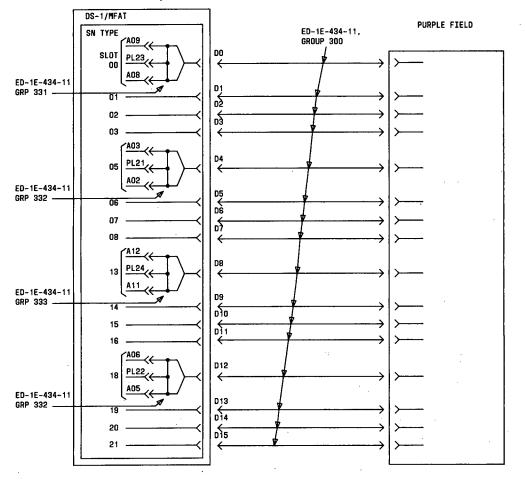
9.3.4 Connectors, slots, and cables for TN403 data channel circuit packs and TN492C alarm interface circuit pack for unduplicated common control
