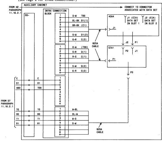
11.16.2.2 RMATS connection with data set in slot 1 or 2 (Sheet 1 of 2) (See Page 2 for cross-connections.)
