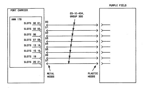
9.3.7 Connectors, slots, and cables for ANN 17B multifunctional analog terminal located in DS-1/MFAT carrier
