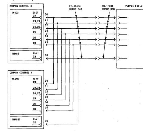
9.3.6 Connectors, slots, and cables for ANN 17B multifunctional analog terminal located in port carrier
