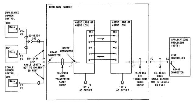
NOTE: FOR GROUND ISOLATION, THE LADS MUST BE PROVIDED IN THE DATA LINK, EVEN IF THE APPLICATION PROCESSOR CABINET IS IN THE SAME LINEUP WITH THE SWITCH CABINETS.
