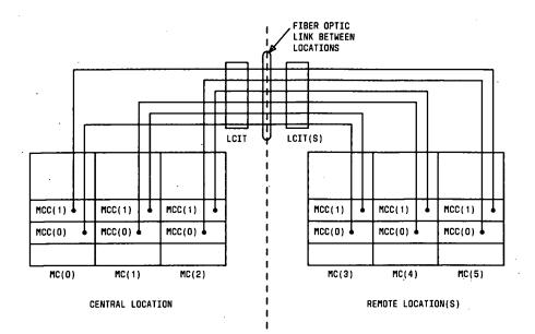
Figure 10. Assigned Module Control Carriers for a Duplicated System With Three Central and Three Remote Modules (Phase 1)
