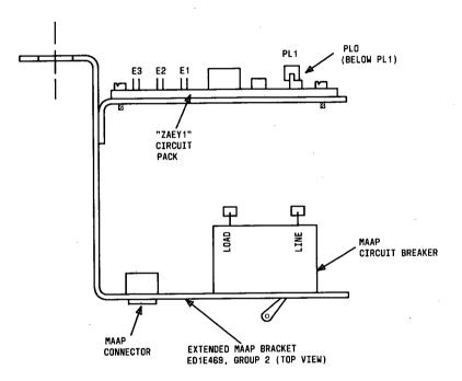
Figure 18. ED-1E469, Group 2 Remote Extended MAAP Bracket (Phases 1 and 2)
