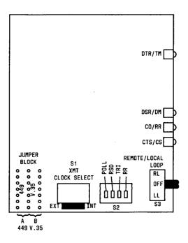
Figure 95. V.35/RS-449 Option Switch Locations
