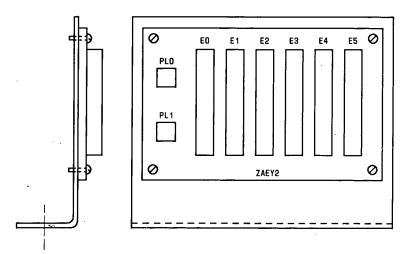
Figure 15. ED-1E469, Group 4 Central Extended MAAP Bracket (Phase 2)
