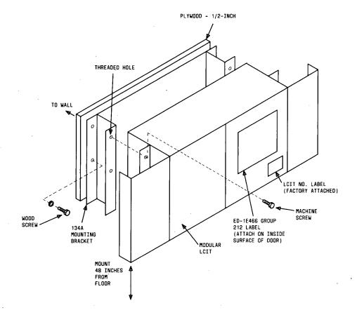
Figure 6. LCIT Installation on Wall
