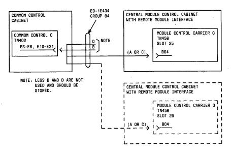
Figure 28. ED-1E434, Group 84 Connections for an All Unduplicated System (Phase 1)
