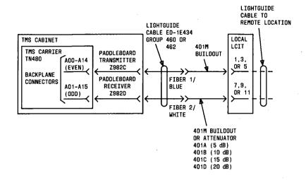
Figure 52. Central TMS Fiber-Link Connections for Unduplicated Module Control (Phases 1 and 2)
