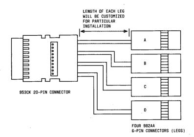
Figure 36. ED-1E434, Group 84 Coaxial Cable
