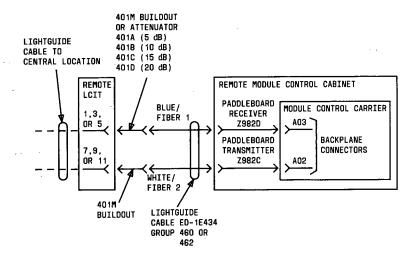
Figure 56. Remote TMS Fiber-Link Connections for Unduplicated Module Control (Phases 1 and 2)
