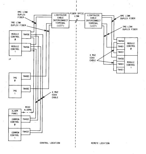
Figure 2. Duplicated RMI System (Phase 1) Block Diagram
