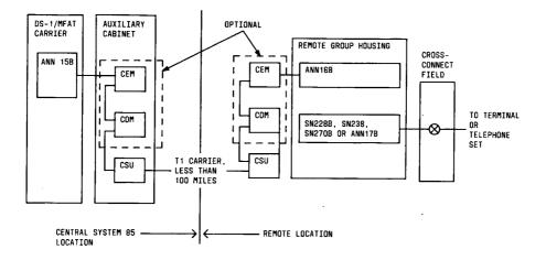
Figure 73. Remote Group Interface Block Diagram
