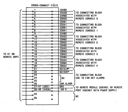
Figure 66. D1 Cross-Connect Connections
