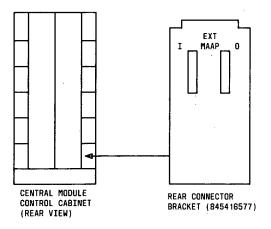
Figure 13. Rear Connector Plate (845416577) and Location (Phases 1 and 2)
