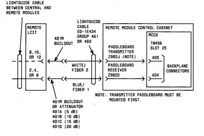
Figure 54. Remote RMI Fiber-Link Connections for Unduplicated Module Control (Phases 1 and 2)
