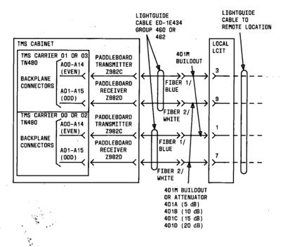
Figure 53. Central TMS Fiber-Link Connections for Duplicated Module Control (Phases 1 and 2)
