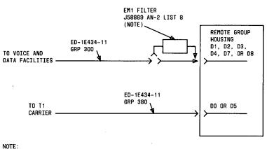
This filter is required only if RGH is equipped with ANN17B, but each connector associated with ANN17B requires a filter.
