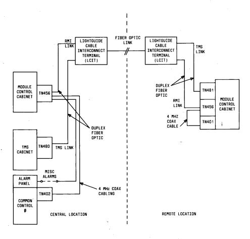
Figure 1. Unduplicated RMI System (Phase 1) Block Diagram
