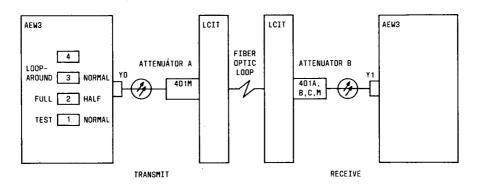
Figure 69. Circuit Pack AEW3 Switch Locations
