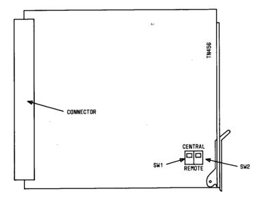
Figure 20. Option Switch Locations for TN456 Circuit Pack
