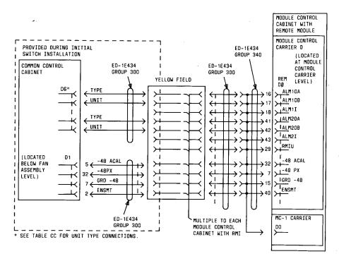
NOTE: FOR DUPLICATED SYSTEMS, AN ED-1E434 GROUP 340 CABLE IS USED TO "Y" MCO AND MC1 "DO" CONNECTORS TOGETHER, AND THEN CONNECTS TO THE GROUP CABLE.
