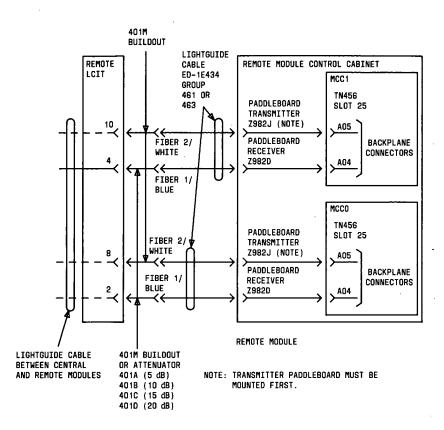
Figure 55. Remote RMI Fiber-Link Connections for Duplicated Module Control (Phases 1 and 2) Remote Location ED-1E434, Group 460 or 462 TMS Fiber Link(s) (Phases 1 and 2)
