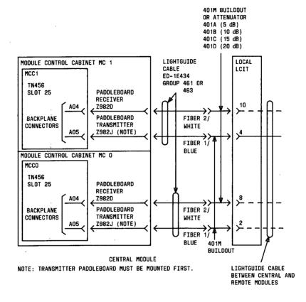
Figure 49. Central RMI Fiber-Link Connections for Duplicated Module Control (Phase 1)
