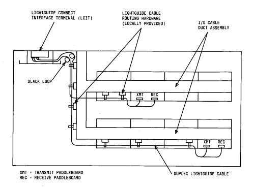
Figure 47. Routing of Lightguide Cables to LCIT
