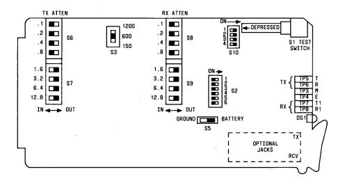
Figure 91. 30044-002 4-Wire E&M Channel Unit Switch Locations
