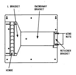
Figure 76. RGH Wall Mounting Bracket
