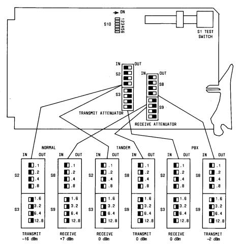
Figure 89. 30003-002 4-Wire E&M Channel Unit
