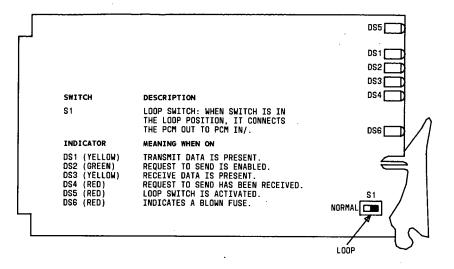
Figure 90. Asynchronous Data Channel Unit Switch Locations and Setting
