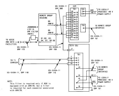
Figure 105. T1 Carrier to RGI Using CEM and CSU
