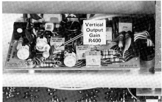
Fig. 5-15. Location of Vertical Output Gain adjustment.
