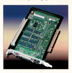
ator offers resolutions of 640-by-480 to 1,280-by-1,024 pixels and 8-, 16- or 32-bit color per pixel for Solaris 2.5.1/2.6-based systems. The EclipsePCI includes a built-in Sun 4/5 keyboard port, enabling multiple users to interface directly with the server without the addition of client workstation, and comes with either 2 or 4 MB of EDO DRAM.
